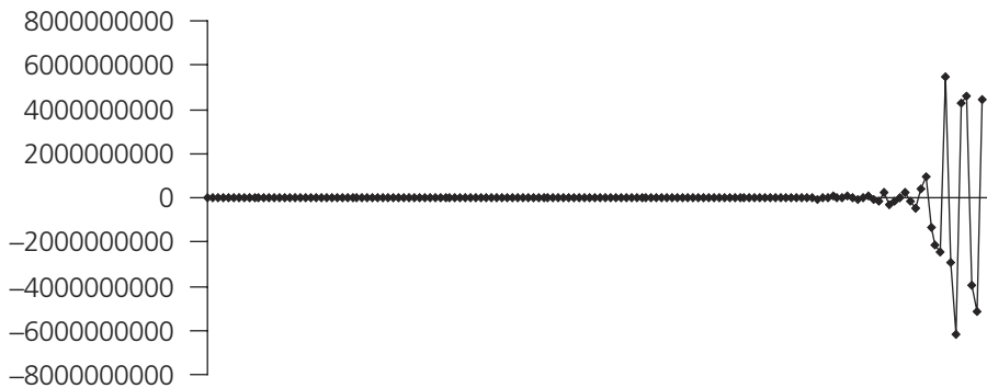
Figure 8.1 If the particle swarm algorithm is run without limiting velocity, the particle quickly explodes beyond the region of interest. (Note: Time runs from left to right for 150 iterations in the graphs in Figures 8.1 through 8.15.)
