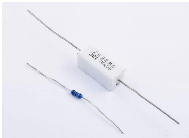
Figure 11 - Resistors designed for different power
