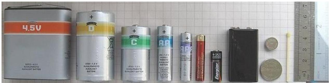
Figure 6 - Different galvanic cells
