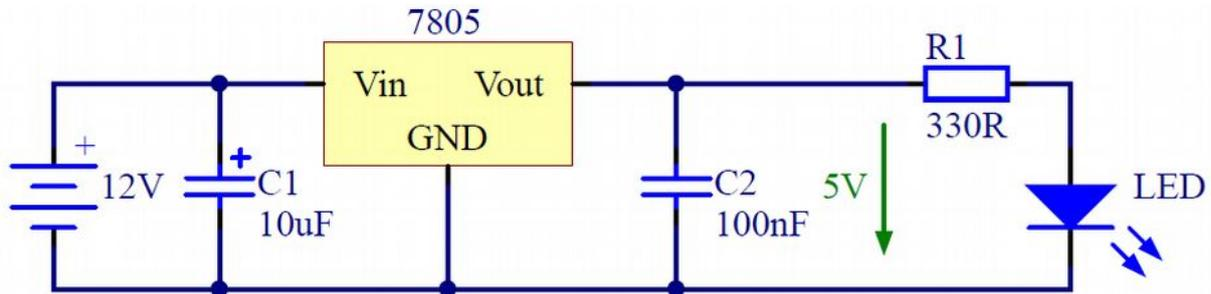
Figure 15 - 7805 power supply with an LED on its output
