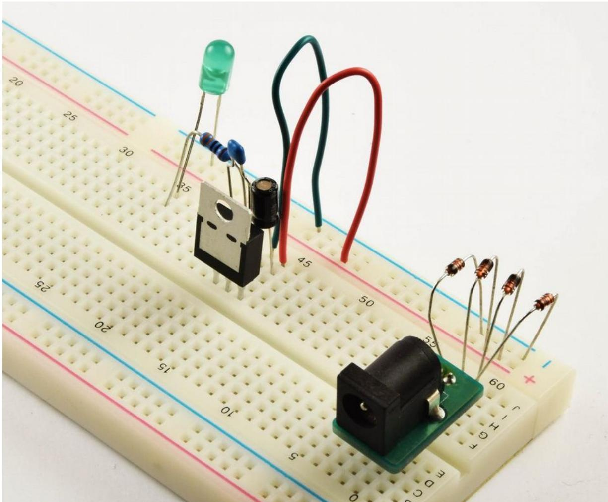
Figure 26 - Wiring breadboard with 4 diodes
