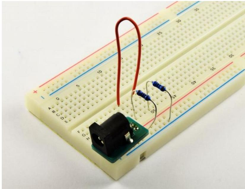
Figure 4 - Resistive divider implemented on Breadboard
