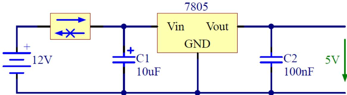
Figure 20 - Power supply with polarity protection
