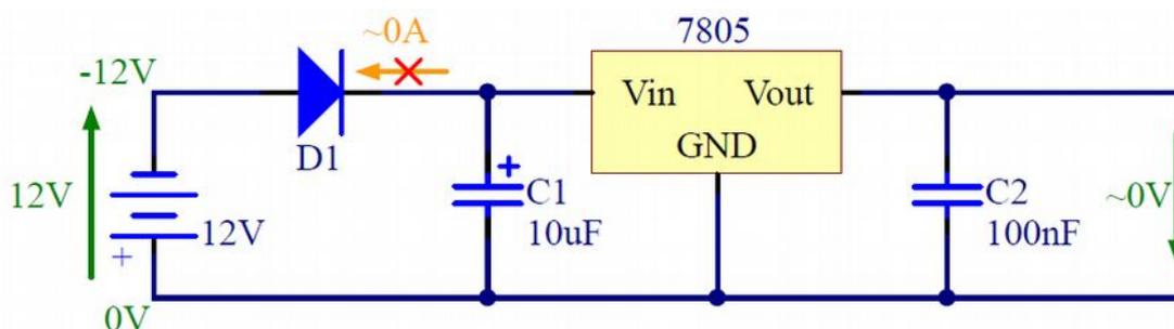
Figure 24 - Power supply protected against reverse polarity
