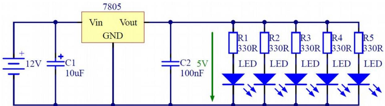
Figure 16 - 7805 power supply with five LEDs on its output
