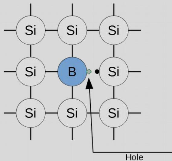
Figure 37 - Silicon in atom grid, polluted with boron
