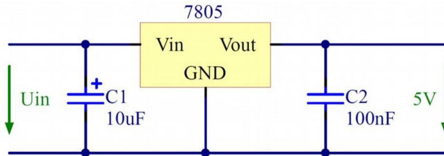
Figure 10 - Wiring of 7805 power supply
