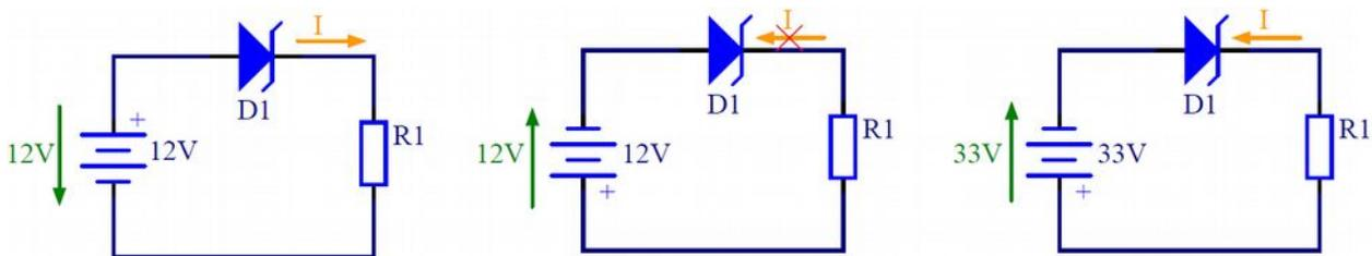
Figure 30 - Operation of Zener diode
