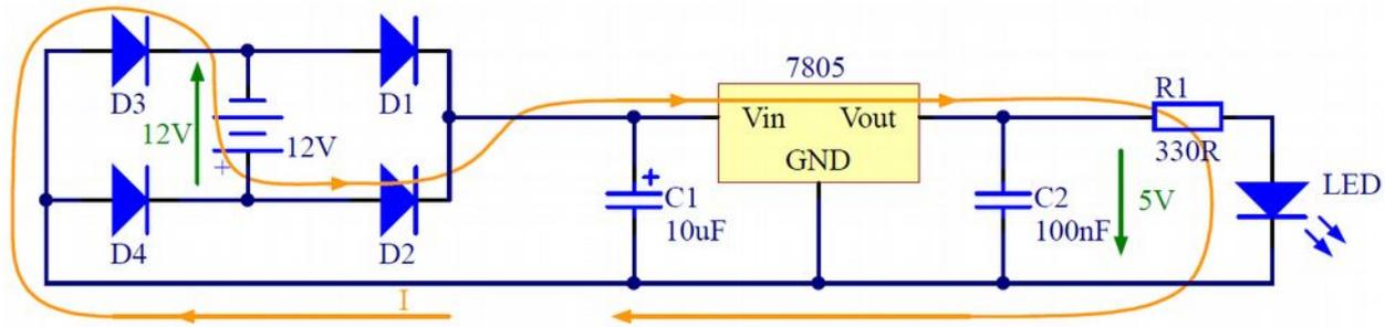
Figure 28 - Operation of polarity independent power supply with negative input
