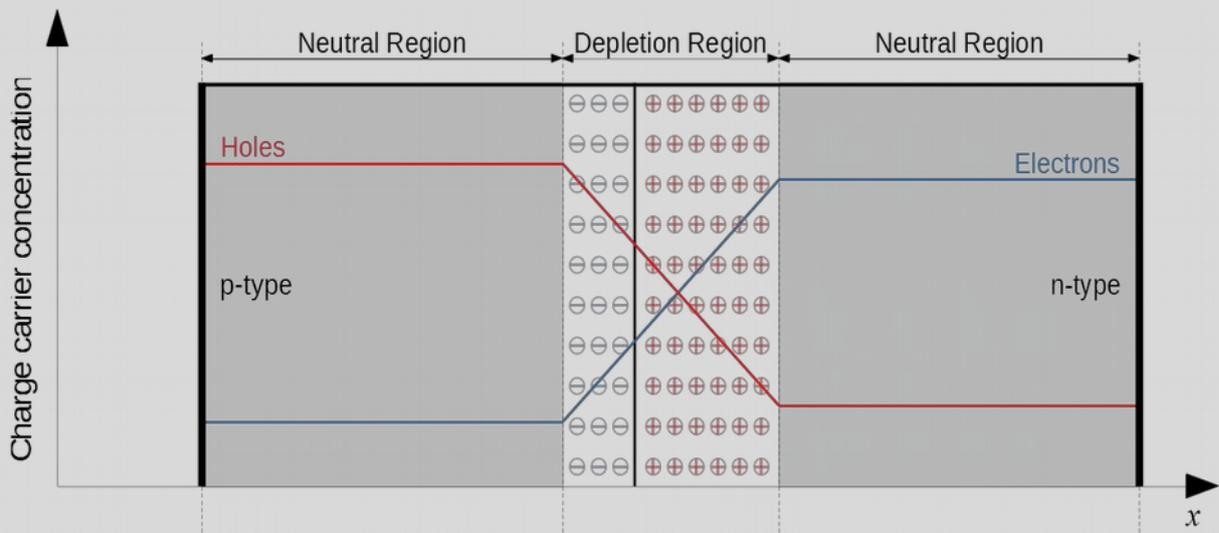
Figure 39 - Empty range of P-N junction
