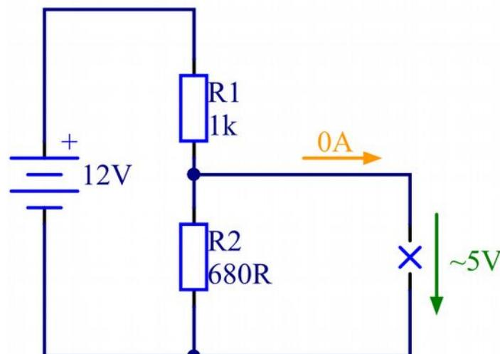
Figure 3 - Resistive divider
