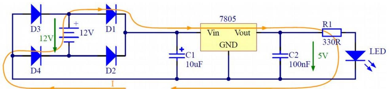
Figure 27 - Operation of polarity independent power supply with positive input
