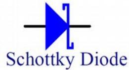
Figure 47 - Symbol of the Schottky diode
