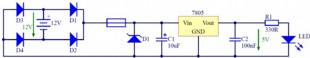
Figure 33 - Polarity independent power supply with overvoltage protection
