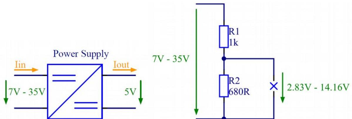
Figure 6 - Controlled power supply and the resistive divider with different voltages
