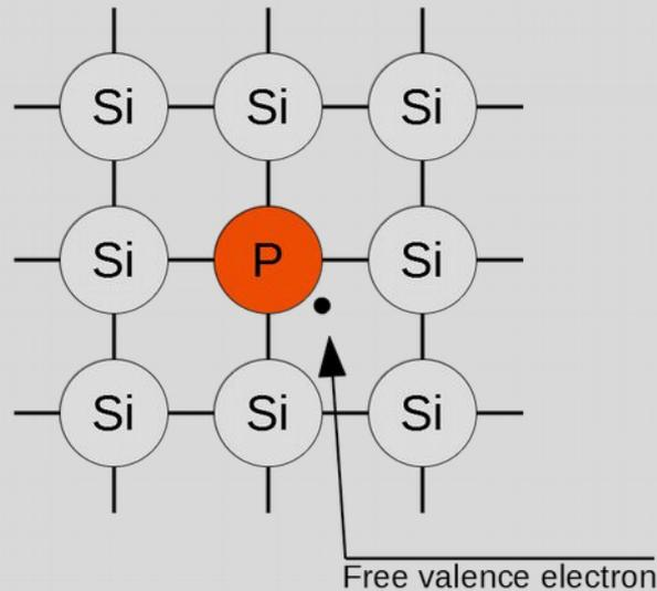
Figure 36 - Silicon in phosphorus polluted atom grid
