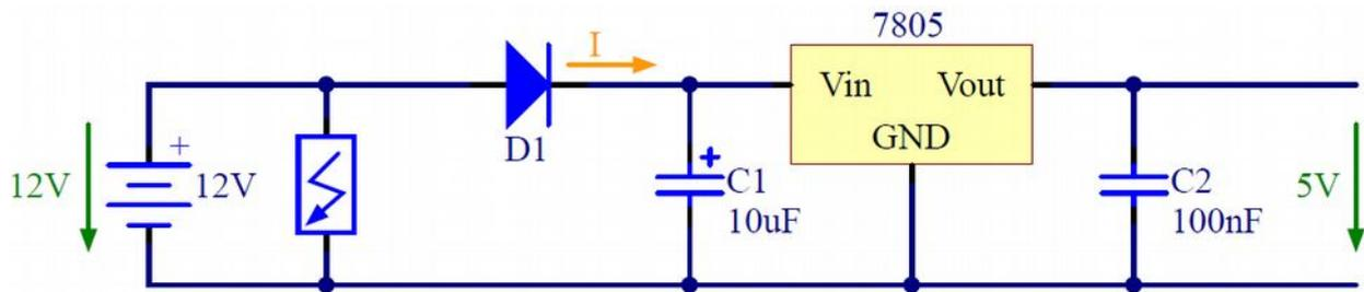
Figure 29 - Power supply with overvoltage protection
