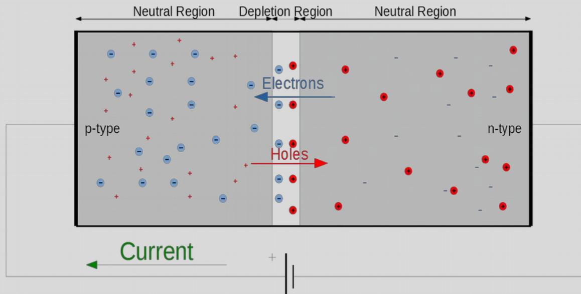
Figure 40 - Positively charged P-N junction, with reduced empty layer, current flows
