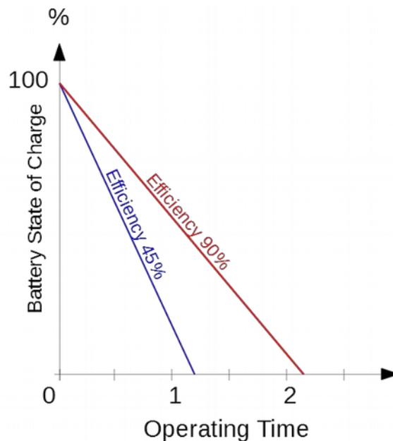
Figure 8 - Battery (12 V @ 1 Ah = 12 Wh), Power Supply 90% | 45%, Consumer (5 V @ 1 A = 5 W)
