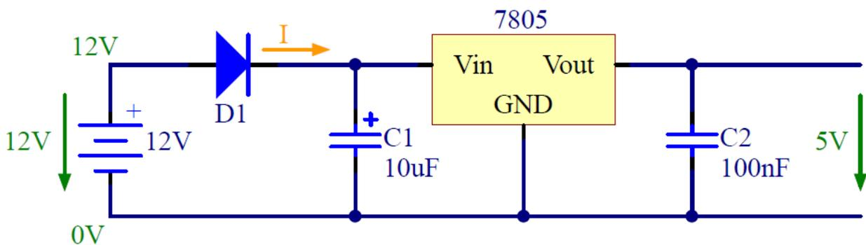
Figure 22 - Power supply with polarity protection, using a diode
