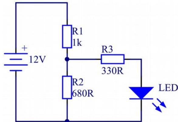
Figure 5 - Resistive divider, with an LED on its output
