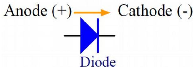
Figure 34 - Symbol of diode
