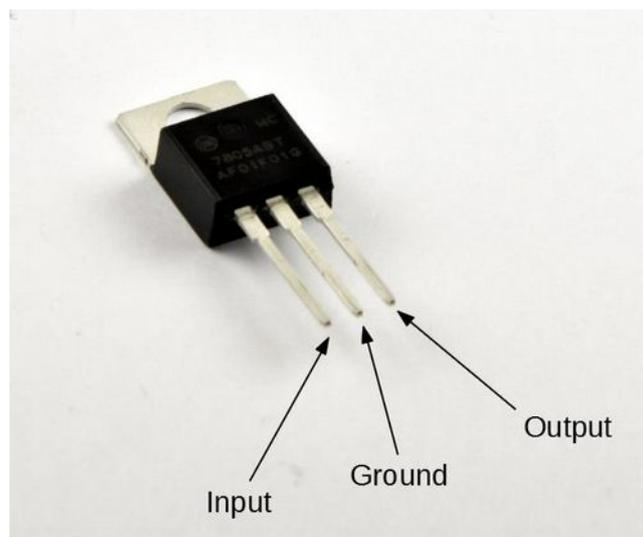
Figure 9 - The 7805 power supply
