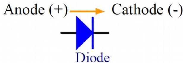
Figure 21 - Symbol of diode
