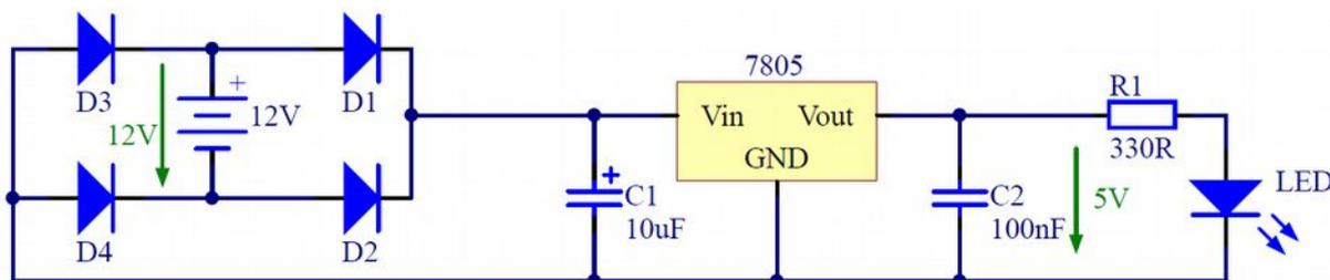
Figure 25 - Polarity independent power supply
