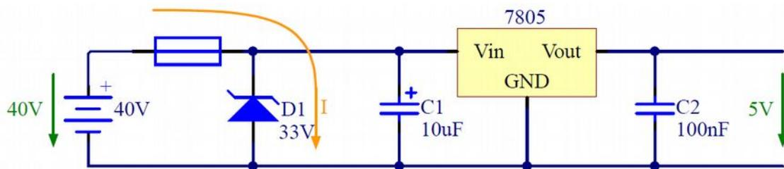
Figure 31 - Power supply protected against overvoltage
