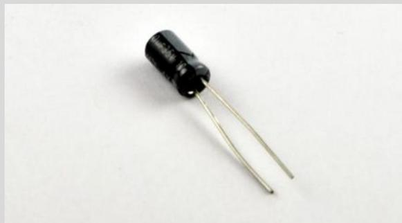
Figure 11 - 10  $\mu\text{F}$  capacitor
