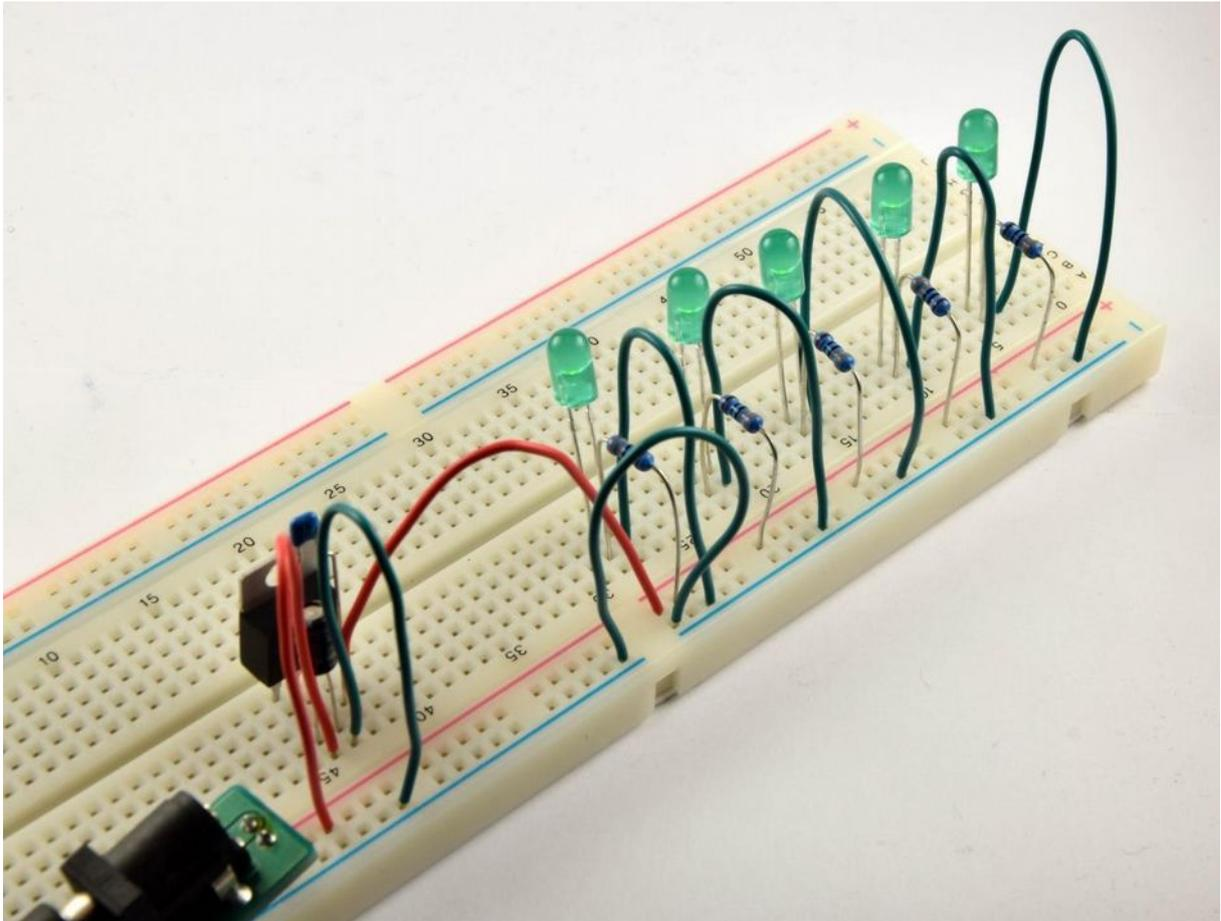
Figure 17 - 5 LED connected to the output, on breadboard
