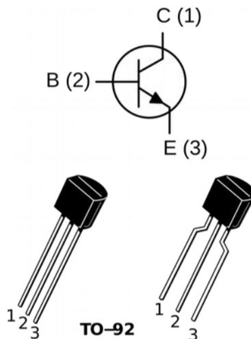
Figure 3 - BC546 transistor pin assignment
