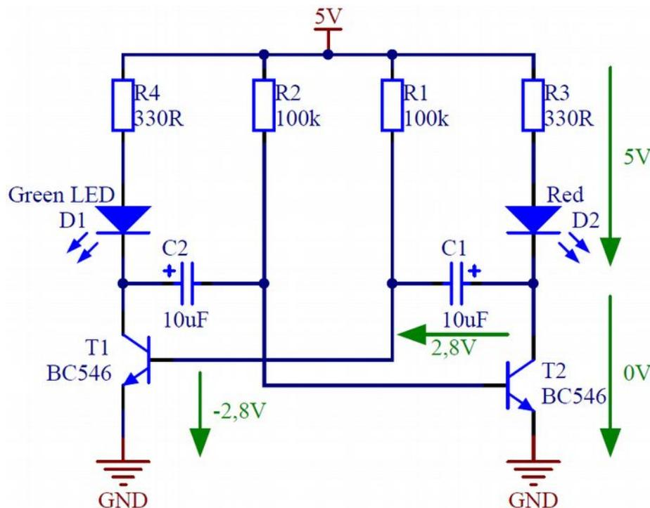
Figure 5 - Voltages immediately after opening T2
