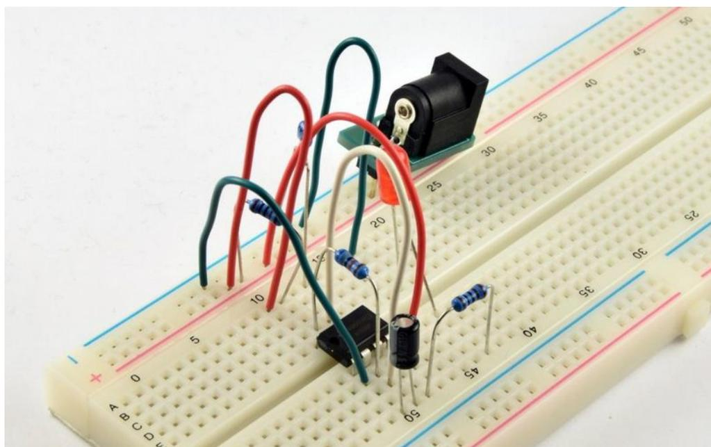
Figure 8 - Astable circuit with 555 IC on the breadboard
