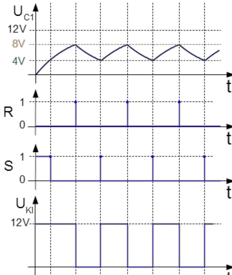
Figure 10 - Voltage measured on the capacitor C1 and the signals of the 555 IC
