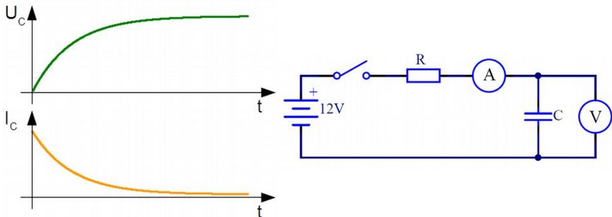
Figure 6 - Capacitor's voltage and current during charging
