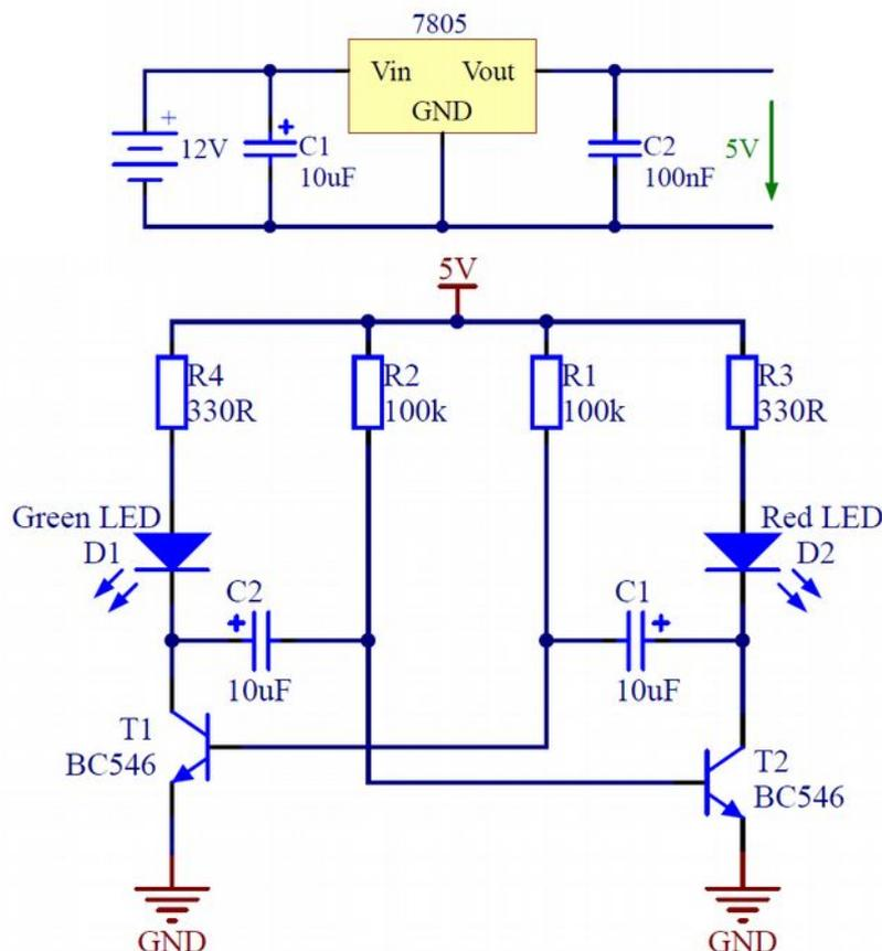
Figure 1 - 7805 voltage regulator and realization of astable circuit with transistors
