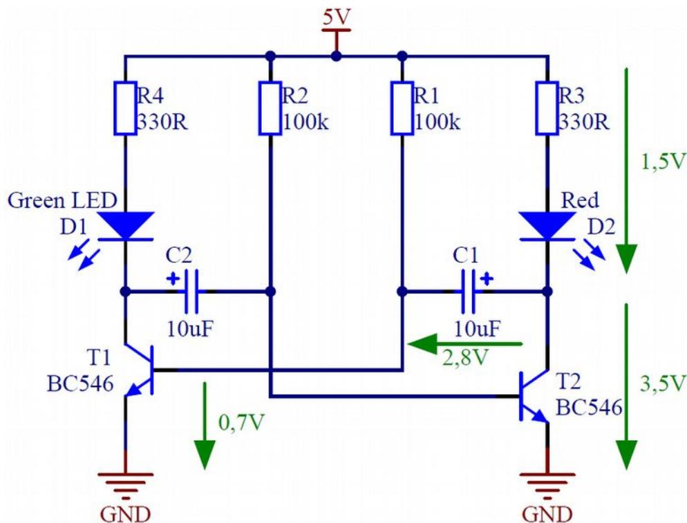
Figure 4 - Voltages, when T1 is open, and T2 is closed
