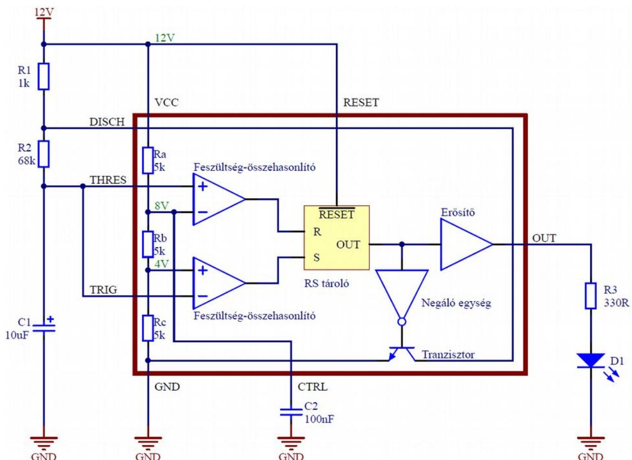
Figure 9 - Block diagram of the 555 IC in the astable circuit
