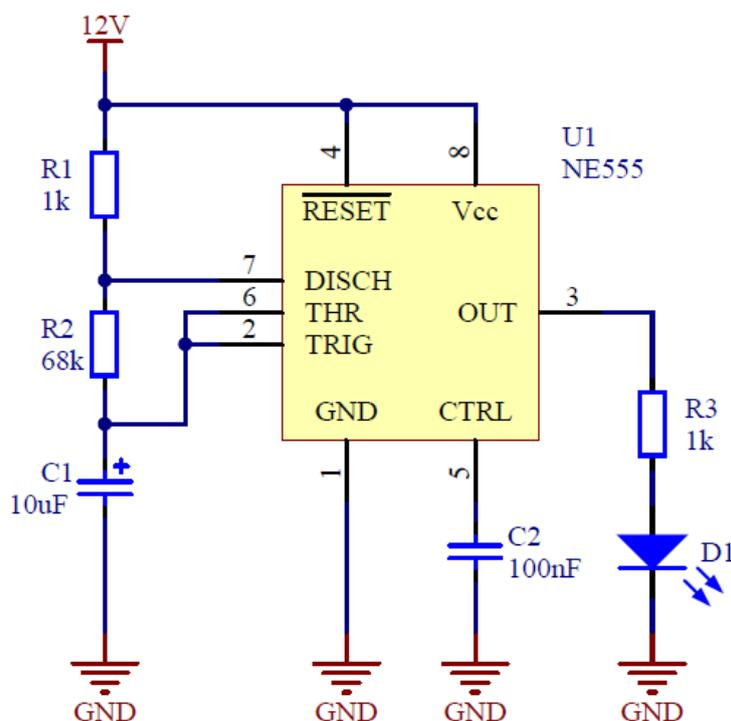
Figure 7 - Astable circuit with 555 IC
