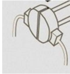
Figure 4 - Commutator
