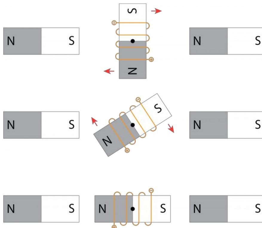
Figure 5 - Force on a magnet/coil
