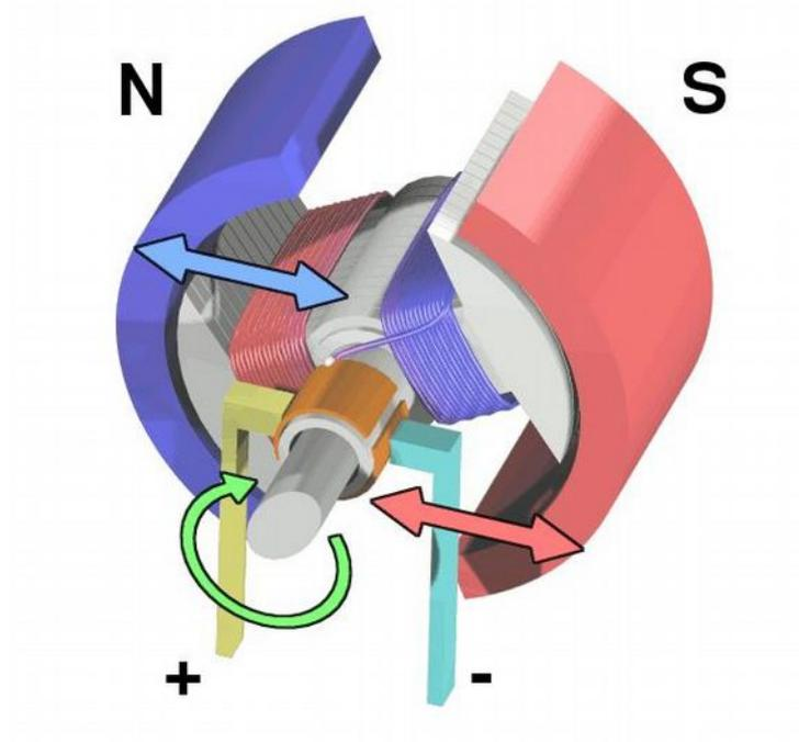
Figure 6 - with the commutator and voltage source. The figure is only for demonstration purposes, in case of this layout, the commutator would short circuit the source by turning
