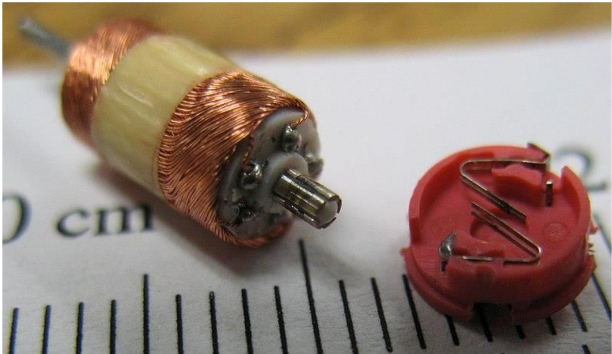
Figure 8 - Commutator
