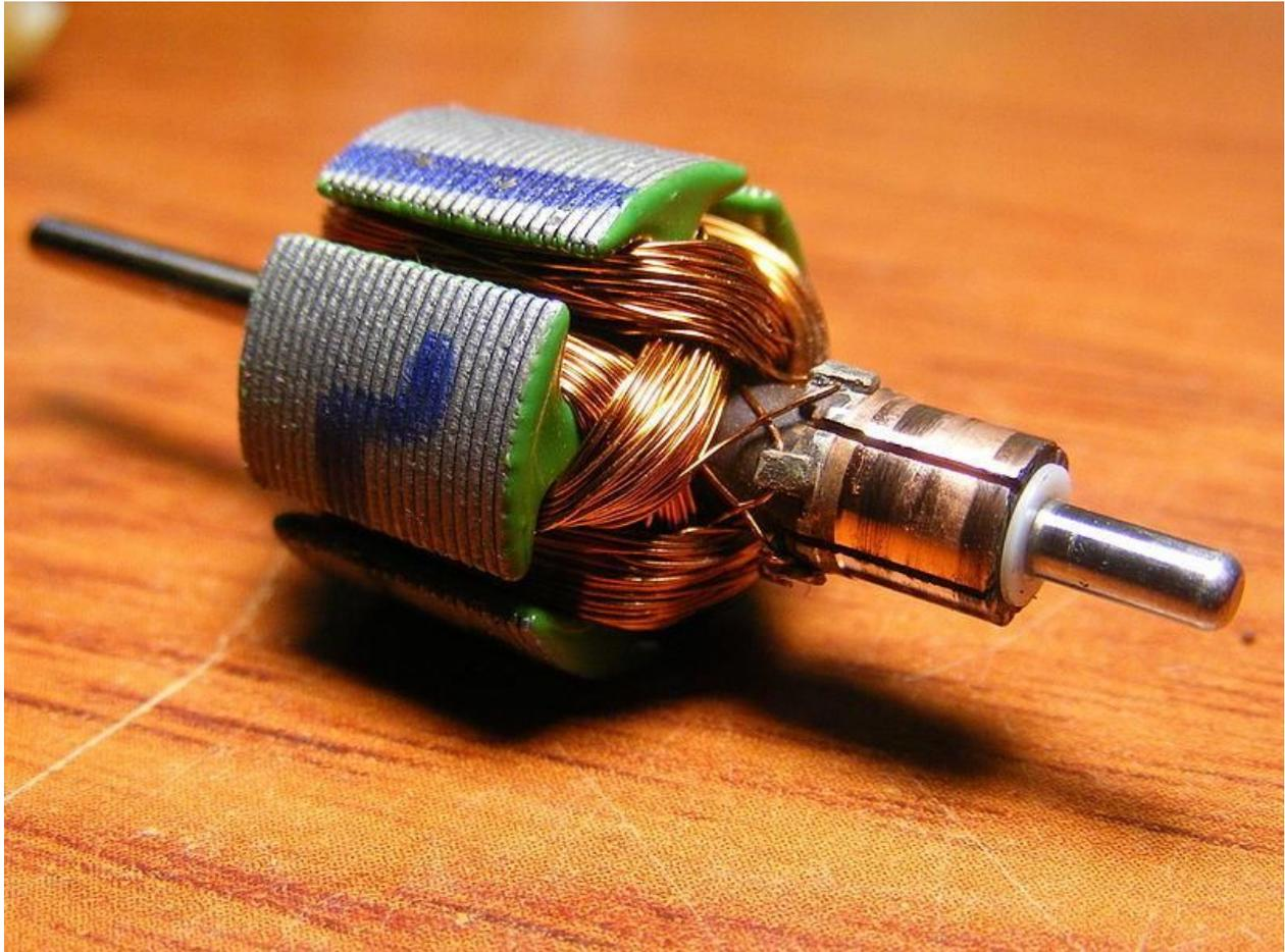
Figure 9 - Commutator
