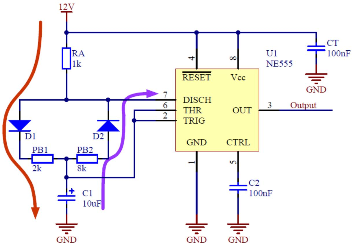
Figure 13 - The way of current when the capacitor  $C_1$  is charging, and discharging
