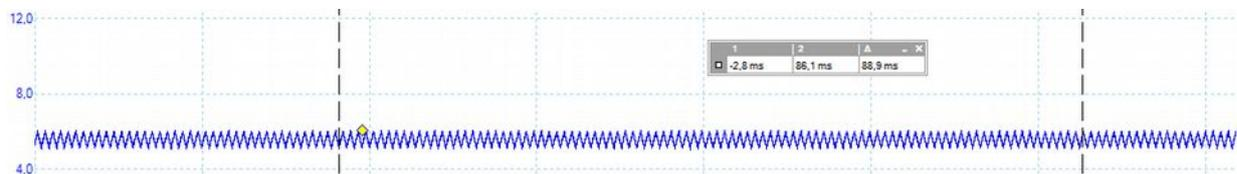
Figure 7 - Voltage on capacitor C3 with a 1.1 kHz square wave with 50% duty cycle
