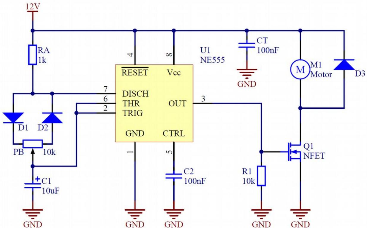
Figure 10 – PWM circuit with a fan on the output
