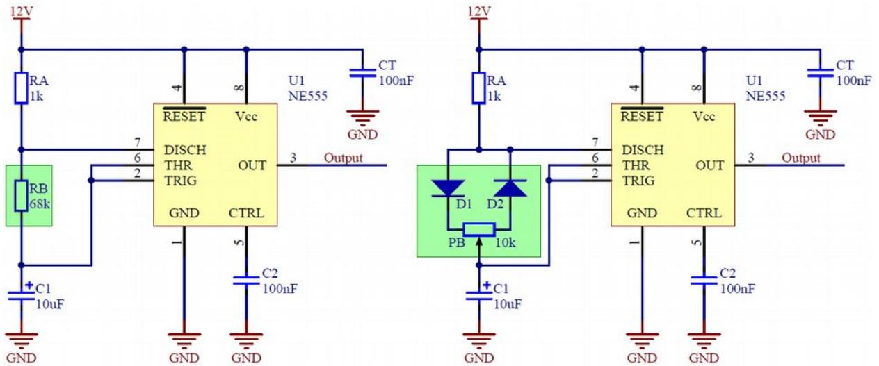
Figure 12 - The difference between the astable circuit and the PWM circuit
