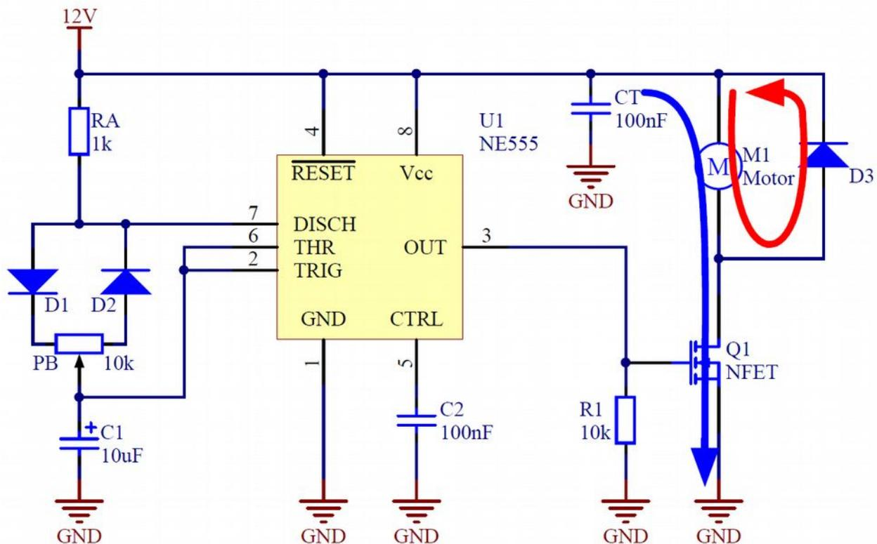
Figure 11 - Current flow paths when the Q1 FET is on (blue arrow), and off (red arrow)
