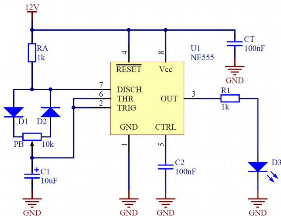
Figure 9 - PWM circuit with an LED on the output
