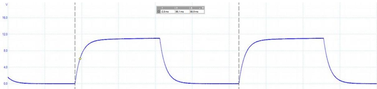
Figure 6 - Voltage on capacitor C3 with a 11 Hz square wave with 50% duty cycle
