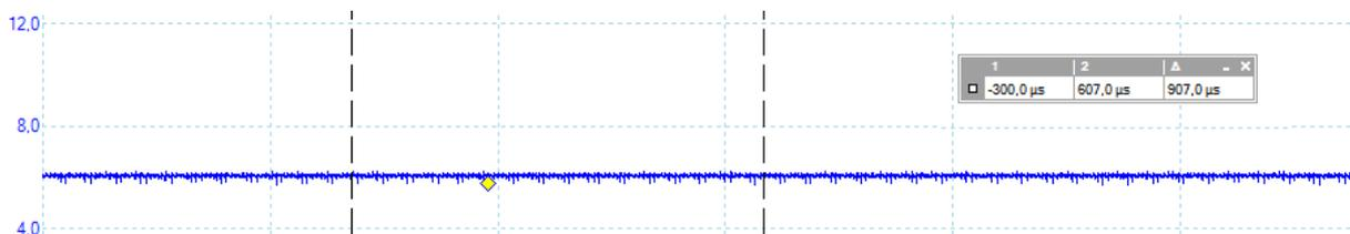
Figure 7 - Voltage on capacitor C3 with a 110 kHz square wave with 50% duty cycle
