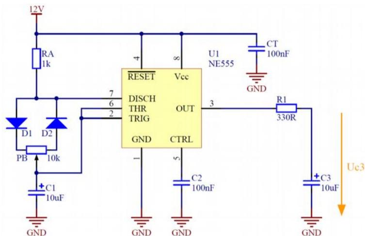
Figure 5 - PWM circuit, with and RC filter on the output
