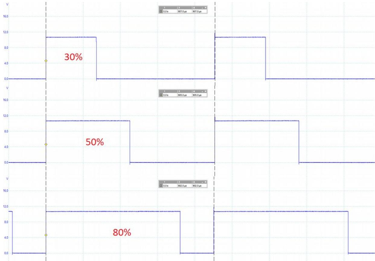
Figure 4 - PWM signals with different duty cycle
