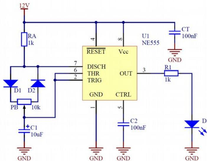
Figure 1 - Changing the brightness of a LED with NE555
