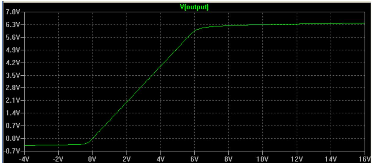
Figure 3 – Cathode voltage of the Zener diode
