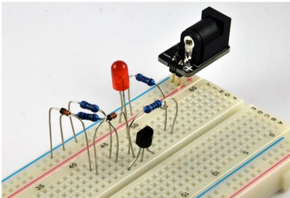
Figure 10 – Driving an LED using current source
