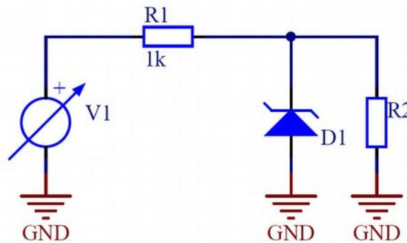
Figure 4 - Shunt voltage regulator
