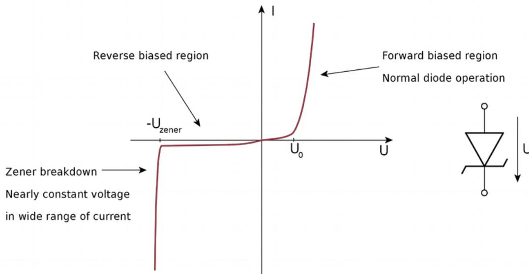
Figure 1 - Current-voltage curve of a Zener diode
