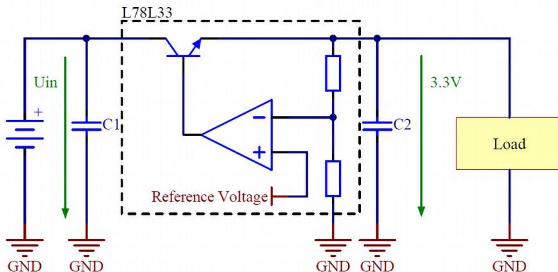
Figure 8 - Implementation of a voltage regulator with integrated circuits
