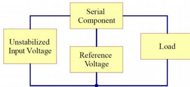
Figure 6 – Schematic structure of a series voltage regulator
