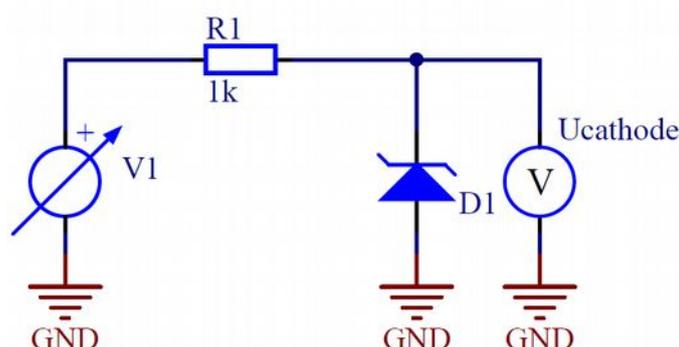
Figure 2 - Zener-diode with a resistor in series
