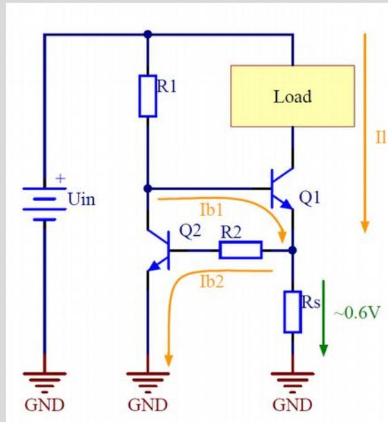
Figure 11 - Circuit diagram of a current limiter
