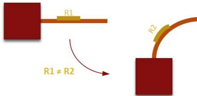
Figure 11 – Schematic structure of piezoresistive acceleration sensor
