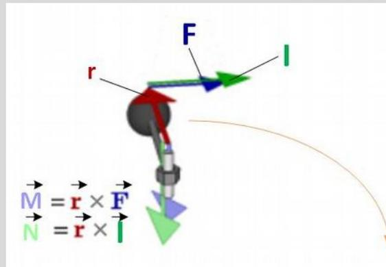
Figure 12 – Force, torque, momentum, angular momentum
