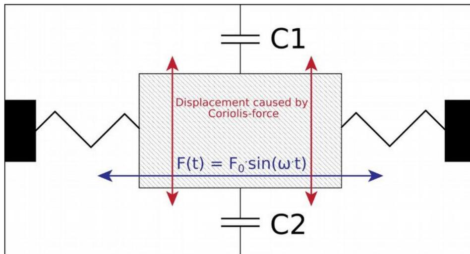
Figure 14 - Structure of the gyroscope which measures with a vibrating mass
