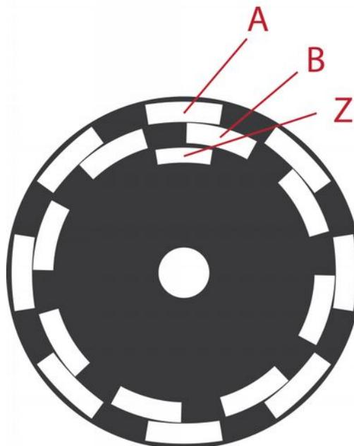
Figure 21 – Null impulse (Z) and rotating transmitter signals (A,B) on a disk
