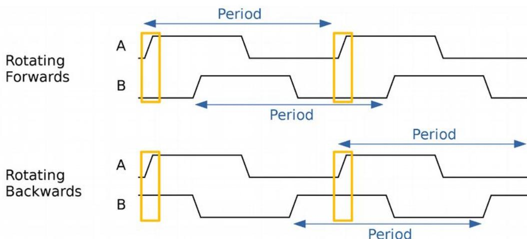
Figure 19 - Detecting rotation direction with incremental encoder
