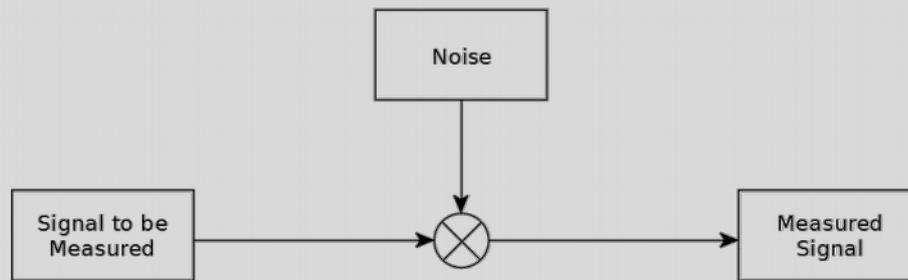
Figure 3 - Noise superimposed on the signal to be measured
