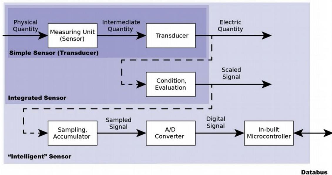
Figure 2 - General structure of sensors
