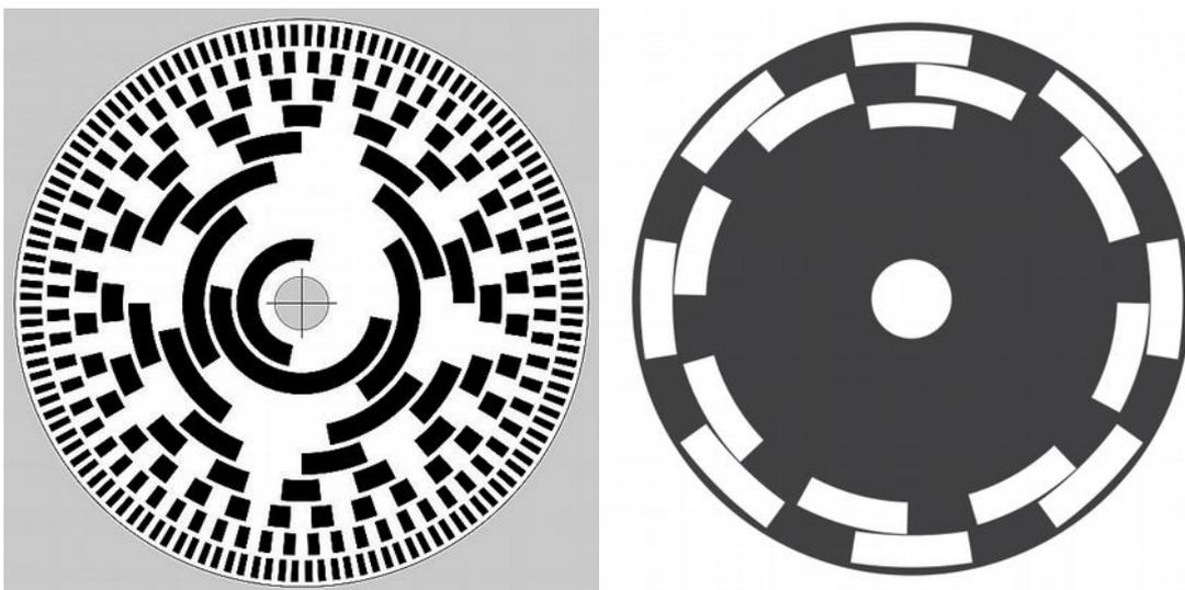
Figure 24 – Disks of absolute and incremental encoders
