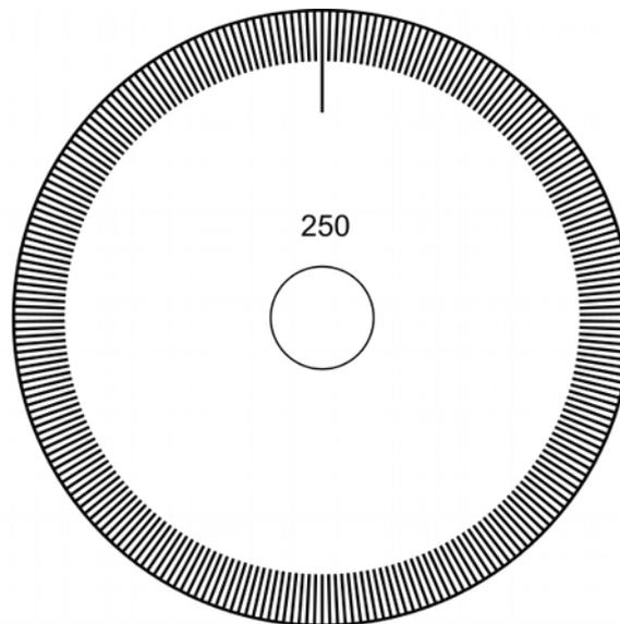
Figure 20 – Glass rotating disk with opaque metal marks
