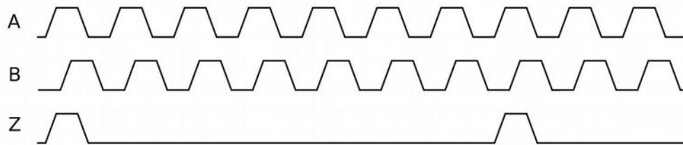
Figure 22 - Null impulse (Z) and rotating encoder signals (A,B)
