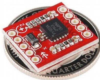
Figure 15 - Modern MEMS gyroscope
