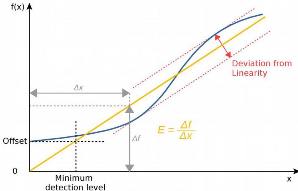
Figure 5 - Static characteristic
