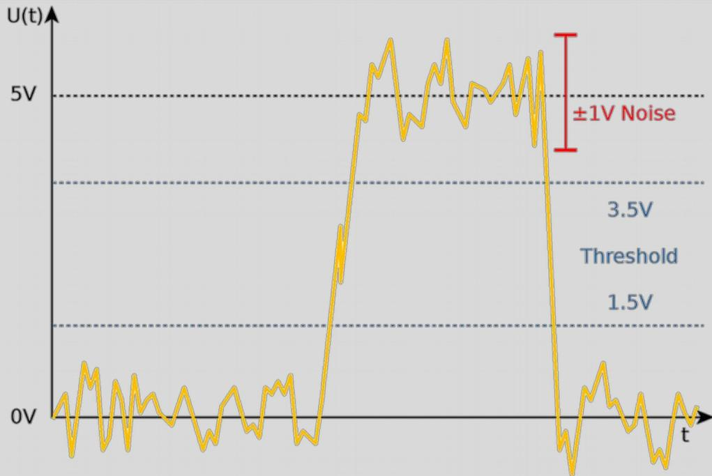
Figure 4 – Detection of short signals with noise
