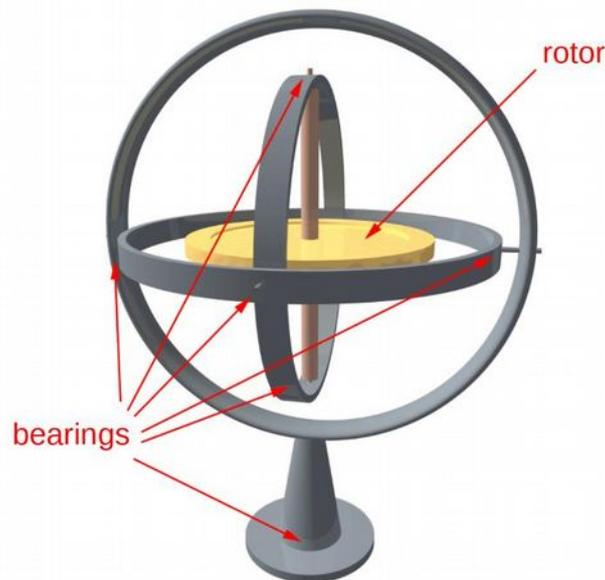
Figure 13 - Classic mechanical gyroscope
