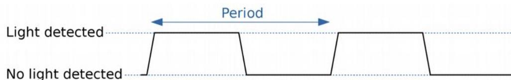
Figure 18 - Pulse train describing speed
