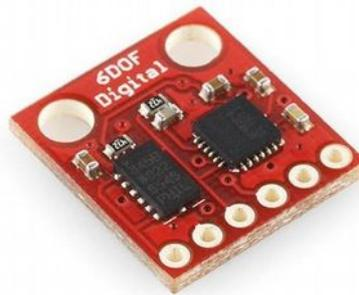
Figure 16 – Six degrees of freedom inertial sensor
