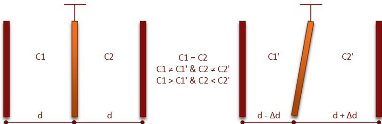
Figure 10 - Schematic structure of capacitive acceleration sensor
