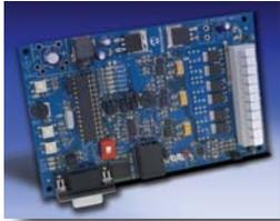
The PICDEM MCLV development board is intended for low-voltage (up to 48V), Brushless DC (BLDC) applications. The board provides a low-cost method for
