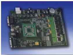
The dsPICDEM MCLV development board is intended for low-voltage BLDC applications up to 48 volts at 10 amps. It provides a low-cost method for users to evaluate and
