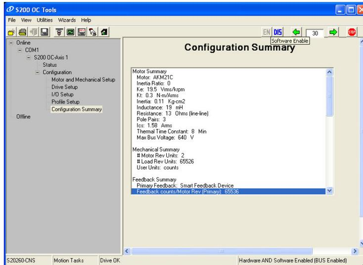
The configuration Summary screen allows the user to see all the drive settings in one location without having to navigate through each possible GUI menu.
