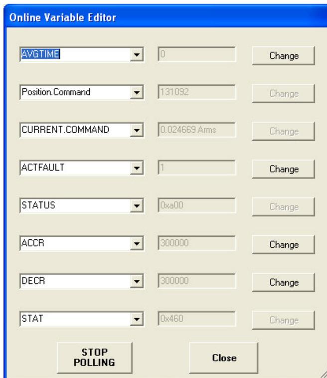
Although the variables available in the S200 Position Node product are not well documented there may be a reason that a user wants to view or change them. The Utilities/Edit Variables On-Line tool brings up this box which can be used to monitor or modify up to 8 variables at a time.
