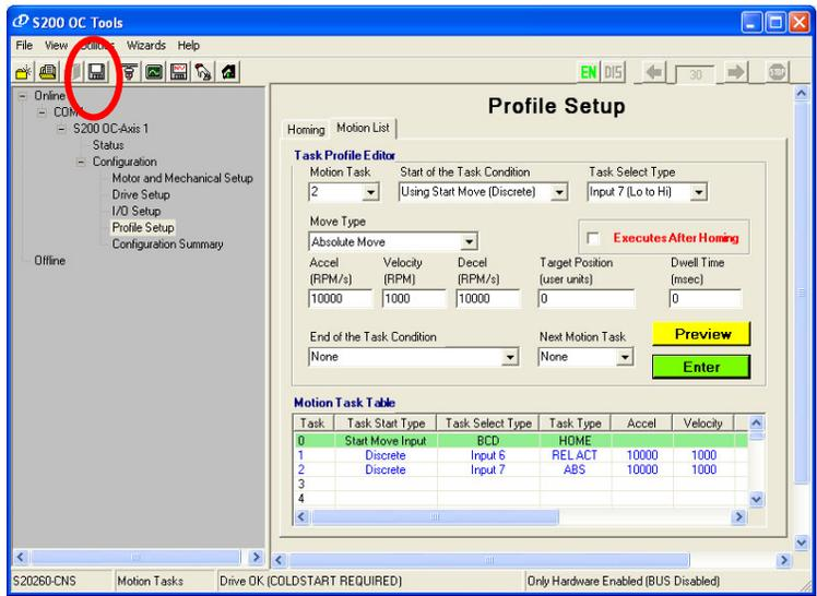
For demonstration purposes; the system shown on the left will index one motor turn (User Units are set to 65536 counts
