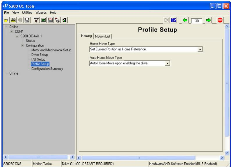
The Profile Setup menu allows you to set homing and motion tasks. This screen shows a handy method to set home when the system doesn't really need to have a home reference.
