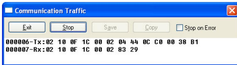
Note that this data traffic representation is sending the speed, 563, as a floating point data type.
