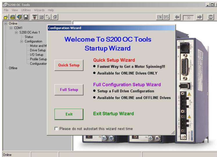
Once the data upload is complete, the wizard screen will appear. (Or can be invoked using 'Utilities / Full Setup
