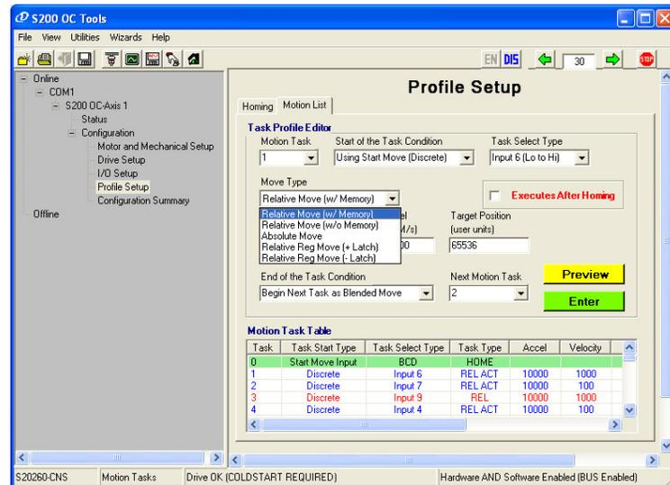
Move types include: Relative move with Memory: When indexing (relative moves) an early termination of prior moves is remembered. Choosing this Move Type calculates the next move
