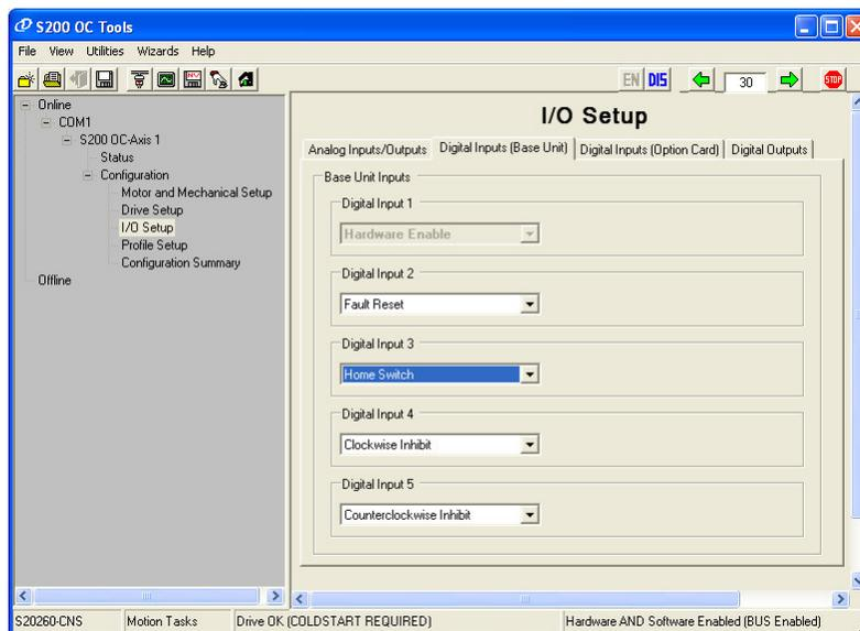
The I/O Setup tabs provide an easy and
