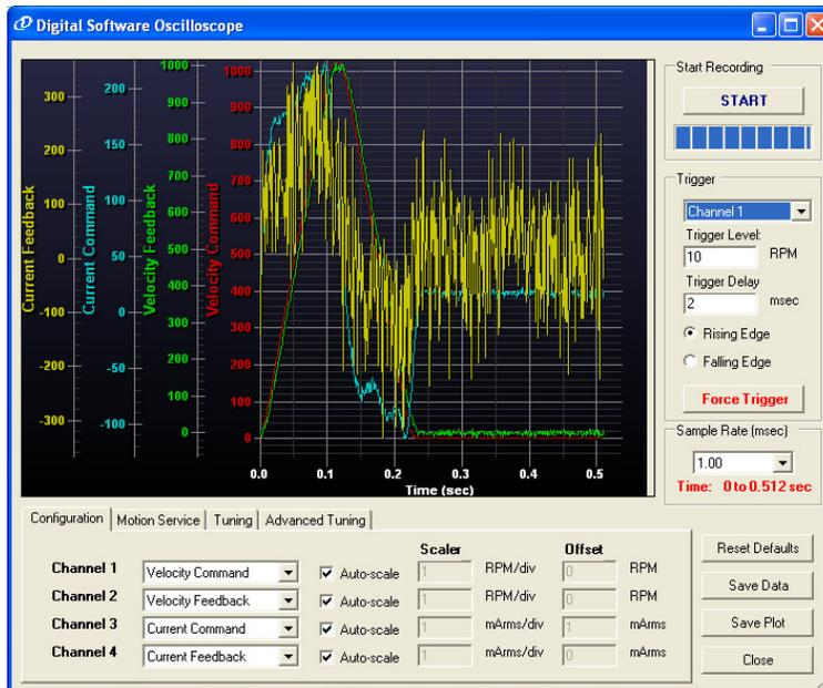
The plot to the left has AVGTIME set to 0. The effect of having AVGTIME set to a value is smoothing but setting AVGTIME to a large number can sometimes prevent the data from showing proper detail and relationship – as any low pass filter would. AVGTIME is the number of reads summed in the average calculation.
