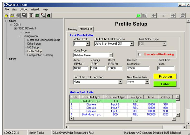
Set up motion tasks as required. Motion task 0 will always be a homing routine. The task number is the binary code if BCD select is used. See section 4 about more
