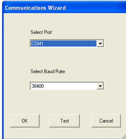
A communications wizard can be found under the Utilities menu. This allows you to select the RS232 communications port for the computer being used and allows a simple test of communications. Baud rate is always 38.4k Baud. Other port parameters are automatically set by S200 OC TOOLS.
