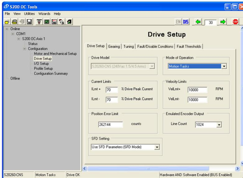
The Drive Setup tab is where the drive's mode of operation is set for Digital Velocity, Electronic Gearing or Motion tasks. This example has selected Motion
