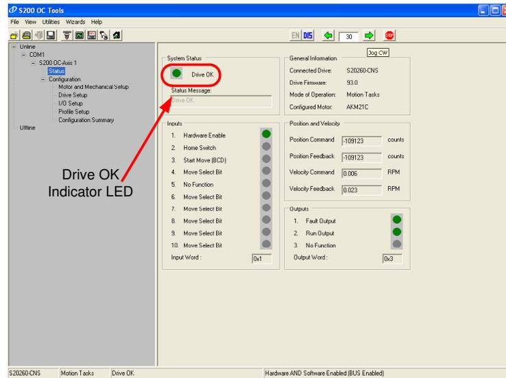
The Status screen can be helpful to understand system operation. Drive Status should read 'OK'. If not then a meaningful fault code will be shown. General information about drive size and firmware version is shown. Energizing a
