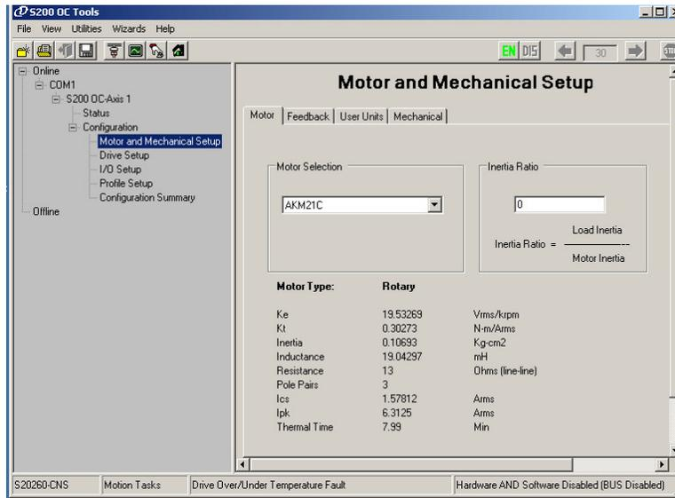
The first step is to confirm that the drive is configured for the motor being used. This information is automatically gathered from a system using an 'SFD-
