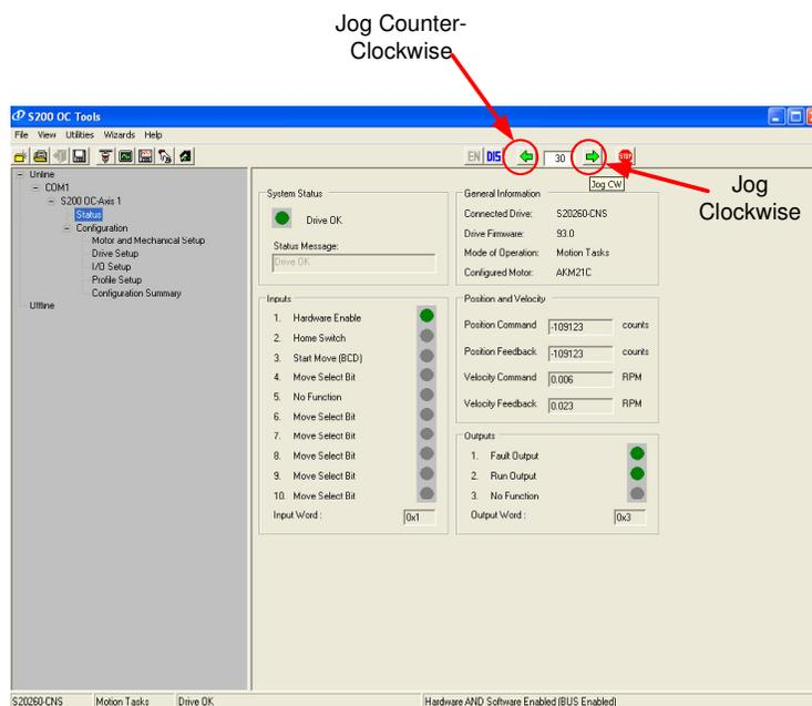
If the system is safe to accept motion then the motor can be jogged from the status screen.
