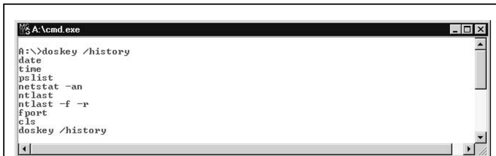
Figure 5-13. Using doskey to record the steps taken during incident response
