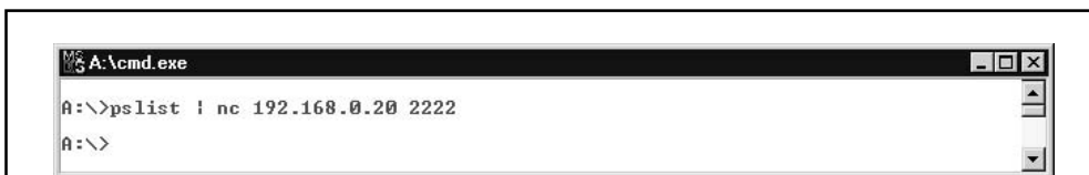
Figure 5-4. Sending the output of pslist to the forensic workstation
