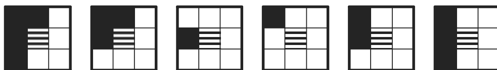
Figure 6. Set of 3 \times 3 templates designed to be used with DHTCJ, in increasing visual impact order. Only the templates that do not cause symbol connection or disconnection are listed. Hatched pixels match either black or white pixels. The score of a given pattern is that of the matching template with the lowest impact. Mirrors, rotations and reverses of each pattern have the same score.
