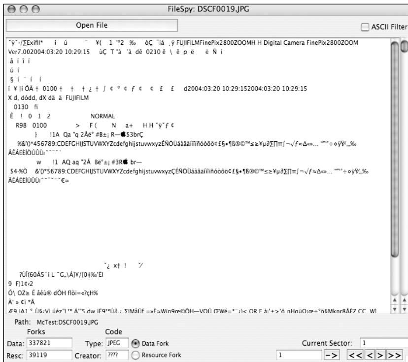
Figure 5.5 FileSpy Allows You to See the Raw EXIF Data in a JPG File
