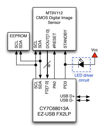
Fig. 2: Internal iSight architecture block diagram consisting of a Cypress EZ-USB, a Micron digital image sensor, a 16 byte configuration EEPROM, and an indicator LED.
