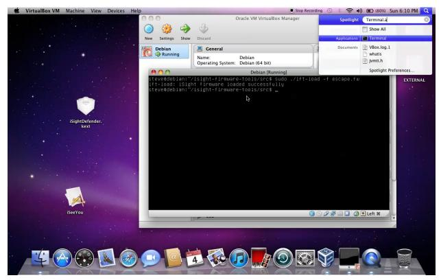
Fig. 4: Virtual machine escape. The iSight has been reprogrammed to act as a USB keyboard from inside a VirtualBox virtual machine and it is sending key presses to the host operating system. It is in the middle of entering "Terminal.app" into Spotlight.
