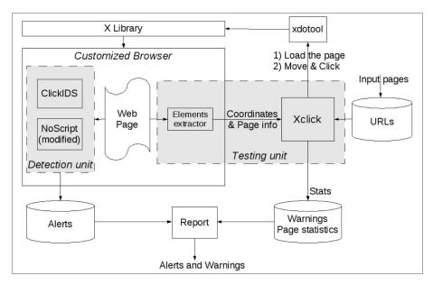
Figure 3.4.: System architecture of an automated detection system for clickjacking [1]
