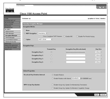
Figure 2.51 Entering the 26-Character Hexadecimal Encryption Key
