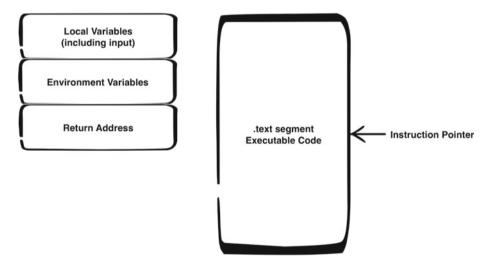
Figure 5-1. Stack and text segments
