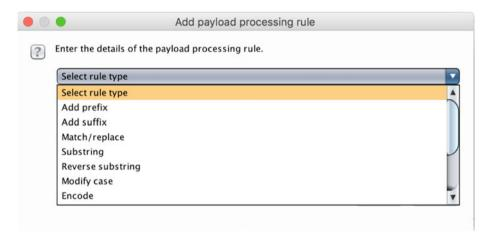
Figure 6-8. Payload processing options in Burp Suite
