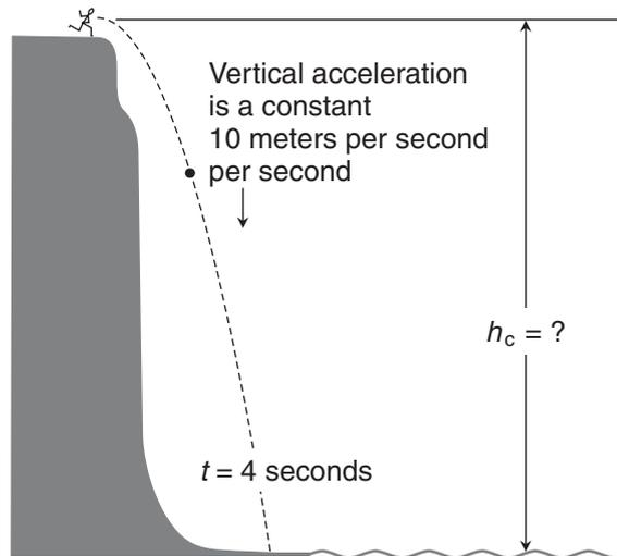
**Figure 27-1** Sir Isaac hurls an apple from the cliffs of Dover. The vertical acceleration is 10 meters per second per second, and the apple takes 4 seconds to fall. What is the altitude  $h_c$  of the apple above the beach at the instant it leaves Sir Isaac's hand?
