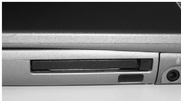
3. Insert the PC Card into the slot with the labeling up. Push the card until you feel a final resistance followed by a faint release, indicating full insertion into the slot. The following picture shows the PC Card fully inserted into the slot.
