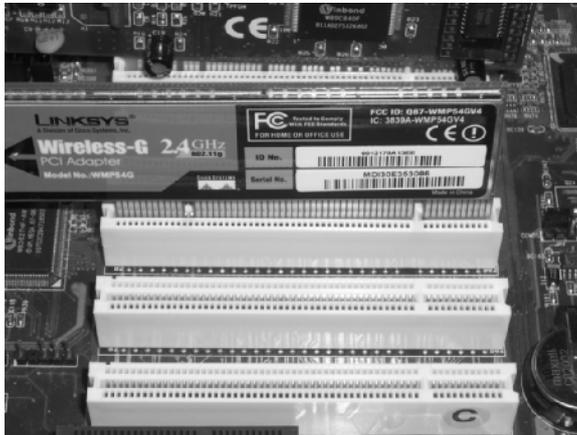
7. (Optional) Remove the existing card if necessary, paying attention to the fact that the card is likely secured, at the bracket, to the backplane. Note that there are various ways to secure cards. Sometimes screws are used, and sometimes mechanical clips. Pull the card firmly and evenly and make sure it's perpendicular to the board in which it is inserted.
