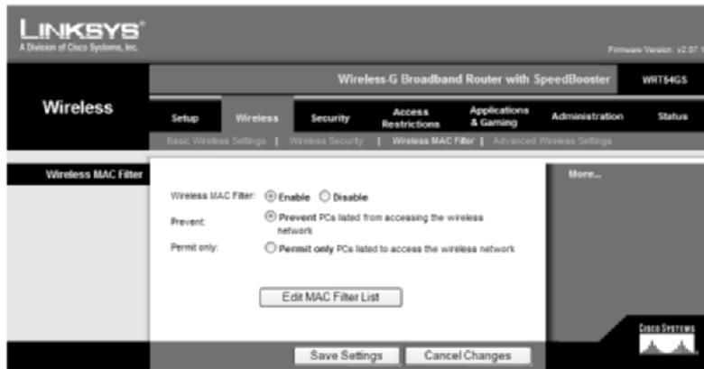
**FIGURE 1.17** Linksys router MAC Address Filter List screen
