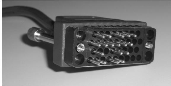
**FIGURE 2.13** Female V.35 connector
