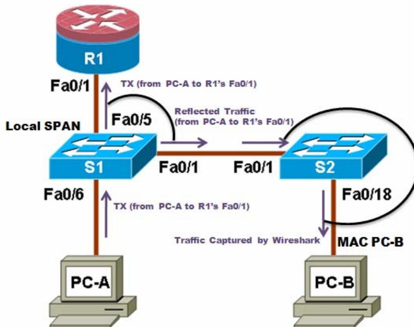
**Note:** Switch S2 is acting as a regular switch, forwarding frames based on destination MAC addresses and switch ports. The traffic entering S2 through Port Fa0/1 utilizes the R1's MAC address as destination for the Ethernet frame, therefore in order to forward those packets to PC-B, the R1's MAC address must be the same as PC-B. To accomplish this, R1's Fa0/1 MAC address is modified using the IOS CLI to simulate PC-B's MAC address. This requirement is specific to the NETLAB+ environment.
