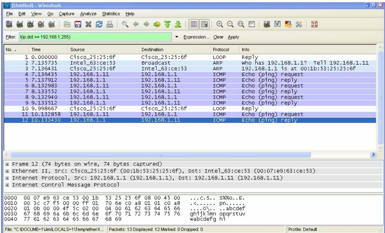
**Step 5: Monitor switch S1 port Fa0/5 SuperScan activity using Wireshark on PC-A.**
