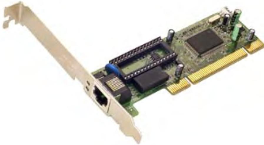
Figure 1-2: U.S. Robotics PCI network card.
