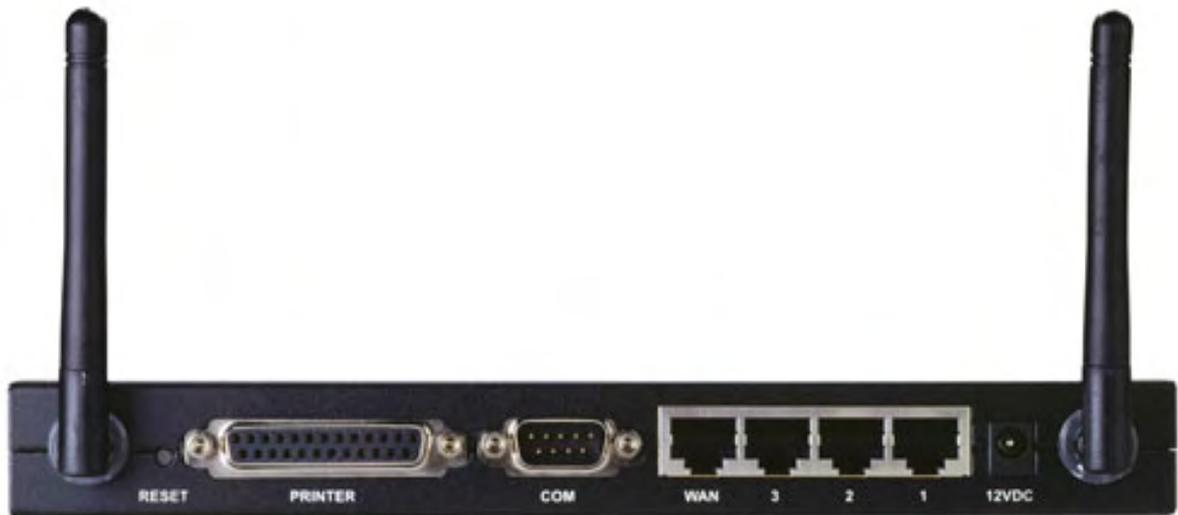
Figure 4-1: The printer connection on the back of a U.S. Robotics Model 8011 Wireless Cable and DSL Router.
