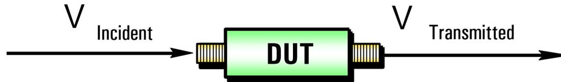
$$\text{Transmission Coefficient} = T = \frac{V_{\text{Transmitted}}}{V_{\text{Incident}}} = \tau \angle \phi$$
