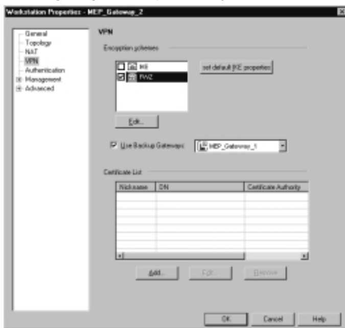
Figure 12.15 Configuring a Backup Gateway
