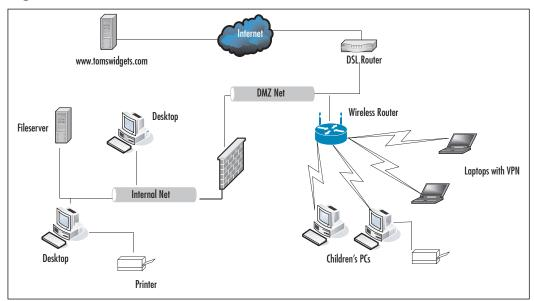
Choose the right firewall for your needs. If you don't have a GB connection, 1000Mbps is not useful. 10/100 is sufficient. DHCP, a decent management GUI for managing the firewall, wireless access points, virtual private networks, along with the type of filters, and the mechanism of firewalling are all aspects you need to analyze to determine what will be the most cost-effective with feature trade-offs. Don't implement services you won't use.
