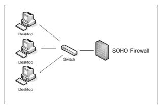
Most home routers designed for use with cable or DSL broadband Internet access come equipped with a basic packet filter firewall, or possibly even a stateful inspection firewall built in. The standard default configuration is generally to Deny All access unless you specifically configure it otherwise, but check the documentation for your router to make sure the firewall is on by default and what the default rule set is.
