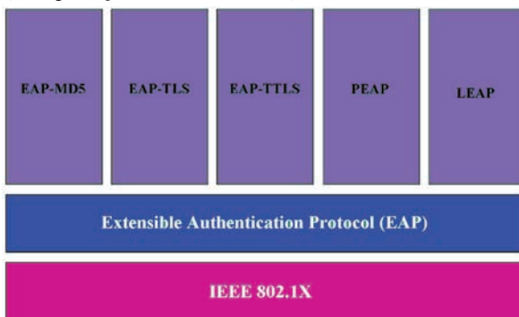
Figure 1. 802.1x authentication components (Adapted from Kwan, 2003)
