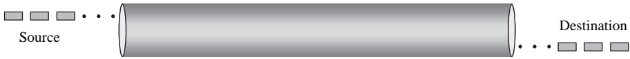
Figure 6.1 A flow: QoS is meaningful only for a flow between a specific source–destination pair
