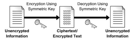
FIGURE 2-2 Implementing cryptography by using symmetric keys
