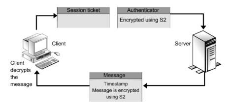
FIGURE 8-3 Client establishing connection with the application server
