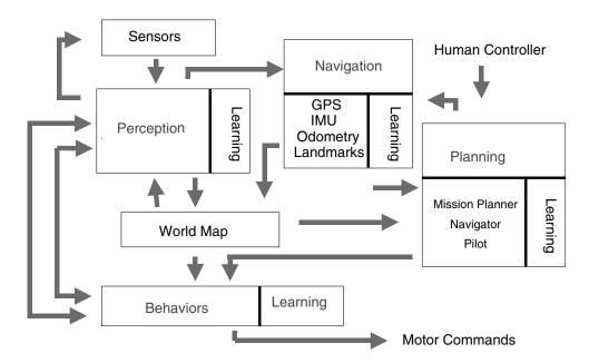
FIGURE 4-2 Autonomous behavior subsystems. Courtesy of Clint Kelley, SAIC.
