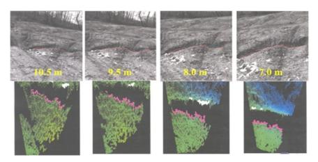
FIGURE C-7 Negative obstacle detection using stereo video. Courtesy of Larry Matthies, Jet Propulsion Laboratory.
