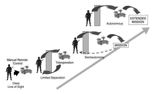
FIGURE 7-1 Evolution of UGV systems. SOURCE: AMCOM (2001).
