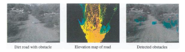
FIGURE D-4 Stereo obstacle detection results. Courtesy of Larry Matthies, Jet Propulsion Laboratory.
