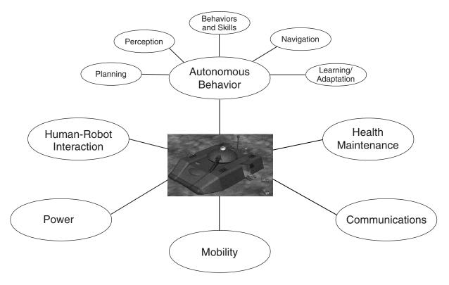
FIGURE 5-1 Areas of technology needed for UGVs.
