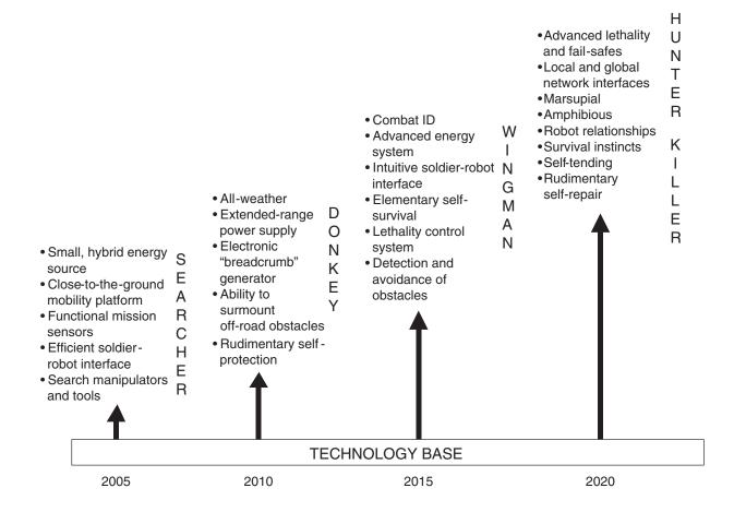
FIGURE 7-2 Possible evolution of UGV system capabilities.
