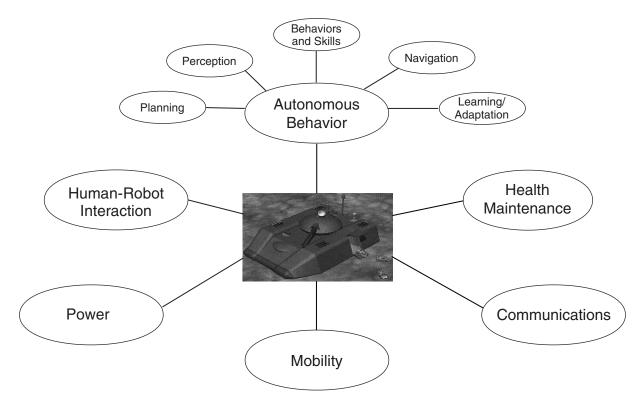
FIGURE 4-1 Areas of technology needed for UGVs.
