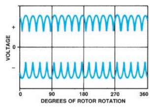
Figure 8-32. The diodes receive the maximum voltage values.
