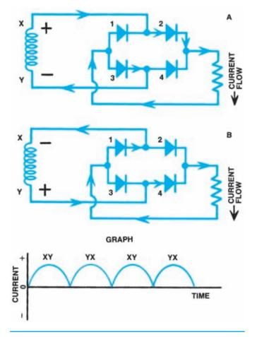
Figure 8-8. More diodes are needed in the circuit for full-wave rectification. (Delphi Automotive Systems)
