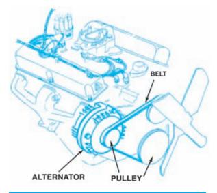
Figure 8-13. AC generator (alternator) and drive pulley. (DaimlerChrysler Corporation)
