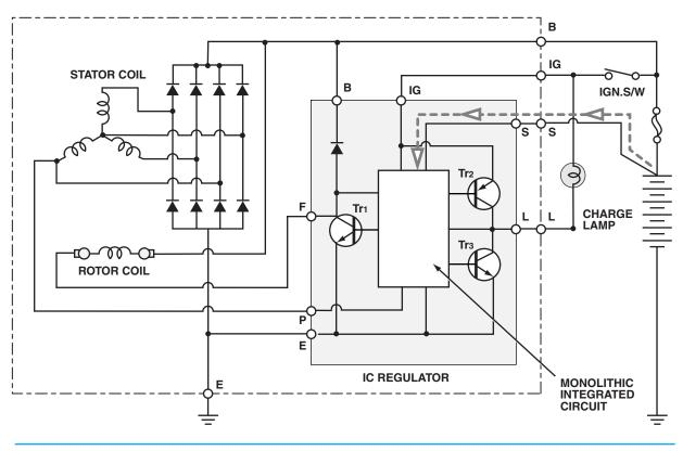
**Figure 8-56.** When AC generator voltage is too high, the regulator momentarily cuts off current to the rotor coils, eliminating the magnetic field. The rotor continues to spin, but no voltage is generated. (Reprinted by permission of Toyota Motor Corporation)
