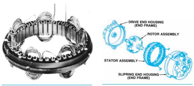
Figure 8-15. A stator with only one conductor installed. (Delphi Automotive Systems)
