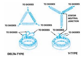
Figure 8-23. Two types of stator windings. (Daimler-Chrysler Corporation)
