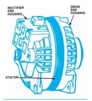
Figure 8-17. AC generator (alternator) with exposed stator core.
