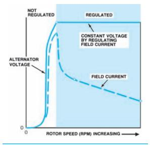
Figure 8-37. Field current is decreased as rotor speed increases, to keep AC generator (alternator) output voltage at a constant level.
