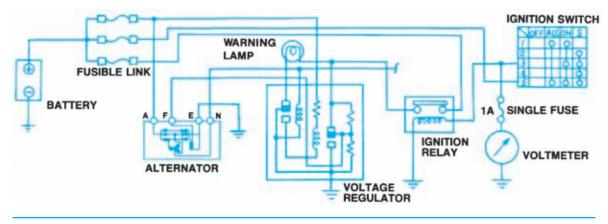
Figure 8-53. A typical voltmeter circuit.
