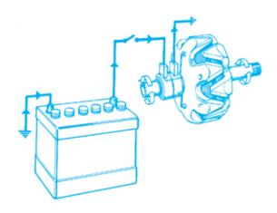
**Figure 8-19.** The sliprings and brushes carry current to the rotor windings.
