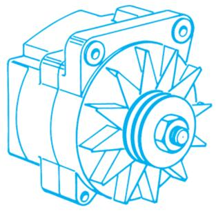
Figure 8-18. AC generator (alternator) with the stator core enclosed.
