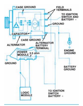
**Figure 8-67.** Typical DaimlerChrysler computer voltage regulation with DaimlerChrysler 40/90-ampere AC generator (alternator). Circuit connections vary on different models. (DaimlerChrysler Corporation)
