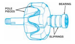
Figure 8-9. Rotor. (DaimlerChrysler Corporation)
