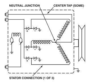
Figure 8-25. A Y-type stator circuit diagram. The center tap connects to the neutral junction of the Y-type stator of some AC generators. (DaimlerChrysler Corporation)
