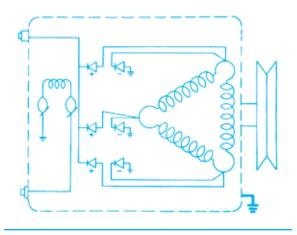
Figure 8-26. Circuit diagram of a delta-type stator.
