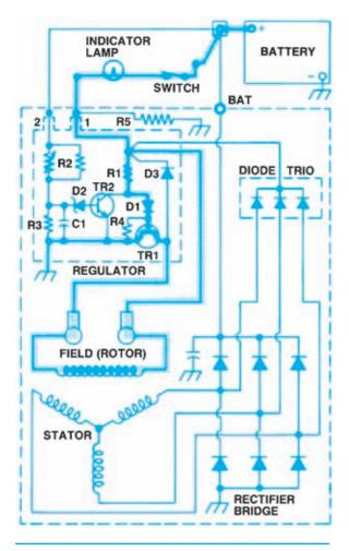
Figure 8-43. Field current in a typical solid-state regulator during starting. (Delphi Automotive Systems)
