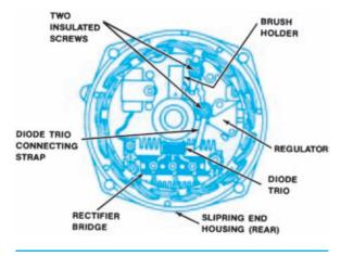
Figure 8-61. The rear end housing of the later-model 10-SI. (Delphi Automotive Systems)
