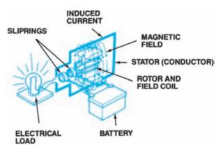
**Figure 8-3.** An AC generator (alternator) is based on the rotation of a magnet inside a fixed-loop conductor. (DaimlerChrysler Corporation)
