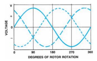
Figure 8-29. The three-phase voltage from one revolution of the rotor. (Reprinted by permission of Robert Bosch GmbH)
