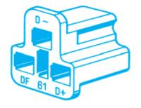
Figure 8-39. Most regulators use a multiple-plug connector to ensure connections are properly made. (Reprinted by permission of Robert Bosch GmbH)
