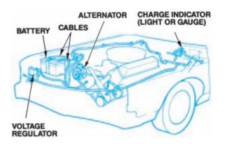
Figure 8-2. Major components of an automotive charging system. (DaimlerChrysler Corporation)
