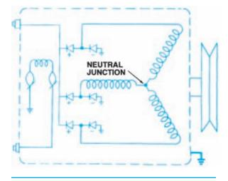
Figure 8-24. Y-type stator circuit diagram. (Daimler-Chrysler Corporation)
