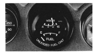
Figure 8-52. Automotive voltmeter in instrument panel.
