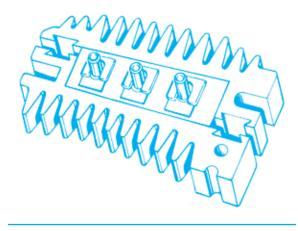
Figure 8-21. Positive and negative diodes may be mounted in a heat sink for protection.
