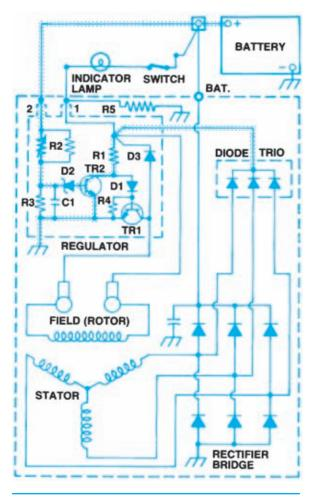
Figure 8-45. When AC generator (alternator) output voltage reaches a maximum safe level, no current is allowed in the rotor winding. (Delphi Automotive Systems)
