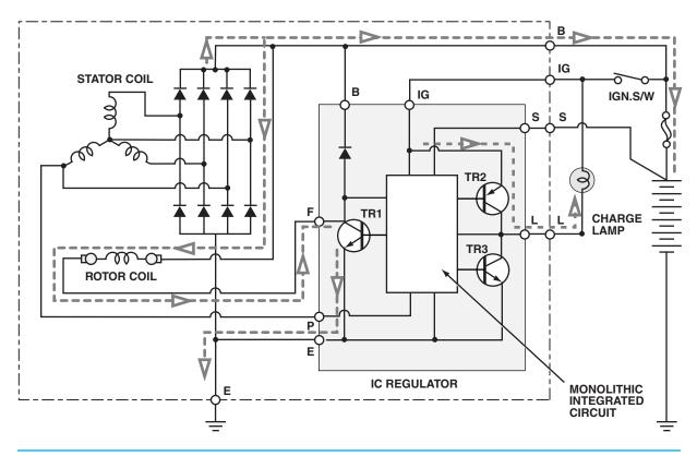
Figure 8-58. After the engine is running, the AC generator generates a voltage greater than the battery. The charge light goes out, indicating normal operation. (Reprinted by permission of Toyota Motor Corporation)
