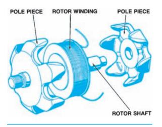
Figure 8-11. The magnetic field of the rotor is created by current through the rotor winding. (Reprinted by permission of Robert Bosch GmbH)
