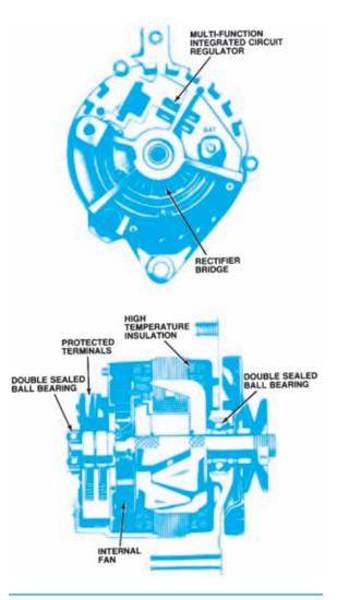
Figure 8-63. Typical Delco-Remy CS series AC generator (alternator) construction. (Delphi Automotive Systems)
