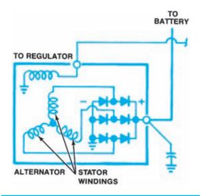
Figure 8-20. Each conductor is attached to one positive and one negative diode.
