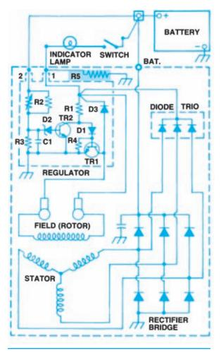
Figure 8-54. GM warning lamp circuit. (GM Service and Parts Operations)
