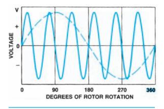
Figure 8-30. An AC generator (alternator) with six pairs of N-S poles would produce the solid line voltage trace. The dashed line represents an alternator with one pair. (Reprinted by permission of Robert Bosch GmbH)
