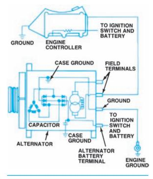
**Figure 8-69.** Current DaimlerChrysler charging system. (DaimlerChrysler Corporation)
