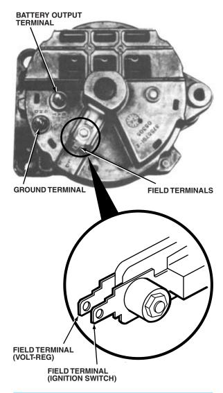
Figure 8-66. The terminals on a 100-amp Daimler-Chrysler AC generator (alternator). (DaimlerChrysler Corporation)
