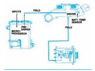
Figure 8-49. Battery temperature circuit of the Daimler-Chrysler computer regulated charging system. (Daimler-Chrysler Corporation)
