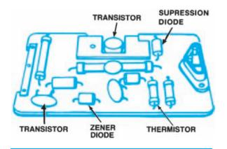
Figure 8-47. DaimlerChrysler solid-state voltage regulator. (DaimlerChrysler Corporation)
