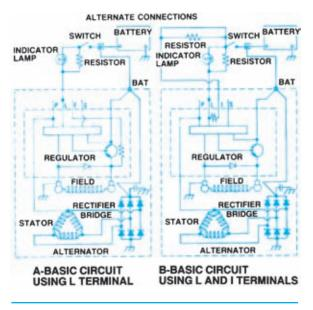
Figure 8-64. Two basic circuits for CS AC generators (alternator). (Delphi Automotive Systems)
