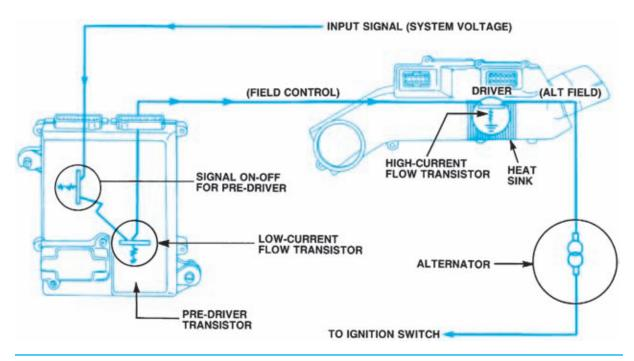
Figure 8-68. DaimlerChrysler computer-regulated charging system internal field control. (DaimlerChrysler Corporation)
