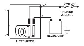
Figure 8-35. An A-circuit. (Regulator is after the field.)
