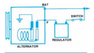
Figure 8-36. A B-circuit. (Regulator is before the field.)
