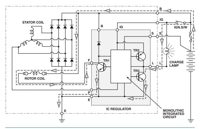
**Figure 8-57.** When the ignition is on and the engine is not running, the regulator energizes the rotor coil to build a magnetic field in the stator. The regulator turns on the charge light, indicating that the AC generator is not generating a voltage. (Reprinted by permission of Toyota Motor Corporation)
