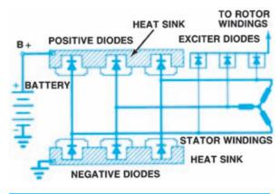
Figure 8-34. Some AC generators (alternators) have additional diodes to rectify field current. (Reprinted by permission of Robert Bosch GmbH)
