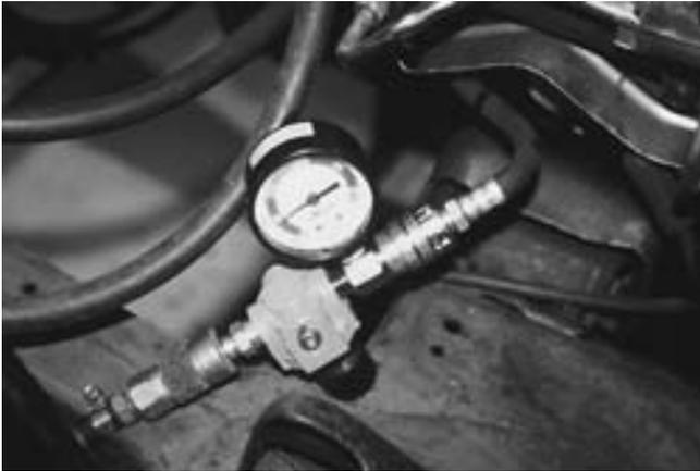
**FIGURE 20-13** A typical handheld cylinder leakage tester.
