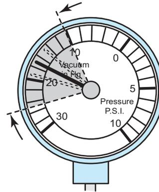
**FIGURE 20-19** A leaking head gasket can cause the needle to vibrate as it moves through a range from below to above normal.
