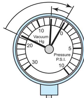
**FIGURE 20-26** A needle that drops to near zero when the engine is accelerated rapidly and then rises slightly to a reading below normal indicates an exhaust restriction.
