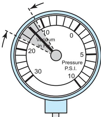
**FIGURE 20-18** A gauge reading with the needle fluctuating 3 to 9 in. Hg below normal often indicates a vacuum leak in the intake system.
