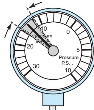
**FIGURE 20-20** An oscillating needle 1 or 2 in. Hg below normal could indicate an incorrect air–fuel mixture (either too rich or too lean).
