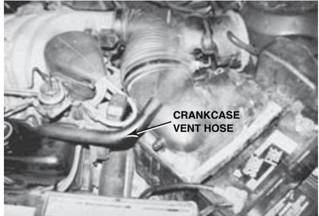
**FIGURE 20-1** Blowby gases coming out of the crankcase vent hose. Excessive amounts of combustion gases flow past the piston rings and into the crankcase.
