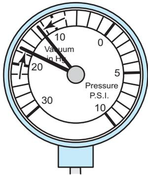
**FIGURE 20-22** If the needle drops 1 or 2 in. Hg from the normal reading, one of the engine valves is burned or not seating properly.
