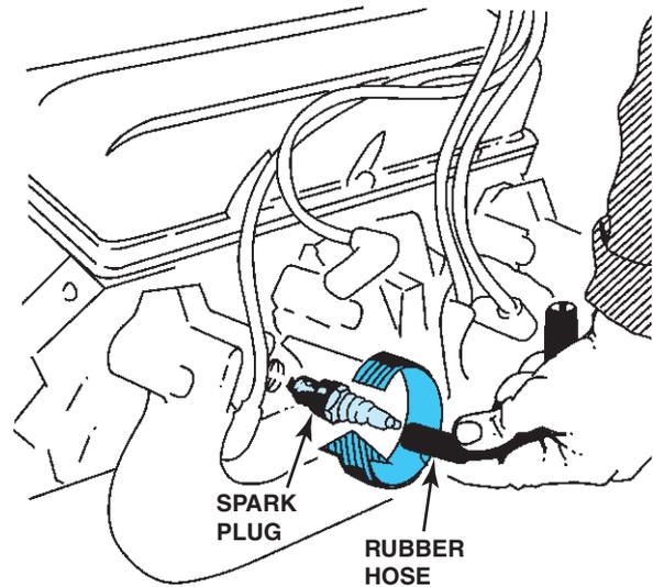
**FIGURE 20-11** Use a vacuum or fuel line hose over the spark plug to install it without danger of cross-threading the cylinder head.
