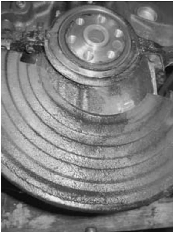
**FIGURE 20-4** The transmission and flex plate (flywheel) were removed to check the exact location of this oil leak. The rear main seal and/or the oil pan gasket could be the cause of this leak.
