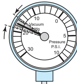
**FIGURE 20-21** A rapidly vibrating needle at idle that becomes steady as engine speed is increased indicates worn valve guides.
