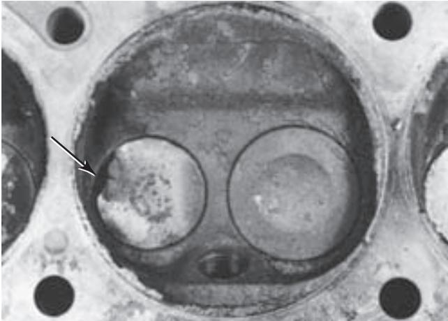
**FIGURE 20-12** Badly burned exhaust valve. A compression test could have detected a problem, and a cylinder leakage test (leak-down test) could have been used to determine the exact problem.
