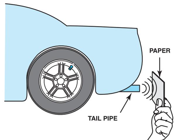
**FIGURE 20-9** The paper test involves holding a piece of paper near the tailpipe of an idling engine. A good engine should produce even, outward puffs of exhaust. If the paper is sucked in toward the tailpipe, a burned valve is a possibility.
