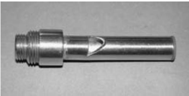
**FIGURE 20-14** A whistle stop used to find top dead center. Remove the spark plug and install the whistle stop, then rotate the engine by hand. When the whistle stops making a sound, the piston is at the top.
