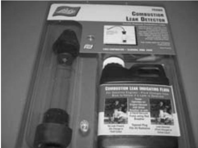
**FIGURE 20-28** A tester that uses a blue liquid to check for exhaust gases in the exhaust, which would indicate a head gasket leak problem.
