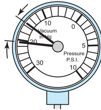
**FIGURE 20-25** A steady needle reading that rises 2 or 3 in. Hg when the engine speed is increased slightly above idle indicates that the ignition timing is advanced.
