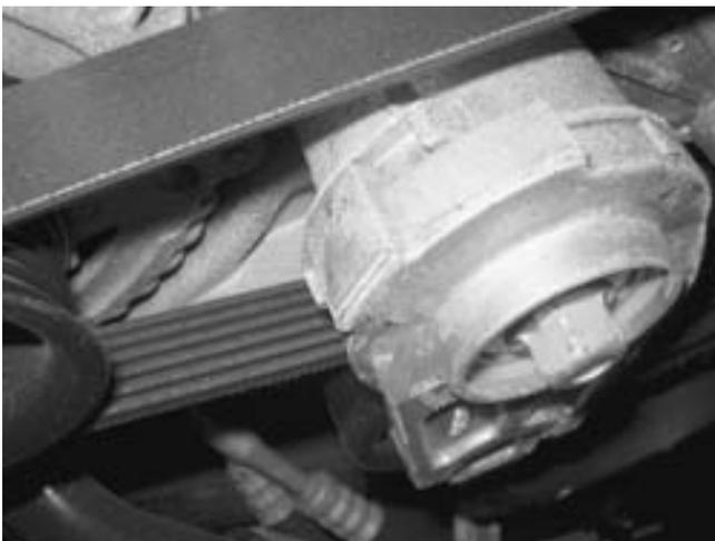
**FIGURE 20-6** An accessory belt tensioner. Most tensioners have a mark that indicates normal operating location. If the belt has stretched, this indicator mark will be outside of the normal range. Anything wrong with the belt or tensioner can cause noise.
