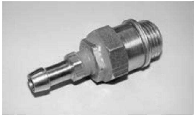
**FIGURE 20-27** A technician-made adapter used to test exhaust system backpressure. The upstream oxygen sensor is removed and the adaptor is threaded into the opening in the exhaust and then a pressure gauge to connected to the hose fitting so that backpressure can be measured.
