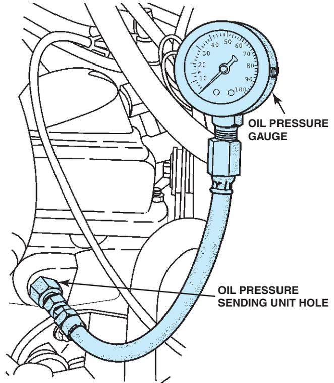
**FIGURE 20-8** To measure engine oil pressure, remove the oil pressure sending (sender) unit usually located near the oil filter. Screw the pressure gauge into the oil pressure sending unit hole.
