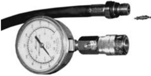
**FIGURE 20-10** A two-piece compression gauge set. The threaded hose is screwed into the spark plug hole after removing the spark plug. The gauge part is then snapped onto the end of the hose.
