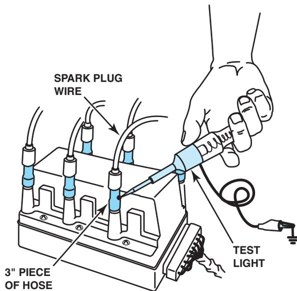
**FIGURE 20-15** Using a vacuum hose and a test light to ground one cylinder at a time on a distributorless ignition system. This works on all types of ignition systems and provides a method for grounding out one cylinder at a time without fear of damaging any component.
