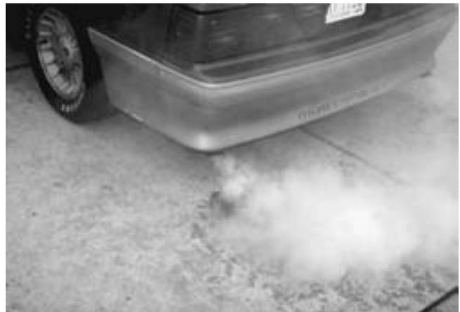
**FIGURE 20-2** White steam is usually an indication of a blown (defective) cylinder head gasket that allows engine coolant to flow into the combustion chamber where it is turned to steam.
