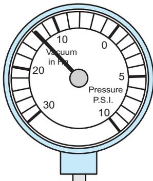
**FIGURE 20-17** A steady but low reading could indicate retarded valve or ignition timing.
