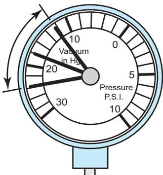
**FIGURE 20-23** Weak valve springs will produce a normal reading at idle, but as engine speed increases, the needle will fluctuate rapidly between 12 and 24 in. Hg.
