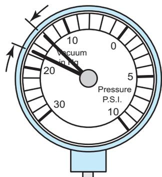
**FIGURE 20-24** A steady needle reading that drops 2 or 3 in. Hg when the engine speed is increased slightly above idle indicates that the ignition timing is retarded.
