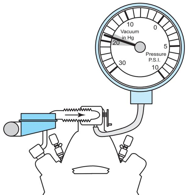
**FIGURE 20-16** An engine in good mechanical condition should produce 17 to 21 in. Hg of vacuum at idle at sea level.
