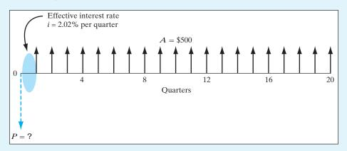
**Figure 4.5** A present-worth calculation for an equal payment series with an interest rate of 8% compounded continuously (Example 4.6).
