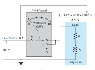
**FIG. 19.7** Demonstrating the reason for rating a load in kVA rather than kW.
