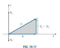
Impedance diagram for a series R-L-C circuit.
