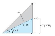
FIG. 19.28 Demonstrating the impact of power-factor correction on the power triangle of a network.
