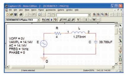
FIG. 19.42 Using PSpice to examine the power distribution in a series R-L-C circuit.
