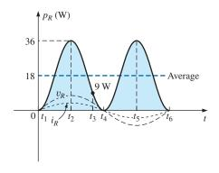
FIG. 19.5 Power curve for Example 19.1.
