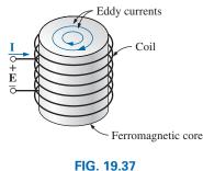
Defining the eddy current losses of a ferromagnetic core.
