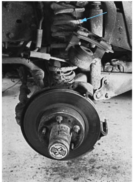
**FIGURE 14-15** The brake caliper has been removed from its mounts and is suspended from the spring using a wire hook to prevent it from falling and possibly damaging the brake hose.
