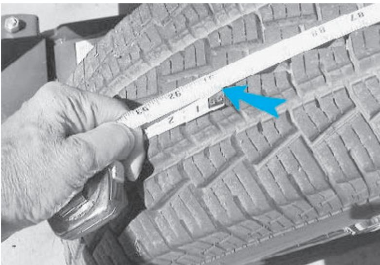
**FIGURE 14-6** The measuring tape wrapped around the tire shows that the circumference is 90 3/4 in. The other three tires should measure close to the same.
