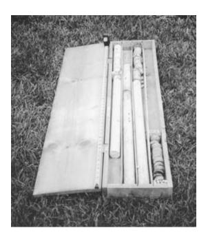
Core recovery is the length of core obtained divided by the distance drilled. For example, a laminated shale stratum with a number of clay seams would likely exhibit a relatively small percentage of core recovery because the clayey soil originally located between laminations may have been washed or blown away by the
