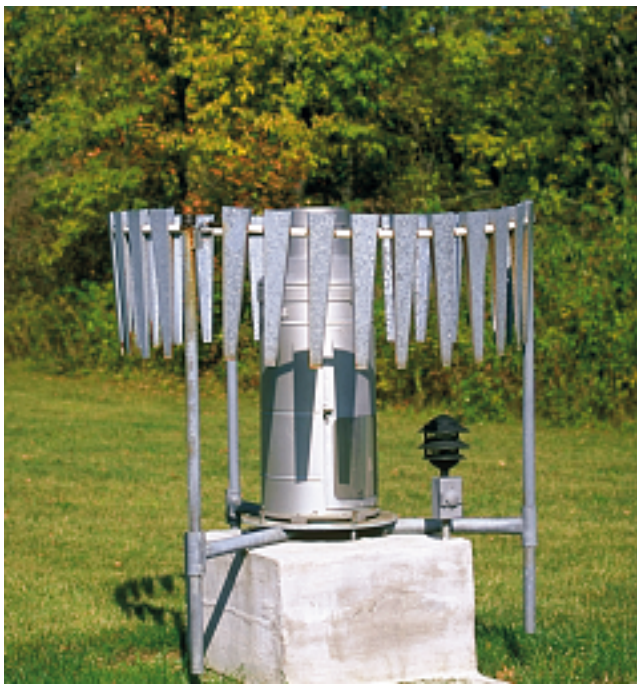
FIGURE 5-26 This standard rain gauge is fitted with metal slats that serve as a windscreen to minimize the undercatch that results because of windy conditions. (Photo by Bobbé Christopherson)
