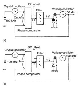
Figure 6.4 Simple phase-locked loop
