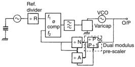
Figure 6.6 Programmable frequency synthesizer
