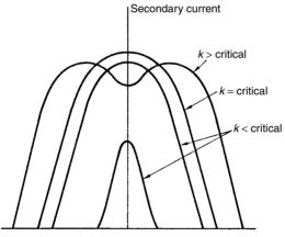
Figure 5.5 Effect of degree of coupling
