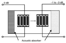
Figure 7.9 Single-phase unidirectional filter configuration
