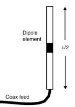
Figure 4.9 Type EDV end-fed antenna (by kind permission of C and S Antennas Ltd)
