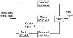
Figure 8.5 Phase shift production of single sideband
