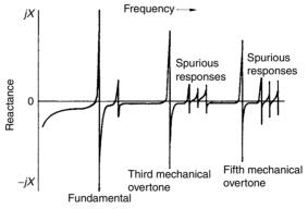
Figure 7.5 Overtone response of a quartz crystal
