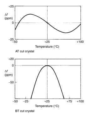
Figure 7.3 Frequency vs. temperature curves AT and BT cut crystals
