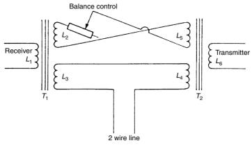
Figure 3.2 Balanced line hybrid
