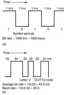
Figure 8.1 Bit rate and baud rate
