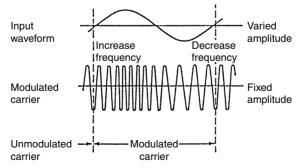
Figure 8.6 Frequency modulation
