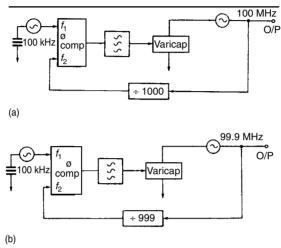
Figure 6.5 Frequency variable phase-locked loop
