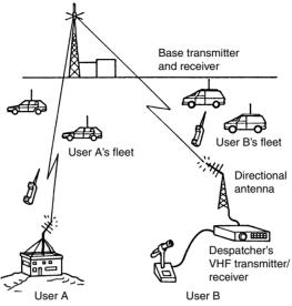
Figure 15.4 Common base station system
