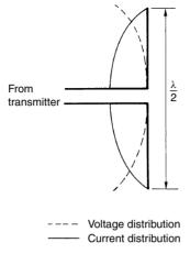
Figure 1.4 Doublet (dipole) antenna
