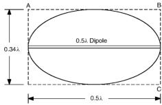
**Figure 4.1B** Capture area of half-wavelength  $(0.5\lambda)$  dipole
