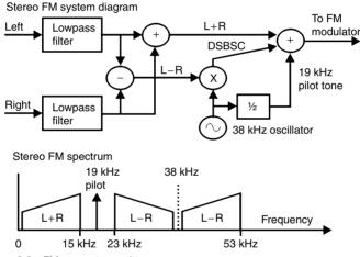
Figure 8.8 FM stereo transmitter
