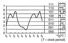
Figure 14.2 Eight-level pulse code modulation
