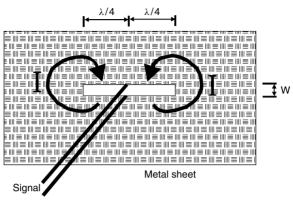
Figure 4.13 Slot antenna
