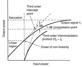
Figure 19.2 Production of intermodulation
