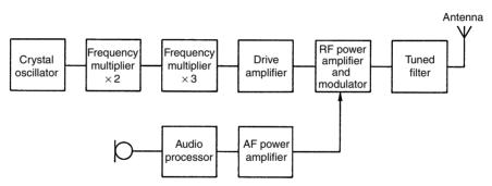
Figure 10.1 Crystal controlled AM transmitter
