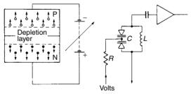
Figure 6.3 Voltage variable capacitance diode
