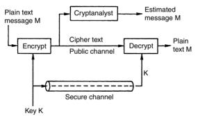
Figure 12.1 Cryptographic channel
