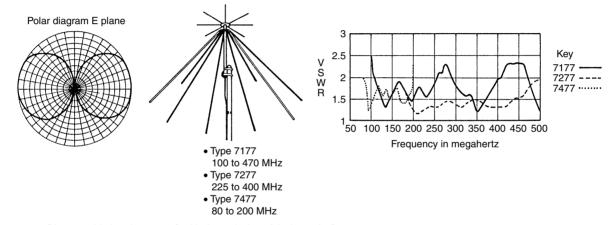
Figure 4.14 Discone wide band antenna (by kind permission of Jaybeam Ltd)
