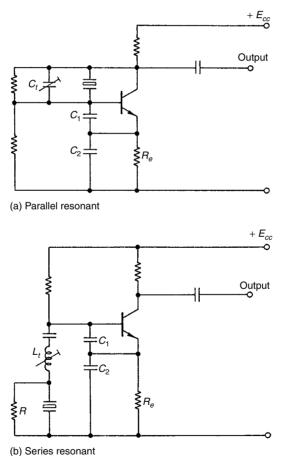
Figure 6.2 Quartz crystal oscillators
