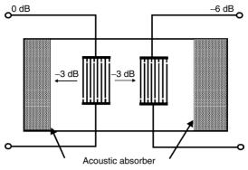
Figure 7.8 Simple transversal SAW filter configuration
