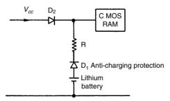
Figure 21.1 Typical lithium battery application
