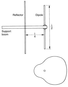
Figure 4.11 Dipole and reflector
