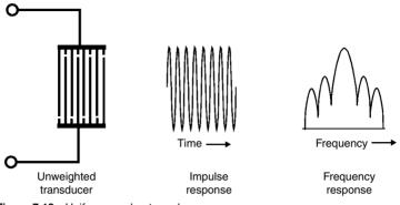
Figure 7.10 Uniform-overlap transducer
