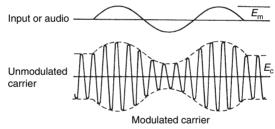
Figure 8.2 Amplitude modulation
