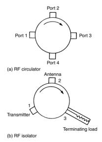
Figure 19.3 RF circulator and isolator
