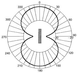
Figure 4.20 Small loop azimuth
