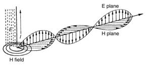
Figure 1.3 Formation of electromagnetic wave
