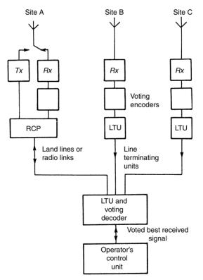
Figure 15.5 Radio scheme with one transmit/receive plus two receiver-only stations with voting
