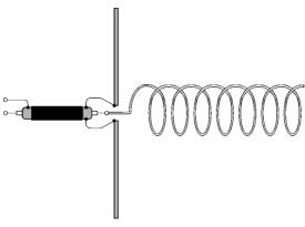
Figure 4.17 Axial mode helical antenna
