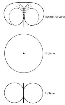
Figure 4.2 Radiation patterns of a half-wave dipole
