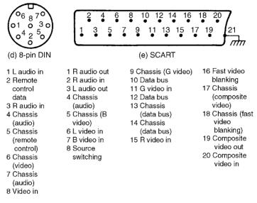
The simplest is a source switching input (pin 8) in which an external source (videorecorder, computer, etc.) can, by issuing a 12 volt signal, cause the television to switch to baseband inputs.
