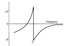
Figure 7.2 Crystal reactance close to resonance
