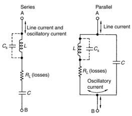
Figure 5.1 Series and parallel resonant circuits
