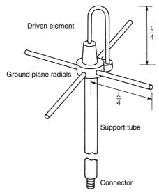
Figure 4.10 Folded unipole antenna
