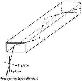
Figure 3.6 Propagation in rectangular waveguide
