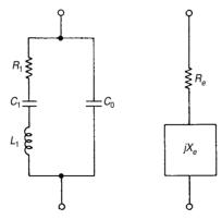
Figure 7.1B Equivalent circuit of a crystal
