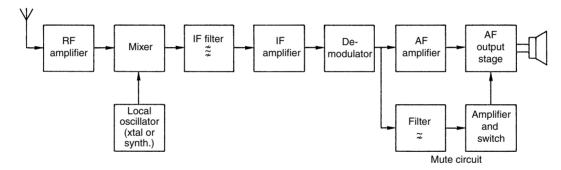
Figure 10.3 FM single superheterodyne receiver
