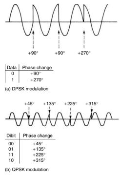
Figure 8.11 DPSK and QPSK
