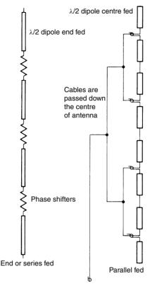
Figure 4.12 General construction of co-linears
