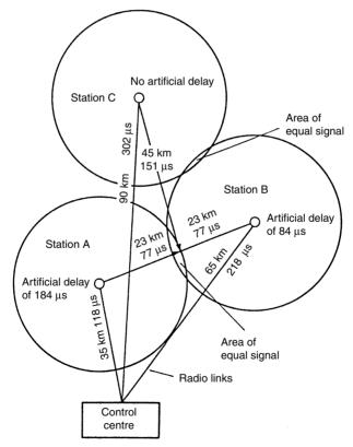
Figure 15.6 Quasi-synchronous transmitter system
