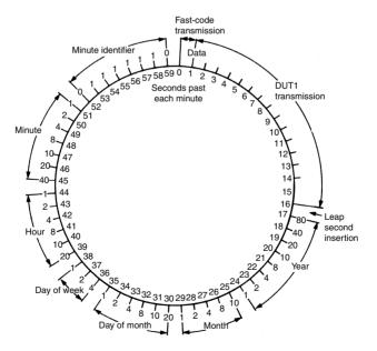
*Slow code* time and date information is transmitted between the 17th and 59th seconds of the minute-long cycle, in normal BCD coding. *Fast code* time and date BCD coded information is inserted into a 500 ms window in the first second of each minute-long cycle, as illustrated below.
