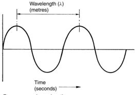
Figure 1.1 Frequency and wavelength
