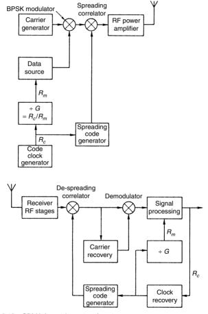
Figure 8.13 CDMA (spread spectrum) system
