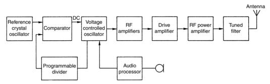
Figure 10.2 Synthesizer controlled FM transmitter
