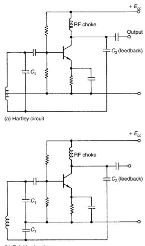
(b) Colpitts circuit **Figure 6.1** Hartley and Colpitts oscillators
