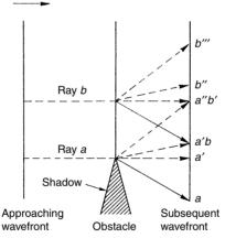
Figure 1.8 Effects of diffraction
