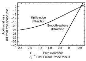
Figure 11.1 Knife-edge and smooth-sphere diffraction
