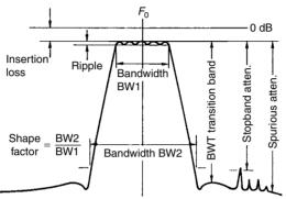
Figure 7.7 Filter characteristics
