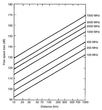
Figure 1.5 Free space loss vs. distance and frequency
