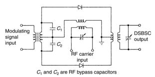
Figure 8.4 Balanced modulator
