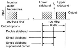
Figure 8.3 Amplitude modulation - sidebands
