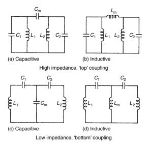
Figure 5.4 Electrical coupling
