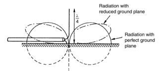
Figure 4.3 Quarter-wavelength vertical radiator
