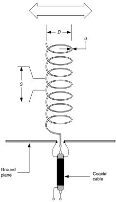
Figure 4.16 Normal mode helix antenna
