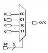
Figure 5-14 Circuit built from the case statement
