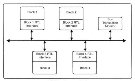
(a) Chip with an on-chip bus
