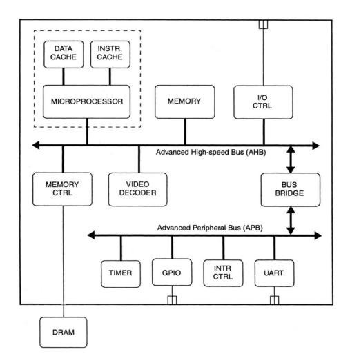
Figure 3-7 Canonical design with ARM on-chip buses
