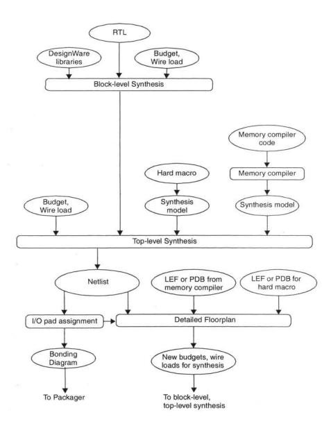
Figure 10-3 Chip-level synthesis
