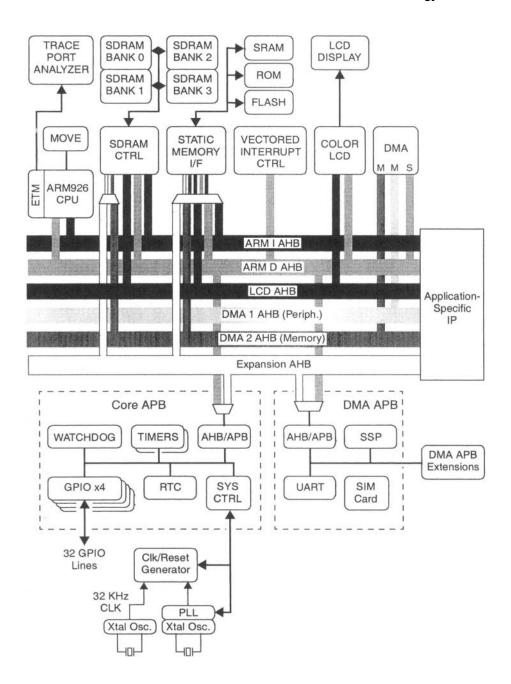
Figure 3-9 Multi-layer AHB System Interface block diagram<sup>1</sup>
