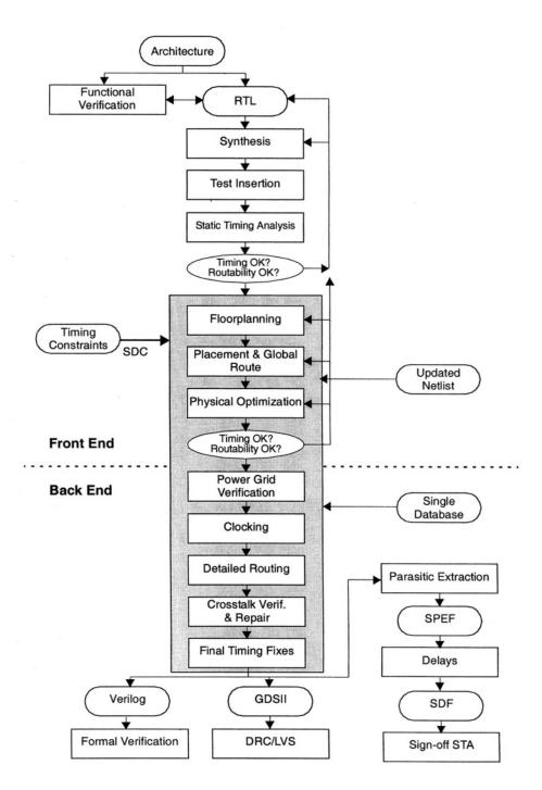
Figure 13-4 LSI Logic's advanced SoC design flow
