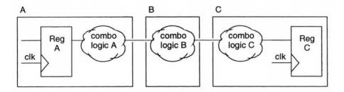
Figure 5-16 Bad example: Combinational logic split between modules
