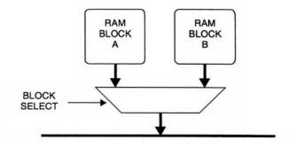
Figure 3-14 Multi-block RAM architecture
