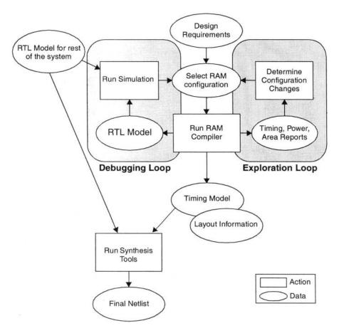
Figure 6-1 RAM generator work flow
