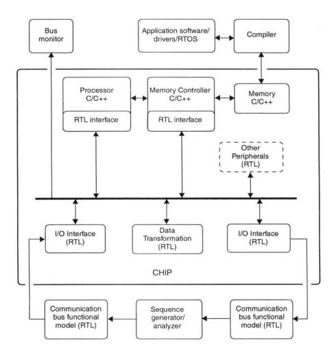
Figure 11-3 System verification environment
