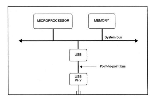
Figure 3-12 Point-to-point connection for a PHY
