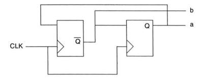
Figure 5-12 Circuit built from blocking and nonblocking assignments
