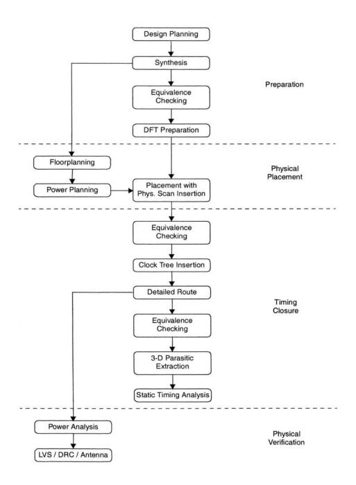
Figure 10-1 Integrating blocks into a chip
