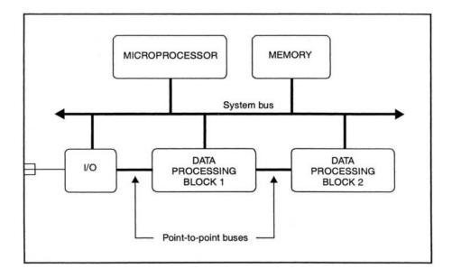
Figure 3-10 Point-to-point connections for system blocks
