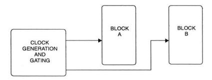
Figure 3-15 Block-level clock gating
