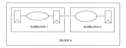
Figure 3-3 Registering outputs of subblocks
