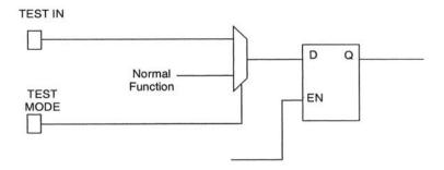
Figure 5-9 Making a latch testable
