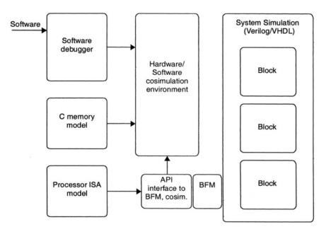
Figure 8-3 Hardware/software cosimulation using an ISA model
