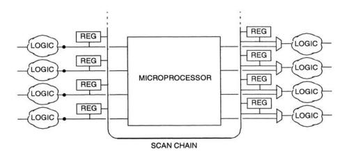
Figure 3-17 Shadow registers for full-scan test logic
