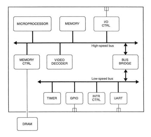
Figure 2-1 Canonical hardware view of SoC
