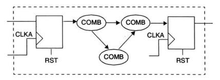
Figure 5-10 Avoiding combinational feedback
