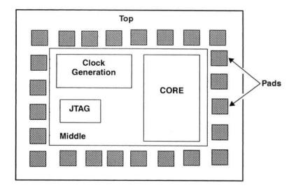
Figure 5-26 Top-level partitioning for an SoC
