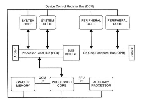
Figure 3-8 CoreConnect block diagram<sup>1</sup>
