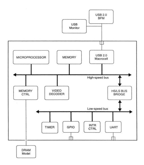
Figure 4-1 SoC verification scheme
