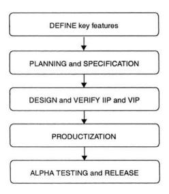
Figure 4-3 Phases of IP design
