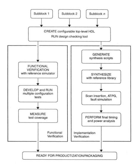
Figure 4-5 Subblock integration process
