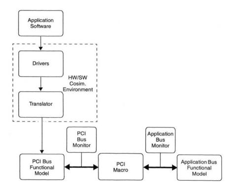
Figure 11-5 Software-driven testbench for macro-level testing
