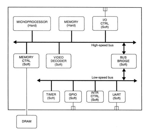
Figure 3-1 Sources of IP for the canonical design
