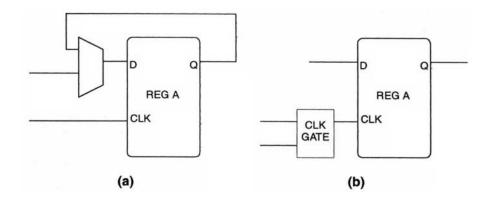
Figure 3-16 Clock gating at individual flip-flops
