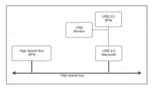
Figure 4-2 USB macro testbench (portion of Figure 4-1)
