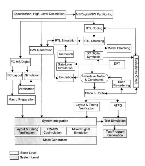
Figure 13-3 Infineon Technologies' SoC design flow
