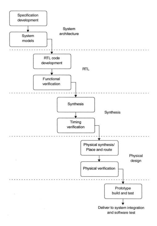
Figure 2-2 Traditional waterfall ASIC design flow
