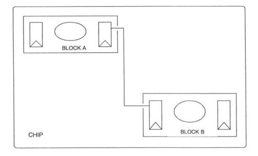
Figure 3-2 Registering inputs and outputs of major blocks
