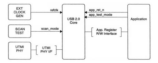
Figure 5-1 USB 2.0 core interfaces
