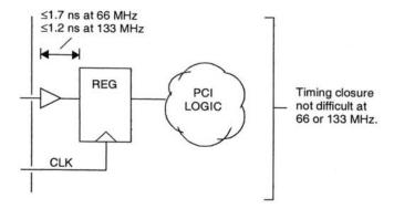
Figure 3-4 Unregistered vs. registered inputs for PCI and PCI-X
