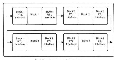
(b) Chip with point-to-point interfaces
