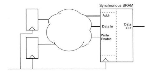
Figure 5-27 Synchronous memory interface
