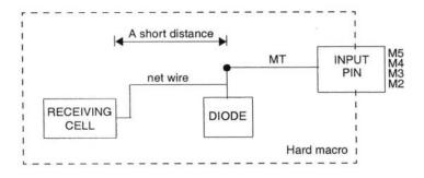
Figure 8-1 Antenna diode insertion for I/O pins
