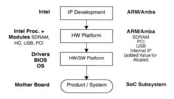
Figure 13-1 Alcatel's SoC design flow
