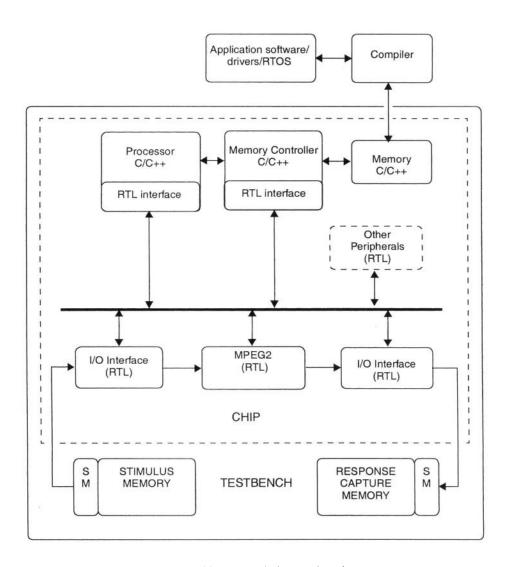
Figure 11-7 Emulation testbench
