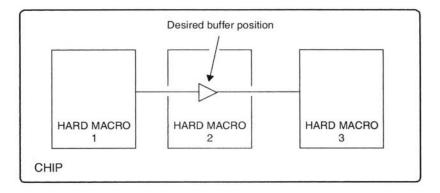
Figure 3-6 Buffer cannot be placed appropriately
