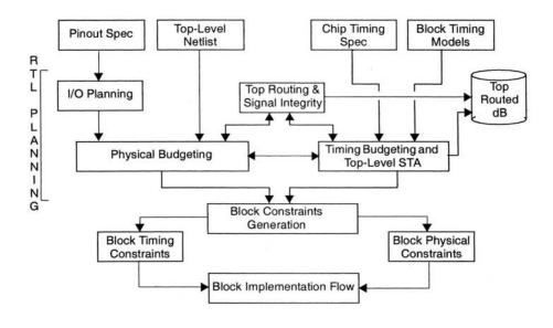
Figure 13-6 STMicroelectronics' design planning steps
