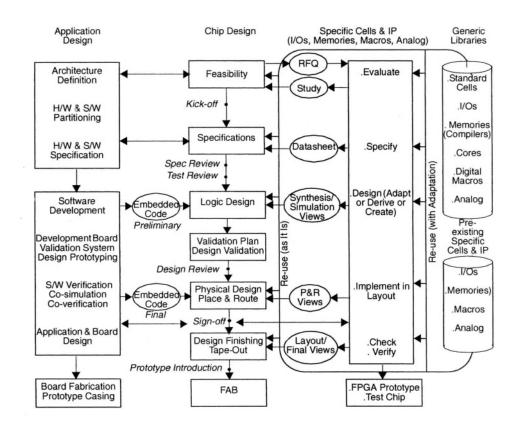
Figure 13-2 Atmel's SoC concurrent engineering SoC flow
