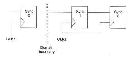
Figure 5-8 Transferring bits between clock domains
