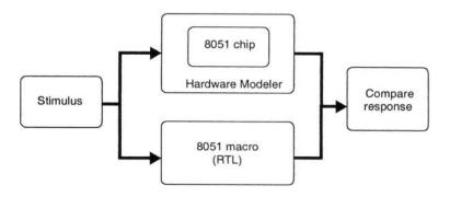
Figure 7-3 Self-checking testbench using a hardware modeler
