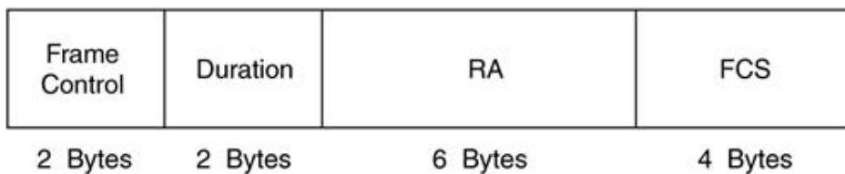
Figure 2-42. Frame Format for the ACK Frame
