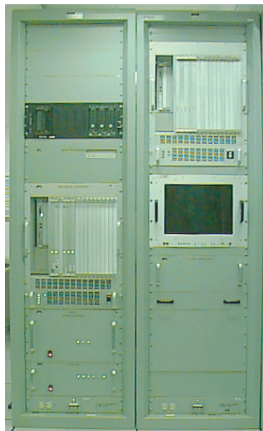
Fig. 9-1. FSPA signal processing equipment: the FSR on the left, and the FSC on the right.
