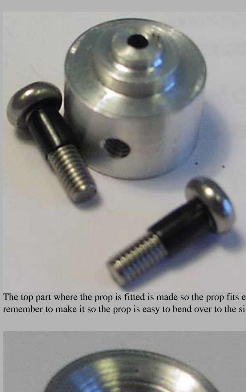
The M3 screws I used are 10mm length
