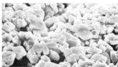
Figure 10-1: Crystalline formation on NiCd cell.
