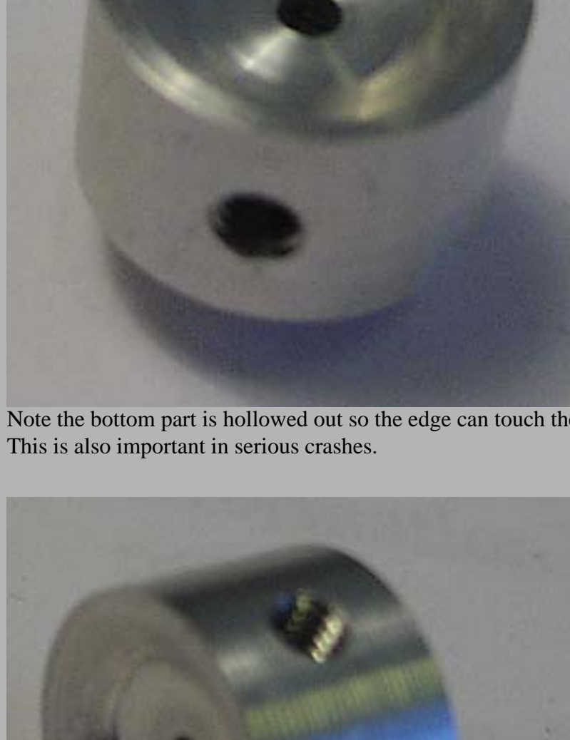
The top part where the prop is fitted is made so the prop fits exactly ! remember to make it so the prop is easy to bend over to the side
