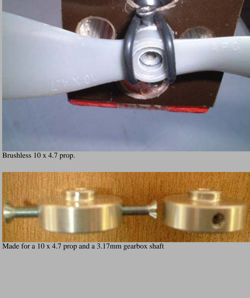
Prop mounting area is 13mm diameter.
