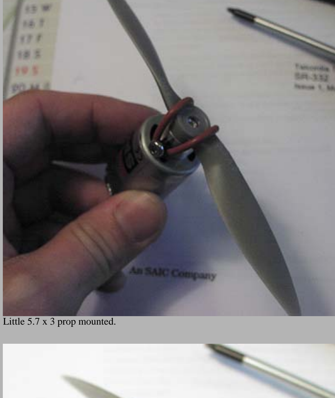
make sure there is a gap from the saver to motor, about 0.2mm
