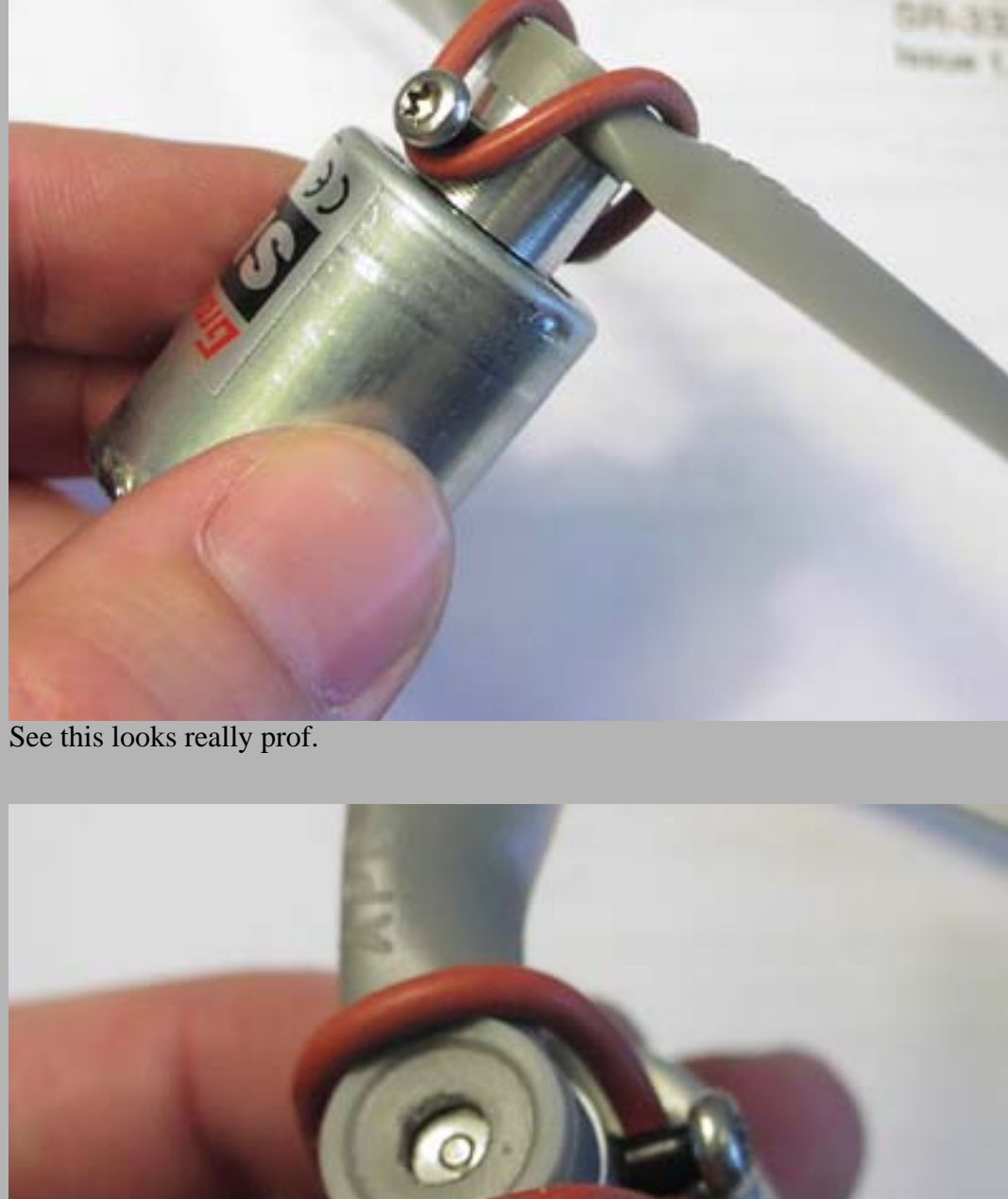
Important: When you press on the saver, it will touch the motor base part, not the bearing.
