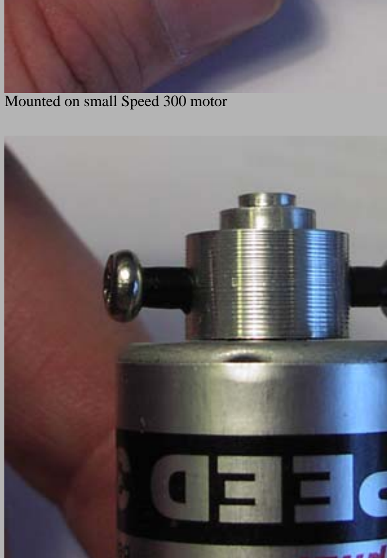
See the plastic tube pressed over the screws, where the thick rubber gasket is mounted.
