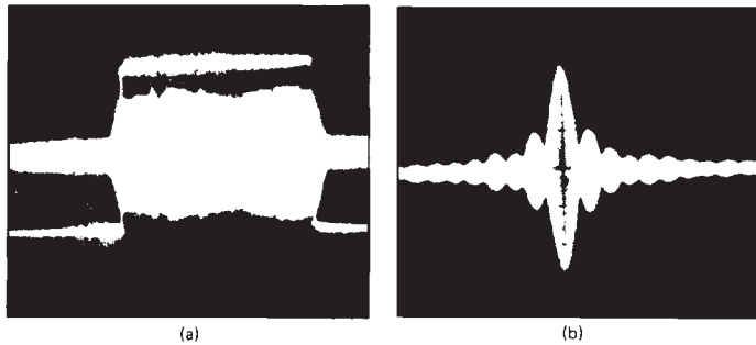
Figure 10.26 Expanded and compressed envelopes for a linear FM dispersive filter: (a) down-chirp linear FM expanded pulse (10- \mu s gate bias), 2.0 \mu s/division, (b) recompressed pulse envelope (spectral inversion), 20 ns/division. (From [10.20]. Reprinted with permission of IEEE.)
