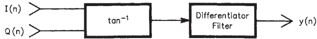
Figure 8.79 FM demodulation can be accomplished by phase detecting the signal using the arc tangent function, and then passing the result through a differentiator. (From [8.60]. Used with permission.)
