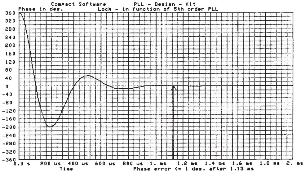
Figure 7.20 Lock-in function of the Type 2, fifth-order loop with a 35^\circ phase margin. Ringing still occurs, but the lock-in time has decreased to 1.13 ms.
