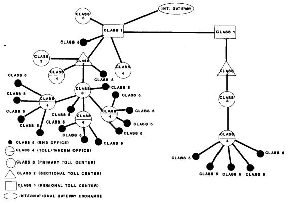
Figure 1.2. Switching system hierarchy
