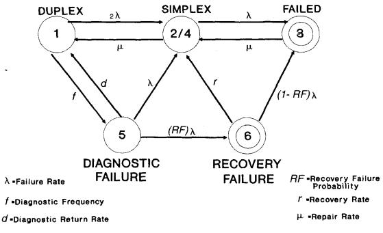
Figure 3.7. Diagnostic and recovery failure models
