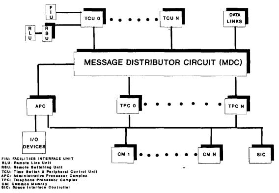
Figure 10.9. GTE GTD-5 EAX switch hardware architecture
