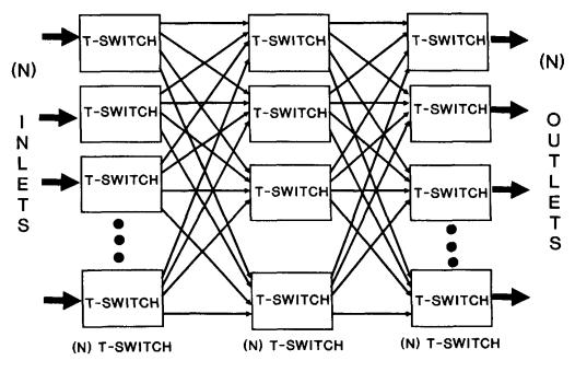
Figure 2.14. Time-time-time (TTT) switching
