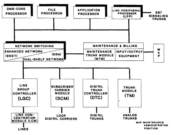
Figure 10.3. NortelDMS-100 switch hardware architecture
