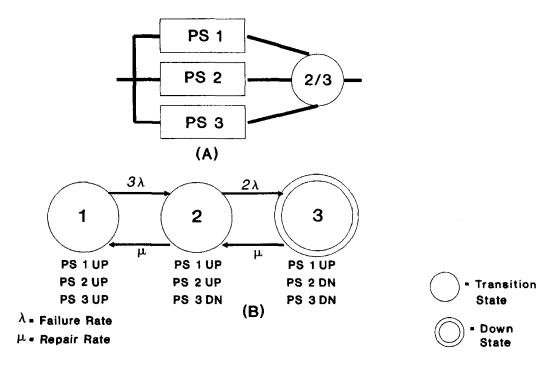
Figure 8.6. Markov model of a STP power supply
