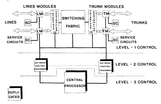
Figure 2.1. Digital switching system—levels of control
