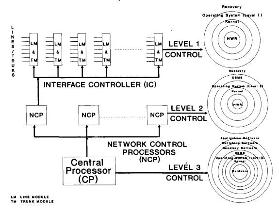
Figure 5.1. Basic software architecture of a typical digital switching system
