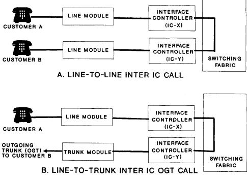
Figure 9.5. Calls between different interface controllers
