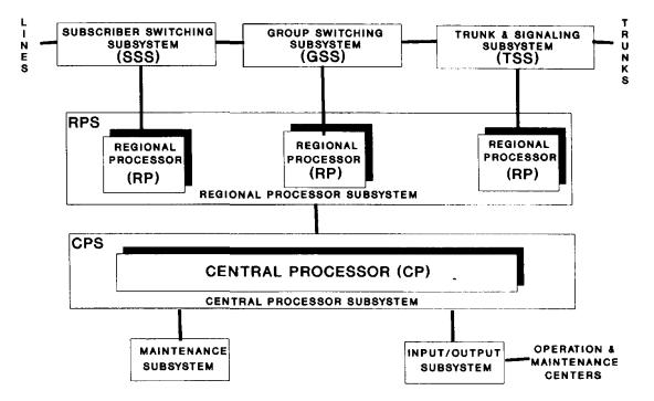
Figure 10.5. EricssonAXE 10 switch hardware architecture
