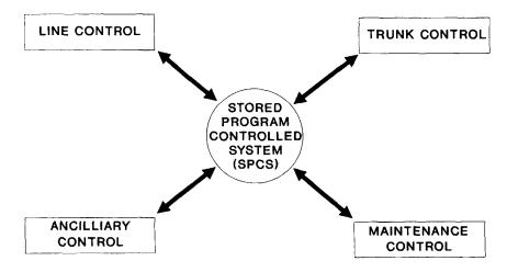
Figure 1.3. Basic control structure of a central office
