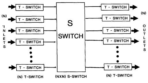
Figure 2.13. Time-space-time (TST) switching
