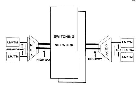
Figure 2.16. Network redundancy
