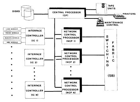
Figure 9.1. A generic switch hardware architecture
