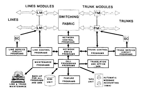
Figure 5.4. Software linkages required during a typical call
