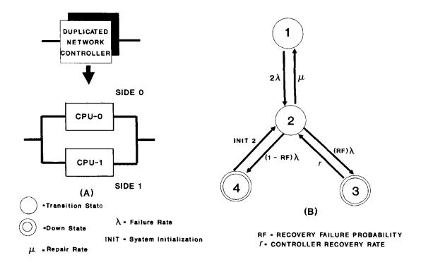
Figure 4.3. Markov model of a network controller
