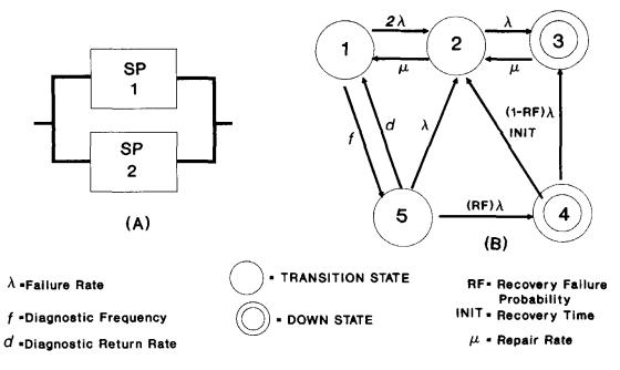
Figure 8.4. Markov model of a STP signal processor
