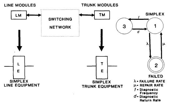
Figure 4.5. Markov model of a line or a trunk
