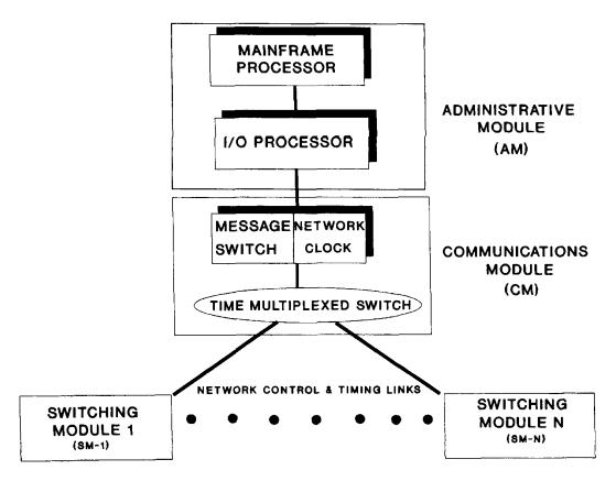
Figure 10.1. Lucent Technologies 5ESS switch hardware architecture
