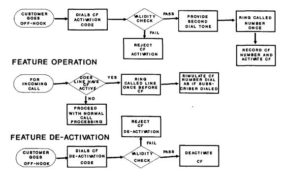
Figure 5.5. Simplified flow diagram for call-forwarding (CF) feature
