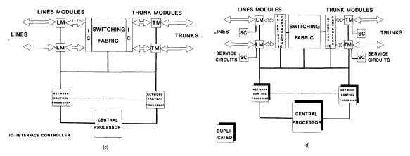
Figure 1.5c Third stage with network control processors
