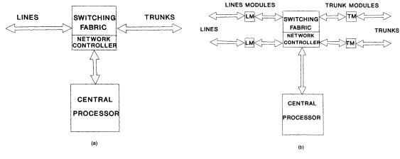
Figure I.5a First stage with lines and trunks
