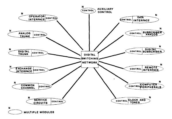
Figure 10-13. Alcatel System 12 switch hardware architecture
