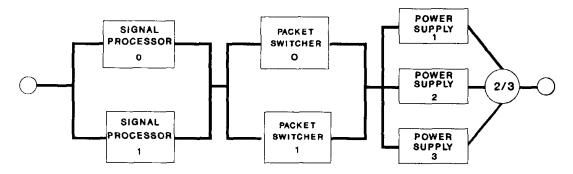
Figure 8.3. Reliability diagram for a sample STP
