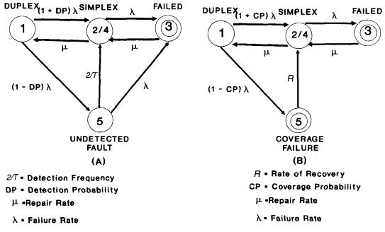
Figure 3.6. Detection and coverage failure models
