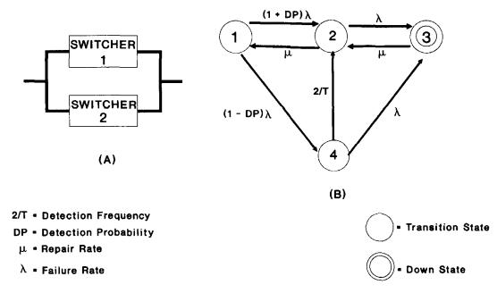
Figure 8.5. Markov model of a STP network packet switcher
