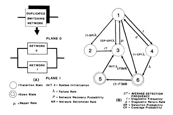
Figure 4.4. Markov model of a switching network
