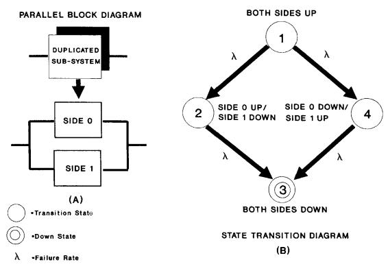
Figure 3.3. Markov model for a duplicated subsystem
