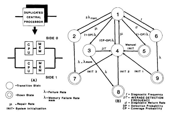
Figure 4.1. Markov model of a central processor
