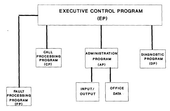
Figure 10.12. NEC NEAX-61 software architecture
