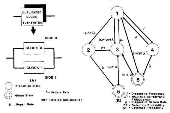
Figure 4.2. Markov model of a clock subsystem
