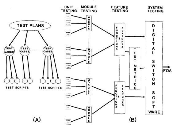
Figure 6.5. A typical digital switch software test methodology
