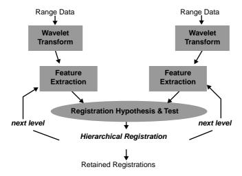
FIGURE 5.4 Block diagram of WaveReg system.
