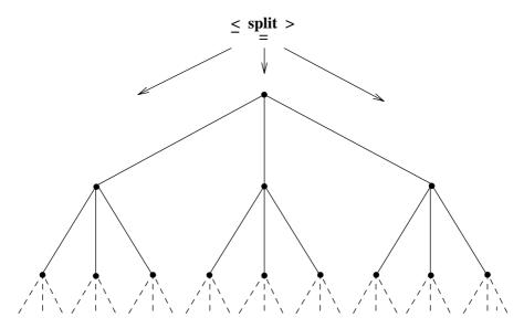
**FIGURE 3.9** Structure of a ternary tree. In a ternary tree, the boxes in the left subtree fall on one side of the partitioning (split) plane; the boxes in the right subtree fall to the other side of the plane; and the boxes in the middle subtree are strictly cut by the plane.
