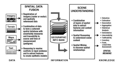
**FIGURE 4.5** The spatial data fusion process flow includes the generation of a spatial database and the assessment of spatial information in the database by multiple users.
