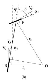
**FIGURE 13.7** The actual experimental vehicle and the "fundamental bicycle model" representation used in the design of the vehicle process model. (A) The host vehicle at the test site with sensor suite. (B) Vehicle kinematics.
