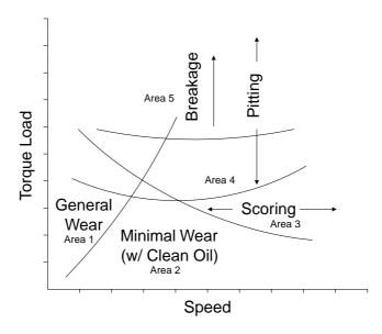
FIGURE 23.7 Regions of gear failures.<sup>35</sup>
