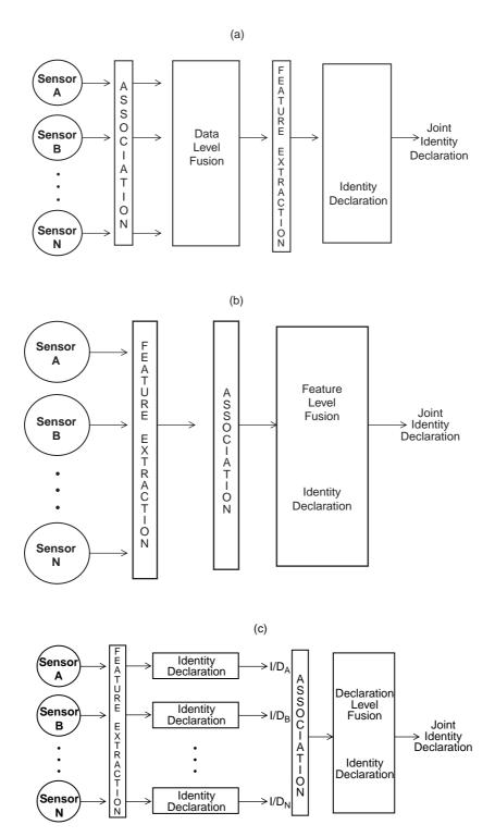
FIGURE 1.4 (a) Direct fusion of sensor data. (b) Representation of sensor data via feature vectors and subsequent fusion of the feature vectors. (c) Processing of each sensor to achieve high-level inferences or decisions that are subsequently combined.
