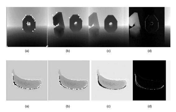
FIGURE 5.6 (a) Features extracted Level 1, Image 1, (b) Features extracted Level 1, Image 2, (c) Merged via averaging registered images, (d) Merged via subtraction of registered images.
