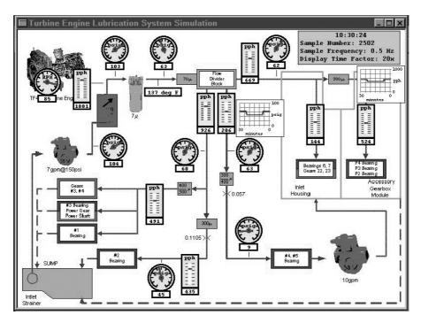
**FIGURE 23.20** TELSS processing of operational data to produce metasensors. Massflow in pounds per hour is shown in bar scaled objects. Pressure throughout the circuit in pounds per square inch is illustrated by pressure gauge objects.
