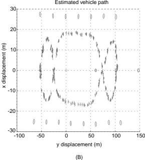
**FIGURE 13.8** The positions of the beacons can be seen in (A) and (B) as the row of ellipses at the top and bottom of the figures.
