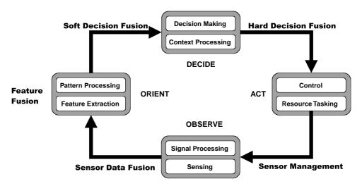
FIGURE 2.12 The "Omnibus" process model.<sup>11</sup>
