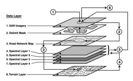
**FIGURE 4.6** Target search example uses multiple layers of spatial data and applies iterative spatial reasoning to evaluate alternative hypotheses while accumulating evidence for each candidate target.
