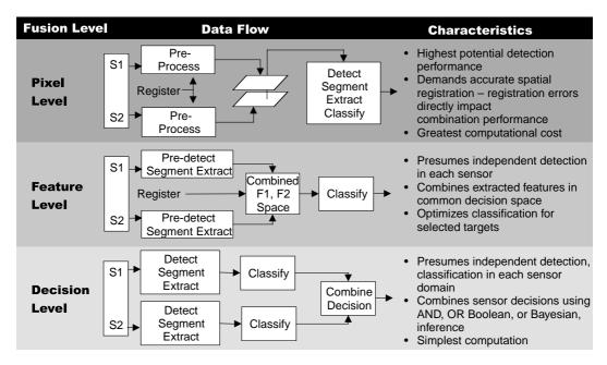
**FIGURE 4.3** Three basic levels of fusion are provided to the multisensor ATR designer as the most logical alternative points in the data chain for combining data.
