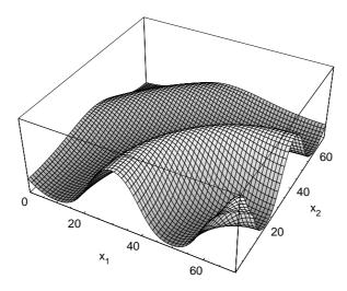
FIGURE 10.1 Detection likelihood function for a sensor at (70,0).
