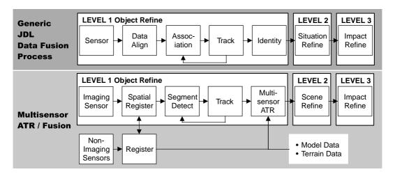
**FIGURE 4.2** Image of a data fusion functional flow can be directly compared to the joint directors of labs (JDL) data fusion subpanel model of data fusion.
