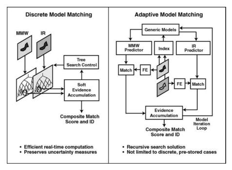
**FIGURE 4.4** Two model-based sensor alternatives demonstrate the use of a prestored hierarchy of model-based templates or an online, iterative model that predicts features based upon estimated target pose.
