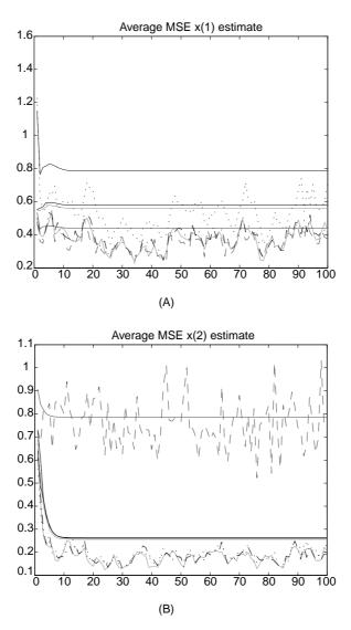
**FIGURE 12.10** Mean squared errors and estimated covariances for all states in each of the four nodes. (A) Mean squared error in x. (B) Mean squared error in  $\dot{x}$ . (C) Mean squared error in  $\ddot{x}$ . The curves for Node 1 are solid, Node 2 are dashed, Node 3 are dotted, and Node 4 are dash-dotted. The mean squared error is the rougher of the two lines for each node.
