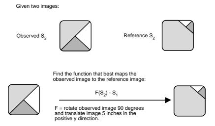
**FIGURE 5.2** Registration is finding the mapping function  $F(S_2)$ .
