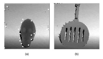
FIGURE 5.5 Features detected, approximate location indicated by white squares: (a) for wavelet Level 2 and (b) for wavelet Level 1.
