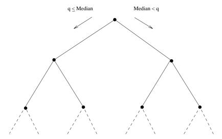
**FIGURE 3.5** Each node in a binary search tree stores the median value of the elements in its subtree. Searching the tree requires a comparison at each node to determine whether the left or right subtree should be searched.
