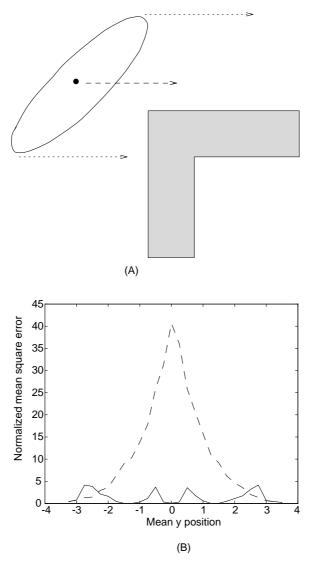
**FIGURE 13.3** A discontinuous system example: a particle can either strike a wall and rebound, or continue to move in a straight line. The experimental results show the effect of using different start values for *y*.
