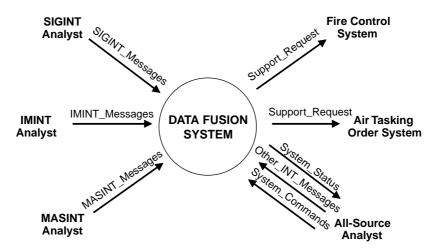
**FIGURE 7.8** The Level 0 diagram establishes the system boundary and clarifies what is considered to be inside or outside the system.
