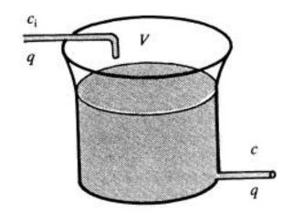
Figure 11.11 A completely mixed tank with a single component.
