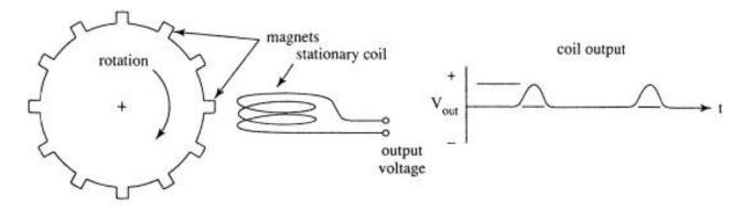
Fig. 1.25 Magnetic sensor
