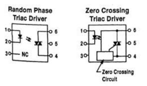
FIGURE 3-38 Electrical diagram of optocouplers specifically designed with triac and zero-crossing triac drivers as the output circuit. (Copyright of Motorola, Used by Permission.)
