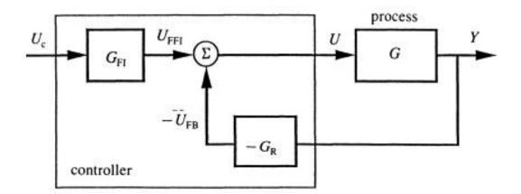
Figure 12.3 Structure of a linear feedforward-feedback controller.
