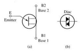
FIGURE 3-8 (a) Electronic symbol of a UJT. (b) Electronic symbol of a diac. These devices are used to fire an SCR.
