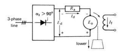
Figure 4-8 Hoist lowering a load.
