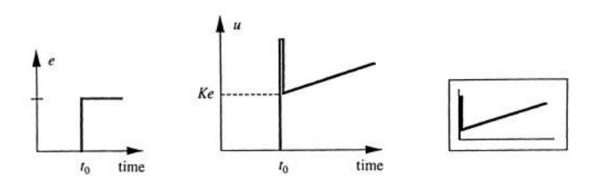
Figure 12.8 The step response of a PID controller and its process scheme symbol. A step change in the error occurs at time to. The part of the controller causes the high peak.
