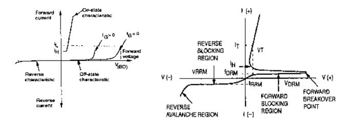
FIGURE 3-4 Static characteristic curve for the SCR. (Courtesy of Philips Semiconductors.)
