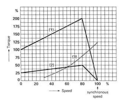
Figure 4-28 Torque-speed curve of blower motor at rated voltage (1) and 50% rated voltage
