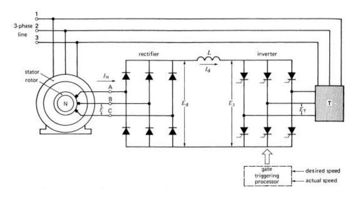
Figure 4-37 Speed control using a rectifier and naturally-commutated inverter.
