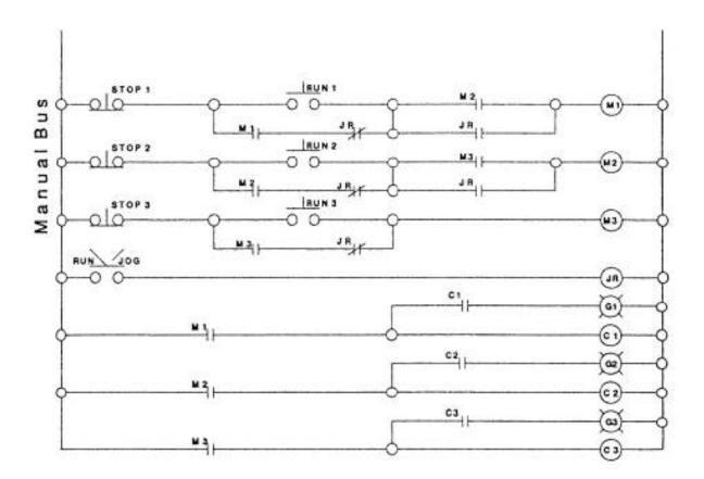
Figure 6-10 Manual-cycle, add jog logic
