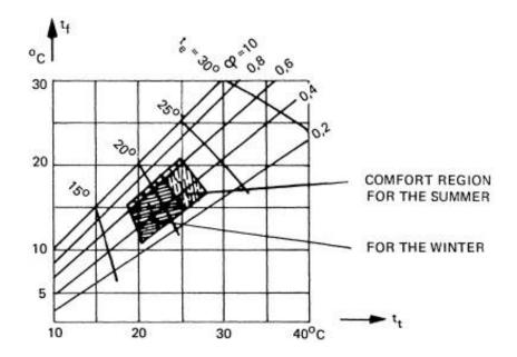
Figure 9-17 Comfort chart: F = relative humidity;  $t_t$  = dry bulb air temperature;  $t_f$  = wet bulb air temperature;  $t_e$  = effective temperature.
