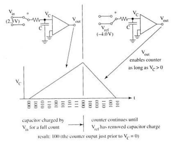
Fig. 8.15 Dual ramp analog to digital conversion
