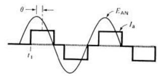
Figure 4-32b Motor voltage and current.
