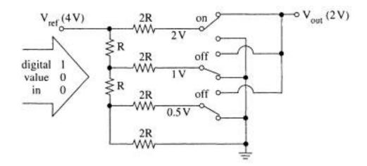
Figure 8-12The R-2R digital to analog conversion circuit
