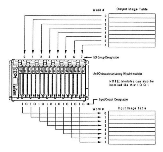
Figure 7-8 I/O addressing scheme
