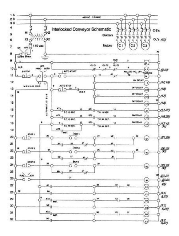
Figure 6-11 Completed conveyor schematic
