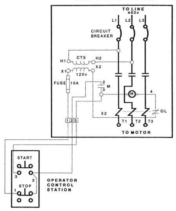
Figure 5-13 Motor starter wiring diagram
