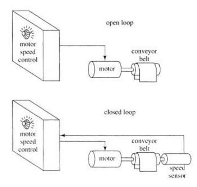
Fig. 0.2 Open loop and closed loop speed control
