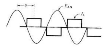
Figure 4-32c Asynchronous generator voltage and current.
