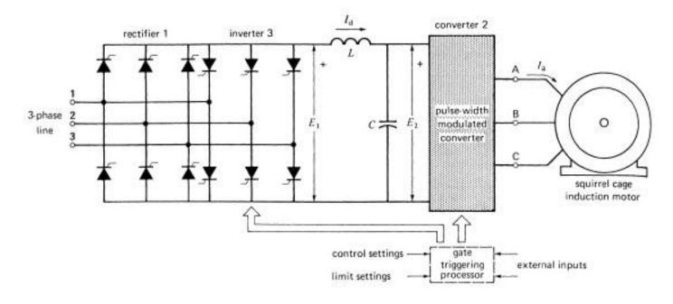
Figure 4-39 Speed control by pulse width modulation.
