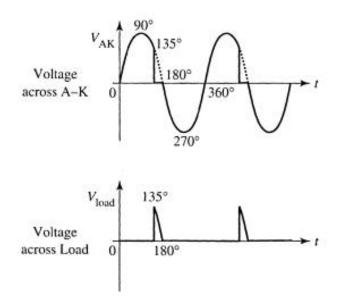
FIGURE 3-5 Waveforms of an ac sine wave applied to an SCR circuit. The top diagram shows the waveform of voltage that is meaured across the anode and cathode of the SCR. The bottom waveform shows the voltage measured across the load. Notice the SCR is fired at 135°.
