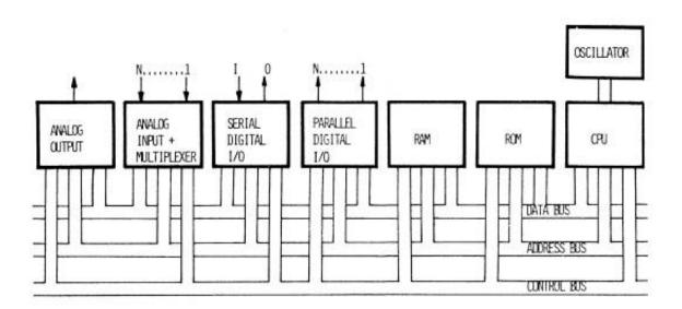
Figure 9-1 Typical microcomputer configuration. (From Ref. 9.)
