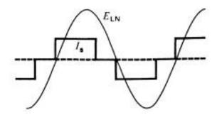
Figure 4-23 Typical voltage and current waveshapes in Fig.4-22.
