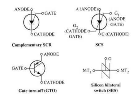
FIGURE 3-12 Electronic symbols for the complementary SCR and the silicon controlled switch (SCS), and the gate turn-off device (GTO). (Copyright of Motorola. Used by Permission.)
