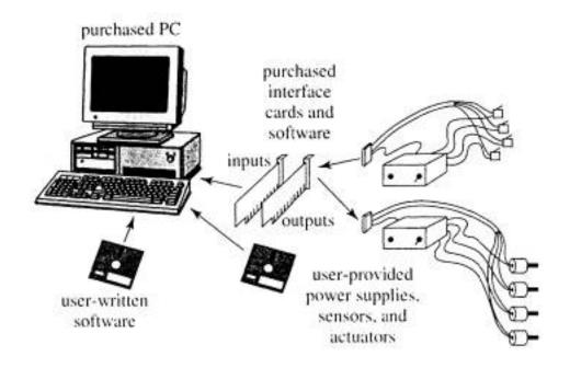
Figure 8-2 A personal computer with peripherals for a control application
