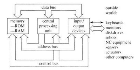
Figure 8-5 Basic computer architecture
