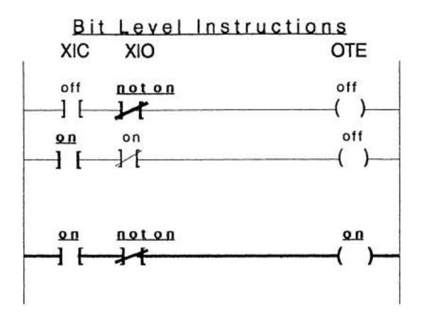
**Figure 7-9 Bit-level instruction logic**
