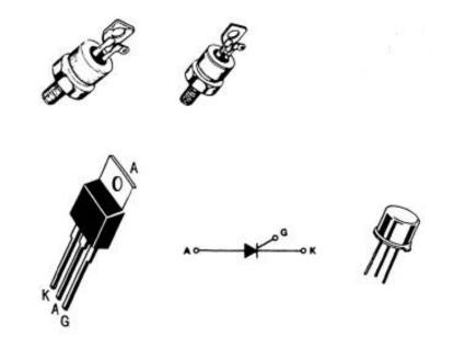
FIGURE 3-1 Examples of SCRs and the electronic symbol of an SCR that identifies the anode, cathode, and gate. (Copyright of Motorola, Used by Permission.)
