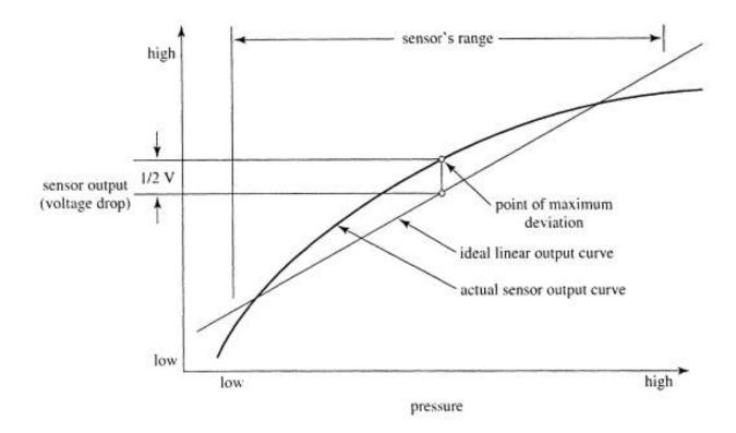
Fig.1. 4 Non-linearity in a pressure sensor
