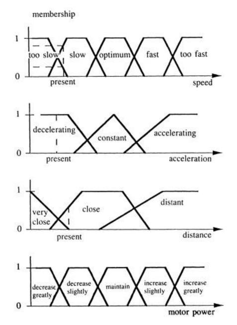
Figure 11.23 Membership functions for a fuzzy speed controller.
