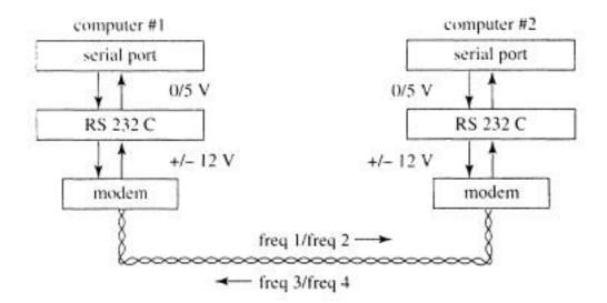
Fig. 8.21 Communication via modems
