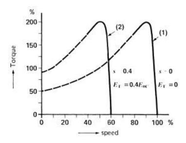
Figure 4-38a Torque-speed characteristics of a wound-rotor motor for two settings of voltage  $E_{\rm T}$ .
