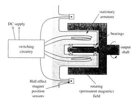
Figure 2-27 Brushless DC servomotor with stationary armature
