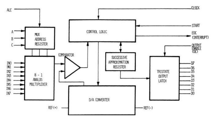
Figure 9-10 An A/D converter with an integrated analog multiplexer. (Courtesy of National Semiconductor GmbH, Furstenfeldbruck, Federal Republic of Germany.)
