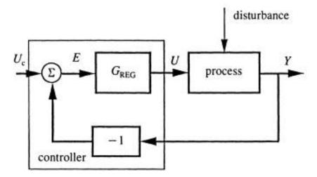
Figure 12.1 The simplest controller structure.
