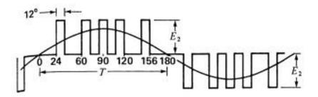
Figure 4-40a Voltage waveform across one phase.
