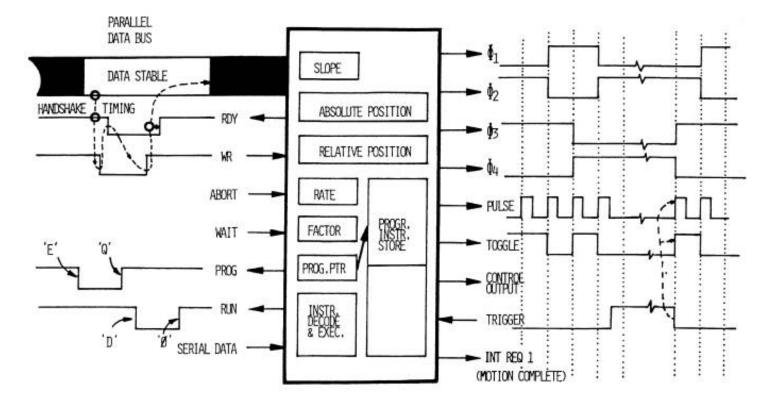
Figure 9-16 The CY500 stepping motor controller.
