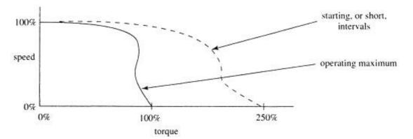
Figure 2-22 Speed/torque relationship for an AC induction motor
