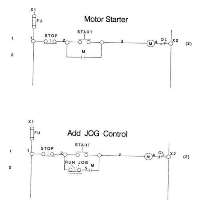
**Figure 5-12 Motor starter schematics**
