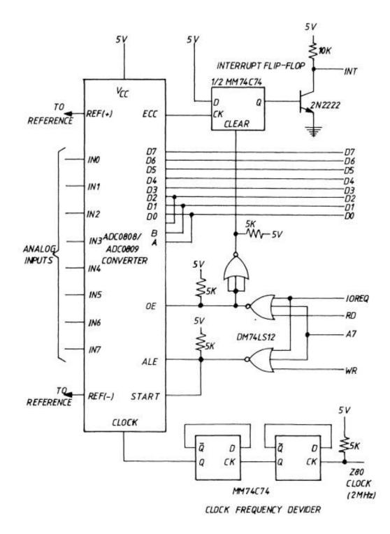
Figure 9-11 An A/C converter with a simple interface. (Courtesy of National Semiconductor GmbH, Furstenfeldbruck, Federal Republic of Germany.)
