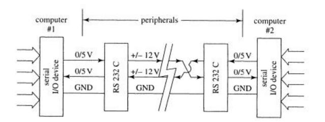
Fig. 8-20 Communication via an RS 232 interface
