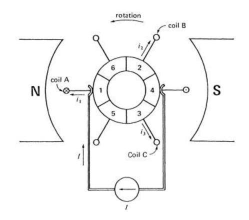
Figure 4-15 Special current-fed dc motor.
