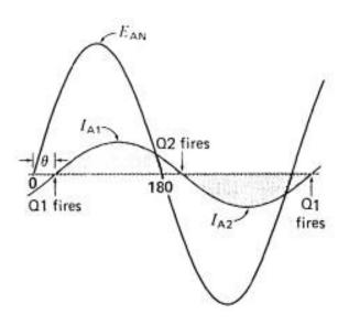
Figure 4-29 Waveshapes at rated voltage.
