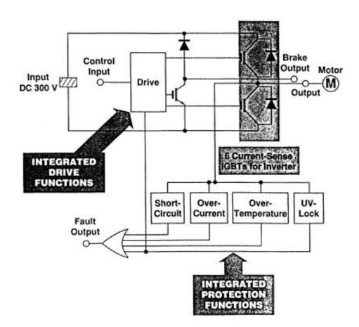
FIGURE 3-22 Block diagram for a circuit that provides IGTBs to sense current in a dc motor drive circuit. The output signal from the IGBTs is sent to protect circuits in the drive. The IGBTs also provide signals that are used for dc braking. (Courtesy of POWEREX Inc.)
