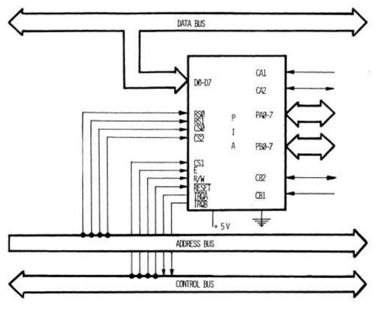
Figure 9-4 Motorola 6820 and 6800 interface. (From Ref. 1.)
