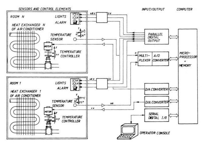
Figure 9-18 Climate control by microcomputer.
