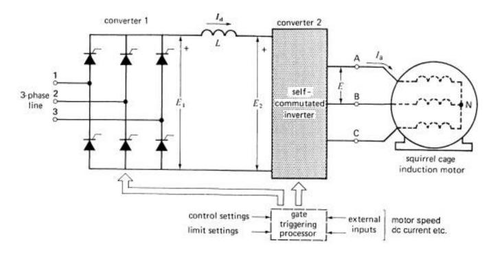
Figure 4-32a Current-fed frequency converter.
