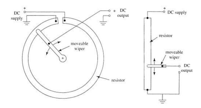
Fig. 1.16 Potentiometric position sensors
