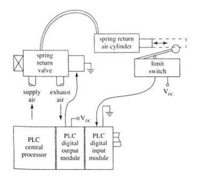
Fig. 0.4 A digital controlled system
