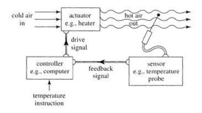
Fig. 0.3 Components of a simple controlled automation system
