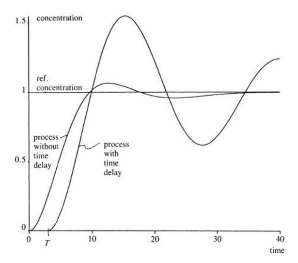
Figure 12.16 A PI control of the chemical dosage with a time delay of 3 time units.
