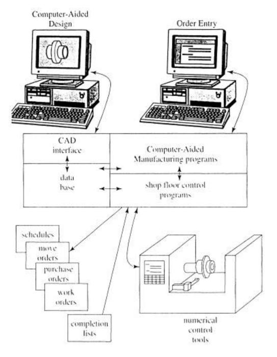
Figure 8-1 A CAD/CAM part production system
