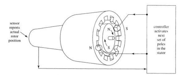
Figure 2-26 DC control and switching in an electronically commutated timing motor
