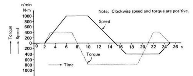
Figure 4-9 Torque-speed characteristic of an industrial drive.
