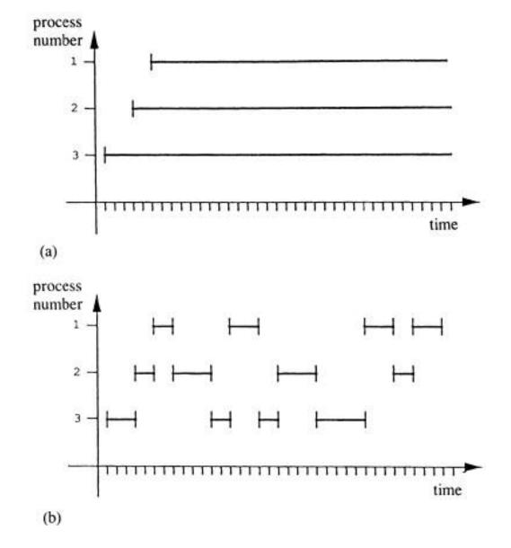
Figure 10-3 the principle of multitasking, (a) Macroscopic effect; (b) CPU time division.
