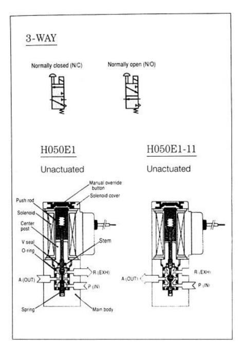
Figure 2-8 Air control valves: spring-return two- and three-way. (Photographs and diagrams by permission, Humphrey Products Company, Kalamazoo, Michigan.)
