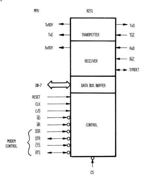
Figure 9-6 INTEL 8251 USART. (Courtesy of SYBEX, Berkeley, California.)
