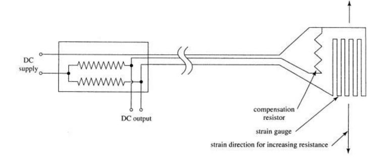
Fig. 1.13 Strain gauges and compensation circuitry
