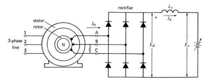
Figure 4-36 Speed control using a variable-voltage battery.
