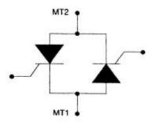
FIGURE 3-14 Two SCRs connected in inverse parallel configuration to provide the equivalent circuit for a triac.
