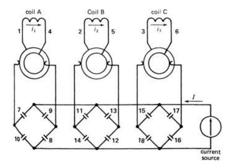
Figure 4-17 The commutator can be replaced by an array of mechanical switches and a set of slip rings.
