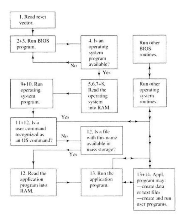
Figure 8-8 Flowchart of CPU operations from startup
