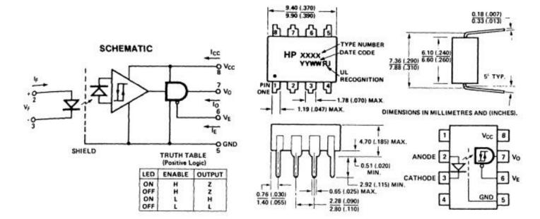
FIGURE 3-33 Schematic diagram and pin outline for a low-power optocoupler. This type of device is used where the input signal is a low-power signal. (Copyright of Motorola, Used by Permission.)
