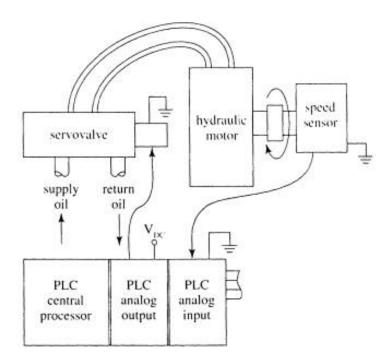
Fig. 0.5 An analog controlled system
