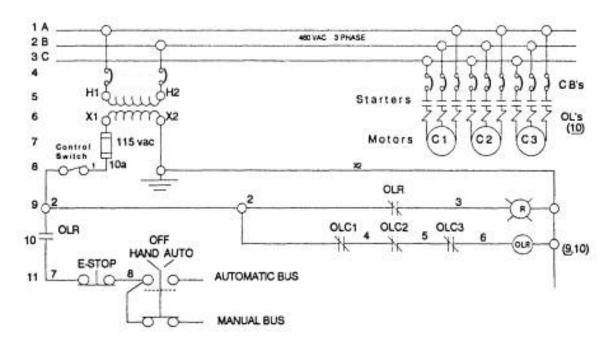
Figure 6-3 Power and Safety logic
