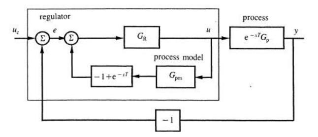
Figure 12.17 Block diagram of the Smith controller.
