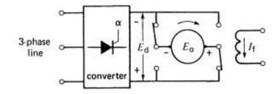
Figure 4-3 Motor control by armature reversal.
