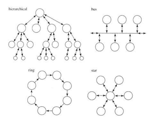
Fig. 8.22 Communication network architecture: hierarchical; bus; ring; star.
