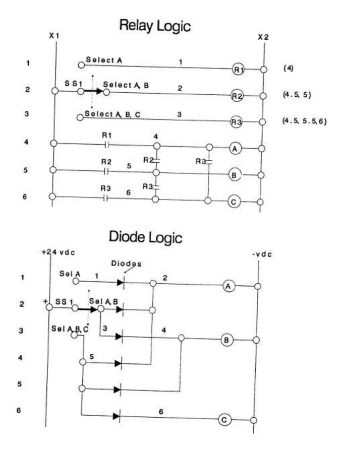
Figure 5-15 Compare relay and diode logic
