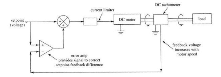
Figure 2-20 A motor with its speed controlled by a servosystem
