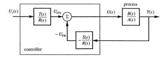
Figure 12.4 The feedforward feedback controller corresponding to Figure 12.3.
