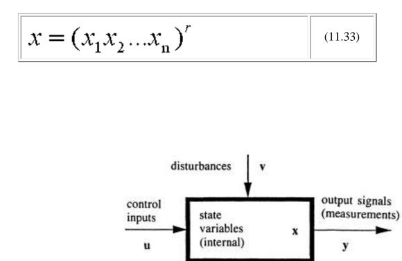
Figure 11.15 Block diagram of a controlled system.
