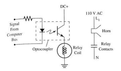
FIGURE 3-27 Electrical diagram of an optocoupler used to interface an annunciator horn to a computer. The relay coil is connected to the output stage of the optocoupler.
