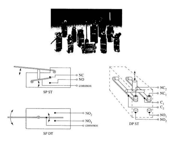
Fig.1.6 Limit switches. (Photograph by permission, Allen-Bradley Canada Ltd., A Rockwell International Company)
