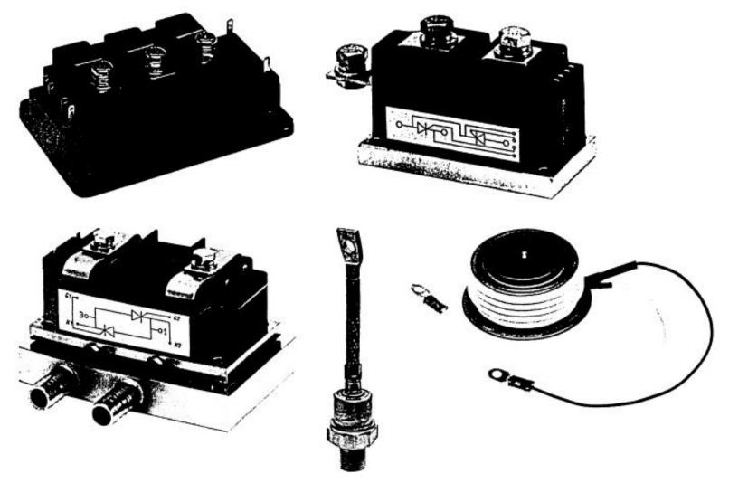
FIGURE 3-10 Typical SCR packages. Notice that the terminals are larger for larger-sized wire required to carry the currents. If more than one SCR is mounted in a package, they are connected internally as pairs so the module is easy to install. (Courtesy of Darrah Electric Company, Cleveland, Ohio.)
