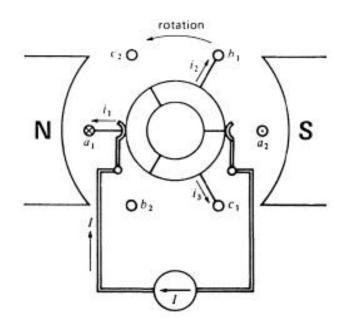
Figure 4-21 This elementary dc motor is equivalent to the entire circuit of Fig.4-20.
