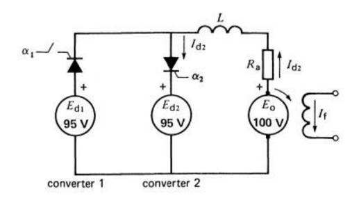
Figure 4-5b Converter 2 in operation, converter 1 blocked.
