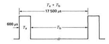
Figure 4-13b Current pulses I<sub>s</sub> drawn by the chopper from the 700V source when the motor is stalled.
