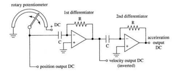
Fig. 1.24 Position sensor and op-amps for velocity and acceleration output
