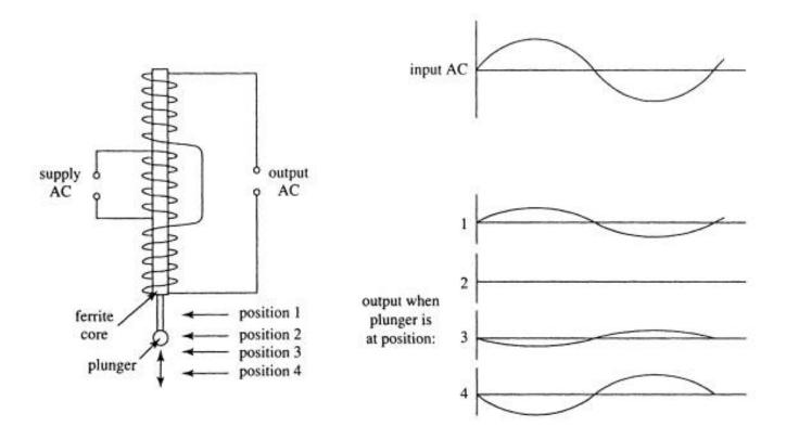
Fig. 1.18 The magnetostrictive position sensor. (By permission, Deem Controls Inc., London, Ontario, Canada.)
