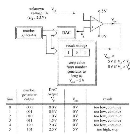
Figure 8-13 Ramp analog to digital conversion
