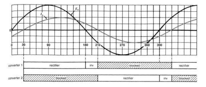
Figure 4-26 Operating mode of converter 1 and converter 2 when current I<sub>a</sub> lags 30° behind  $E_a$ .
