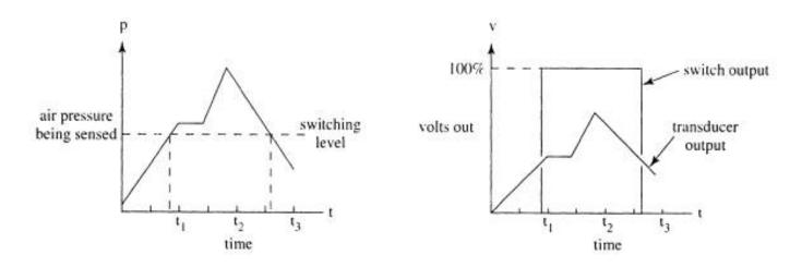
Fig. 1.5 Switch output versus transducer output (switch without hysteresis)
