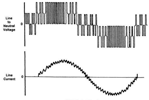
PWM Output Waveforms
