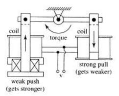
Figure 2-4 Electromagnetic torque motor
