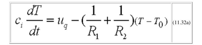
A large temperature difference across the walls will cause a rapid temperature change. If the thermal resistances are large then the temperature rate of change will be dampened.
