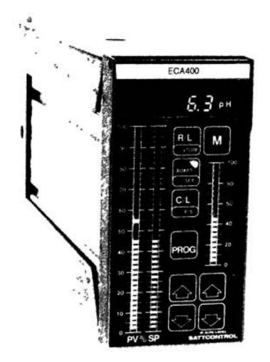
Figure 12.13 An industrial PID controller. (Courtesy of SattControl, Sweden).
