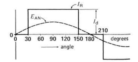
Figure 4-38b Rotor voltage and current in Fig. 4-35.
