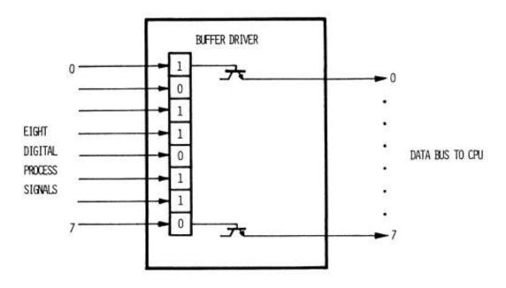
Figure 9-2 Principle of parallel data input.
