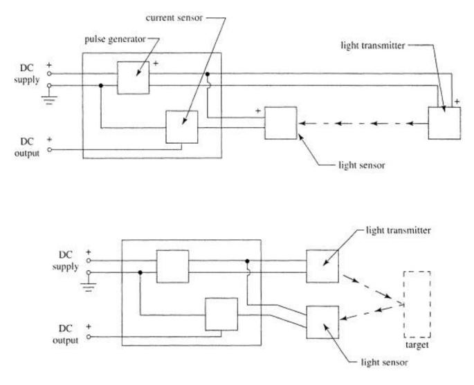
Fig. 1.10 Optical proximity sensors.
