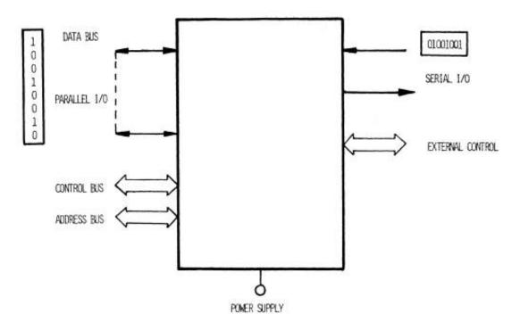
Figure 9-5 Serial digital I/O. (From Ref. 9.)
