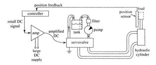
Fig. 0.7 Hydraulic actuated position control
