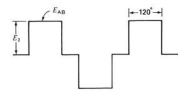
Figure 4-33b Motor line-to-line voltages.
