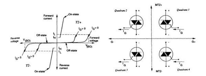
FIGURE 3-15 (a) A graph of the positive and negative voltage and current characteristics of a triac. (b) The four quadrants identified for the graph to describe the voltage polarity of the triac when it is in conduction. (Courtesy of Philips Semiconductors.)
