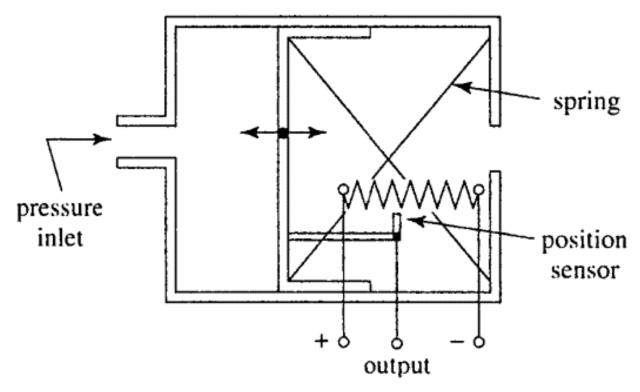
Fig. 1.12 A spring-type pressure sensor
