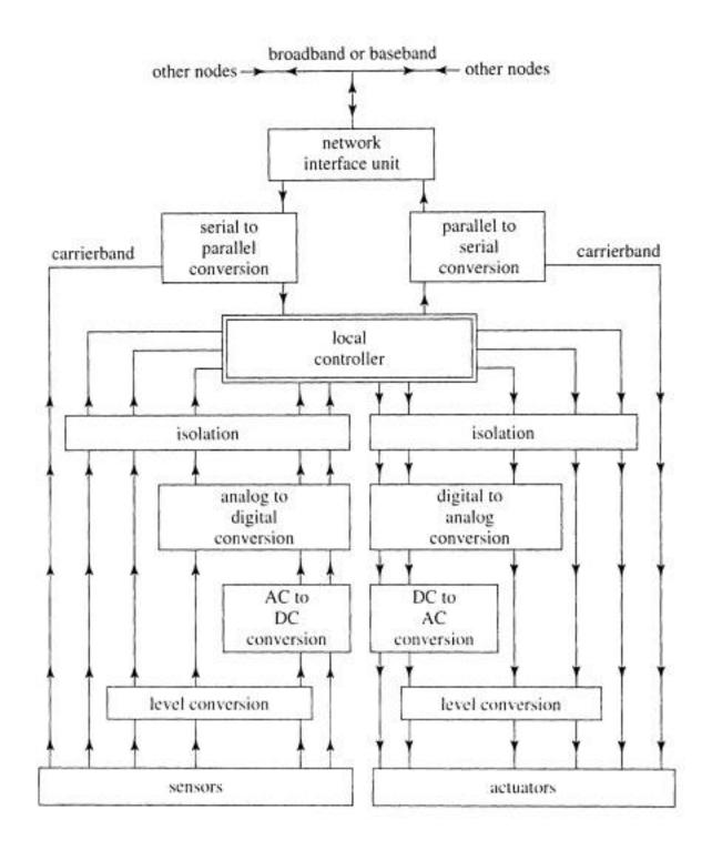
Figure 8-9 I/O interfacing requirements of a local controller
