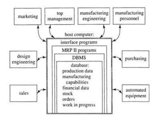
Figure 8-4 Central controller: database, programming, and networking
