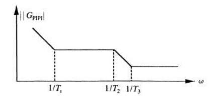
Figure 12.10 The Bode plot gain of the PIPI controller.
