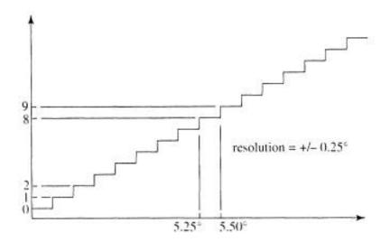
Fig.1. 3 Resolution in a digital temperature sensor output numbers representing temperature step input (temperature)
