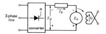
Figure 4-2 Motor control by field reversal.
