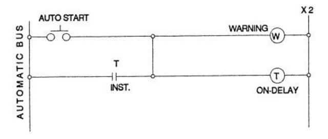
Figure 6-4 Auto-cycle warning circuit logic
