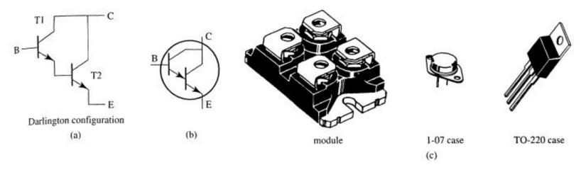
FIGURE 3-20 (a) Internal configuration for a darlington transistor pair. This diagram shows transistor T1 as the driver of transistor T2, which is the output for the darlington. (b) Electronic symbol for the darlington transistor. (c) Typical packages for the darlington transistor including the module, 1-07 case, and the TO-220 case. (Courtesy of Philips Semiconductors.)
