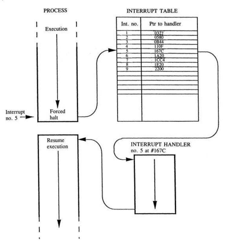
Figure 10-10 Interrupt handling procedure.
