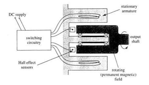
Figure 2-28 Brushless DC servomotor turned inside out
