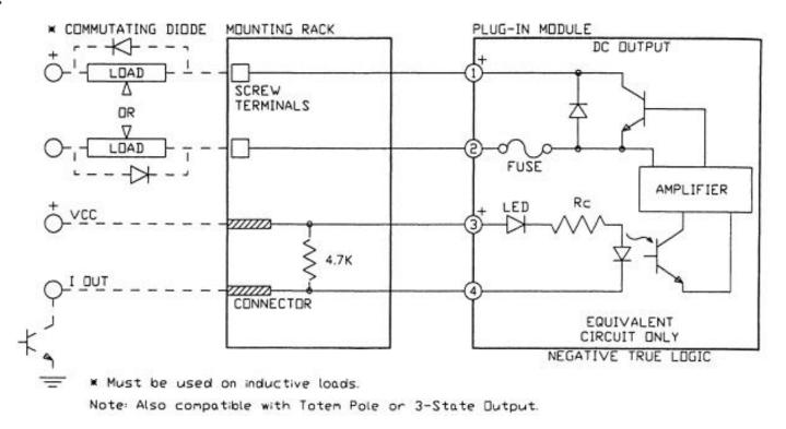
FIGURE 3-32 Electrical diagram of the solid-state relay used as an output module. Notice that the output circuit includes an optocoupler and a transistor that is used as an amplifier. (Courtesy of Opto 22, Remecula, CA.)
