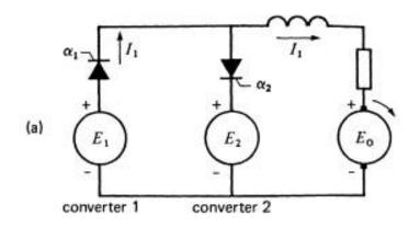
Figure 4-11a Polarities when the speed is positive.
