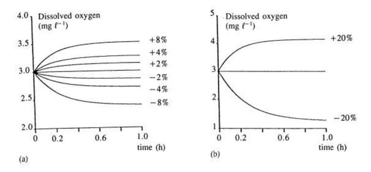
Figure 11.17 Changes of the dissolved oxygen concentration in an aerator system when the air flow has been changed as a step at time 0. Different air flow step sizes have been applied, (a) 2 per cent, 4 per cent and 8 per cent; (b) 20 per cent.
