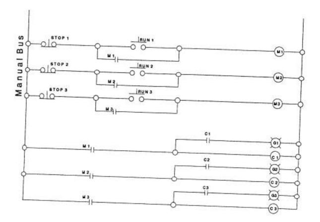
Figure 6-8 Manual-cycle conveyor run logic
