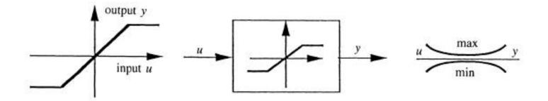
Figure 11.16 An actuator with limitation (and its symbols).
