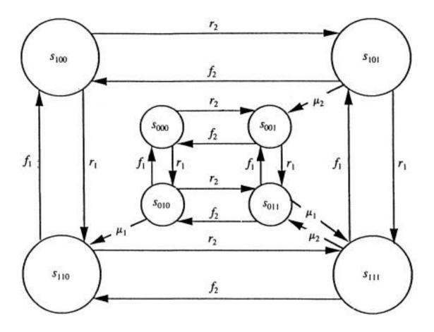
Figure 11.25 A state graph of the transfer line.
