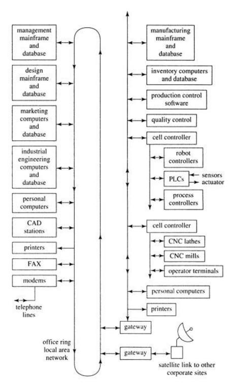
Fig. 0.1 A computer integrated manufacturing environment
