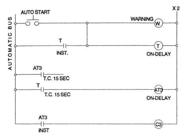
Figure 6-5 Auto-cycle, add first conveyor start logic
