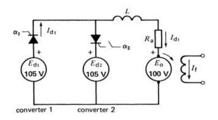
Figure 4-5a Converter 1 in operation, converter 2 blocked.
