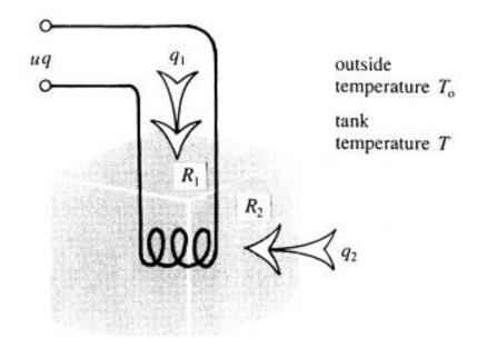
Figure 11.14 A thermal balance system.
