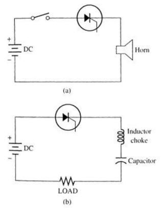
FIGURE 3-9 (a) A switch is used to commutate the SCR in a dc circuit by interrupting current flow. This type of circuit is used to provide control in alarms or emergency dc voltage lighting circuits, (b) A series RL resonant circuit use to commutate an SCR. (c) A parallel RL resonant circuit used to commutate an SCR.
