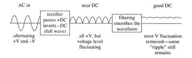
Fig. 8.18 Rectification and filtering of an AC signal
