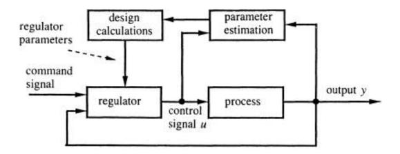
Figure 12.20 The principal parts of an adaptive controller.
