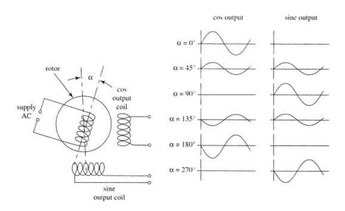
Fig. 1.21 The rotary resolver
