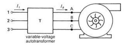
Figure 4-27 Variable-speed blower motor.
