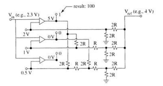
Fig. 8.17 The economical analog to digital converter
