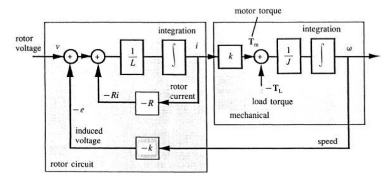
Figure 11.10 Block diagram of the d.c. motor.
