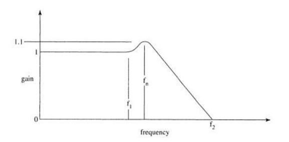
Fig. 1.29 Frequency response of an accelerometer (Bode diagram)
