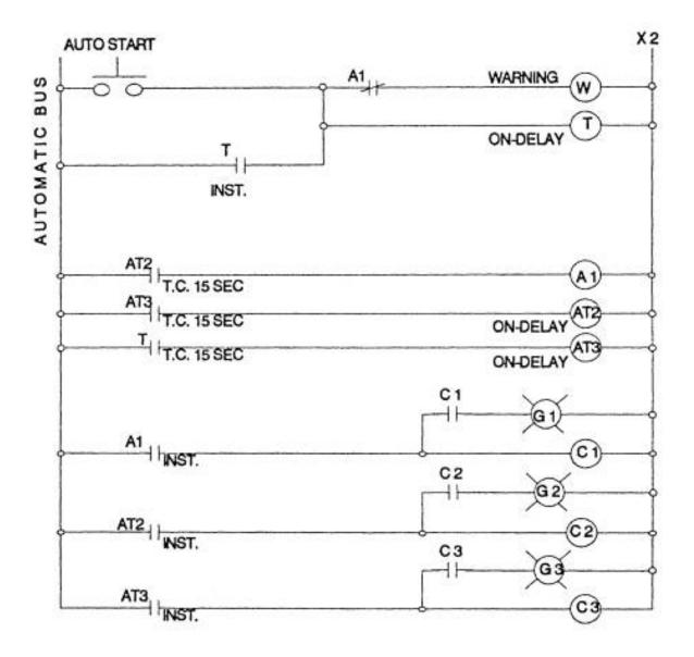
Figure 6-6 Auto-cycle, complete conveyor start logic
