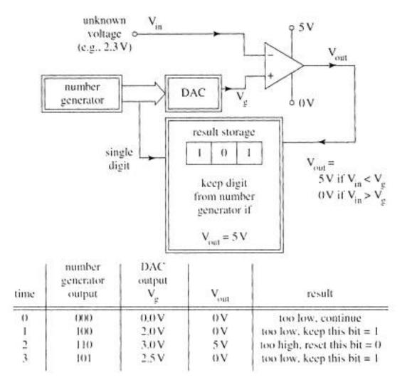
Fig. 8.14 Successive approximation analog to digital conversion
