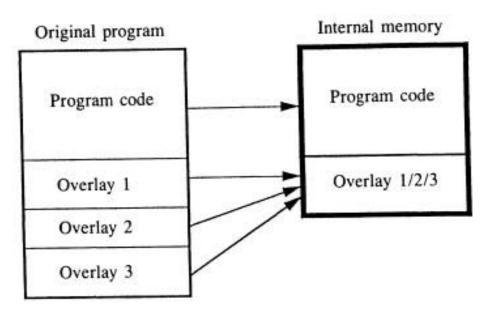
Figure 10-5 Use of program segments and overlays.
