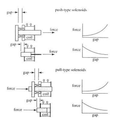
Figure 2-3 Push and pull solenoids and force/displacement characteristics
