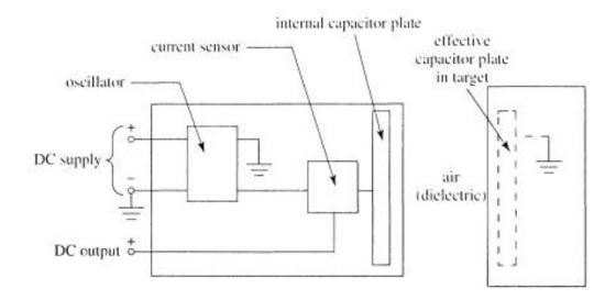
Fig.1. 9 Capacitive proximity sensors.
