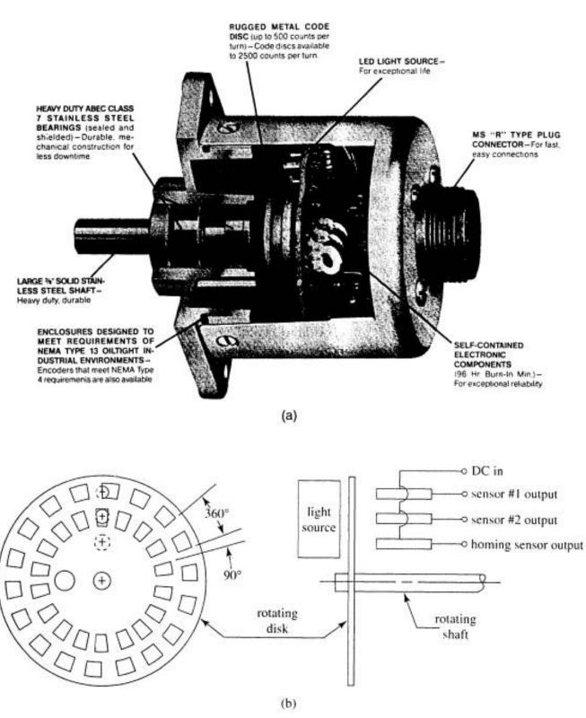
Fig. 1.22 The incremental optical encoder, (a) Cutaway view of encoder; (b) the etched disk.
