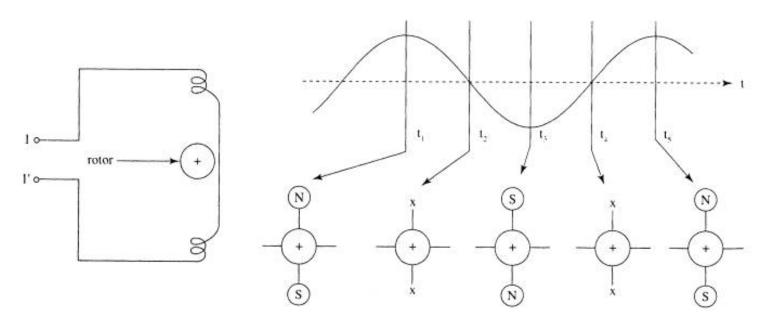
Figure 2-23 Single phase AC showing alternating magnetic field
