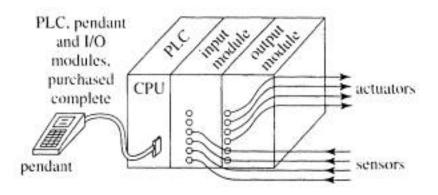
Figure 8-3 A PLC as a cell controller
