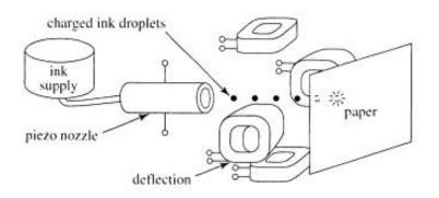
Figure 2-1 Piezoelectrics in ink jet printers
