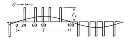
Figure 4-40b Waveform yielding the same frequency but half the voltage.
