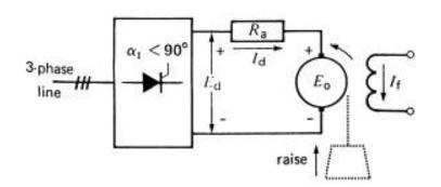
Figure 4-7 hoist raising a load.
