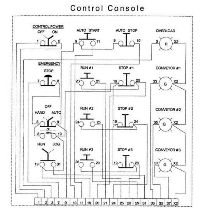
Figure 6-19 Control console wiring diagram
