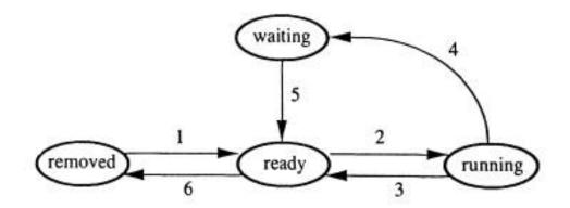
Figure 10-4 The states of a process.
