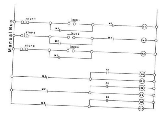
Figure 6-9 Manual-cycle, add stop sequence logic
