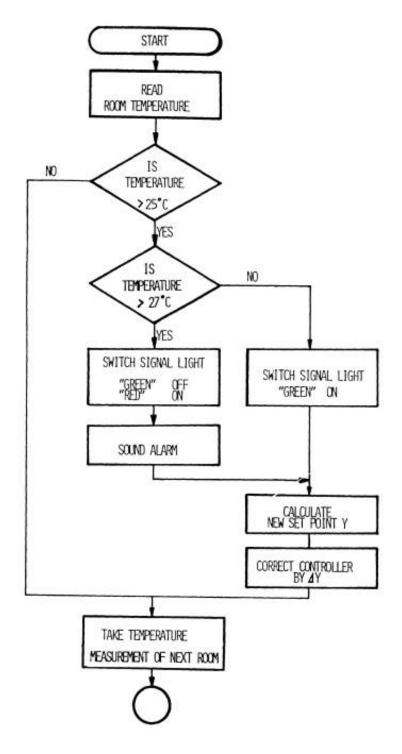
Figure 9-19 Program module "temperature measurement".
