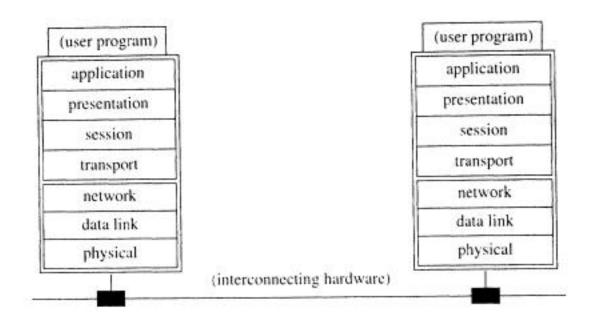
Fig. 8.23 OSI seven layer model
