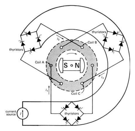
Figure 4-19 The armature is now the stator, and the switches have been replaced by thyristors.
