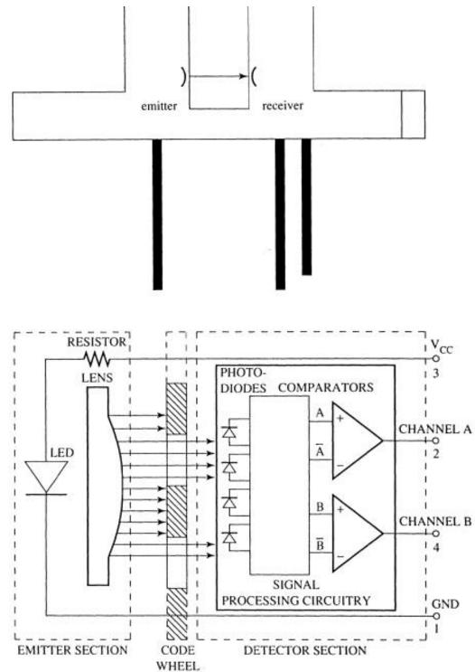
FIGURE 3-39 Drawing and electrical diagram of a photo- interrupter used to detect data from punch cards or other similar media as it moves through the slot in the head where the sender and receiver are mounted. (Courtesy of Hewlett Packard Company.)
