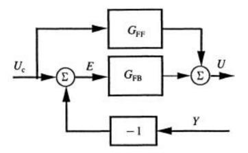
Figure 12.2 A regulator made up by a feedforward loop from the command signal and a feedback loop from the process output.
