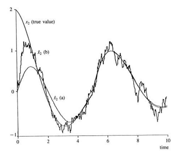
Figure 11.22 Velocity estimation with noisy position measurement. (a) K, = 1, K<sub>2</sub> == 0.4; (b) K, = 5, K<sub>2</sub>= 8.4.
