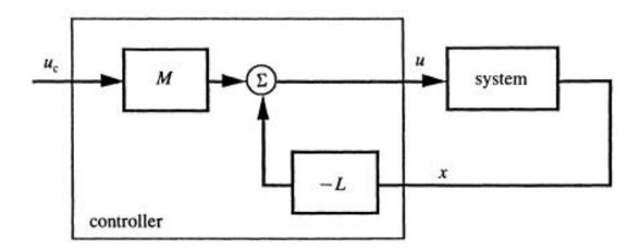
Figure 12.22 Structure of the state feedback controller.
