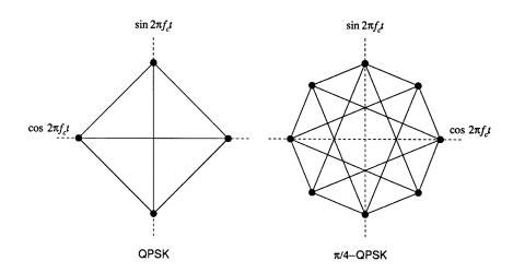
FIGURE 16.2: Signal-space constellations for QPSK and  $\pi/4$ -DQPSK.
