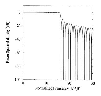
FIGURE 16.10: Power density spectrum of OFDM with N = 32.
