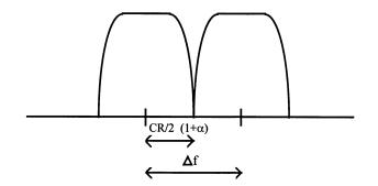
FIGURE 36.2: Relationship between chip rate (CR), roll-off factor ( $\alpha$ ), and channel separation ( $\Delta$ f).
