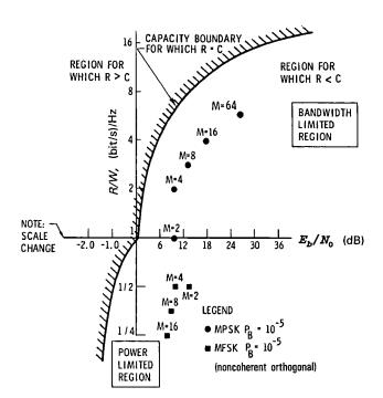
FIGURE 13.1: Bandwidth-efficiency plane.
