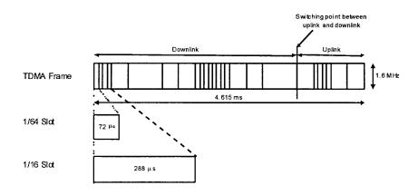
FIGURE 36.13: Wideband TDMA frame and slot structure.
