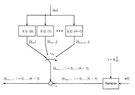
FIGURE 7.4: A set of *m* interleaved echo cancellers.
