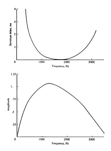
FIGURE 5.2: Average amplitude and delay characteristics of medium-range telephone channel.
