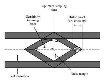
FIGURE 5.7: Effect of intersymbol interference on eye opening.
