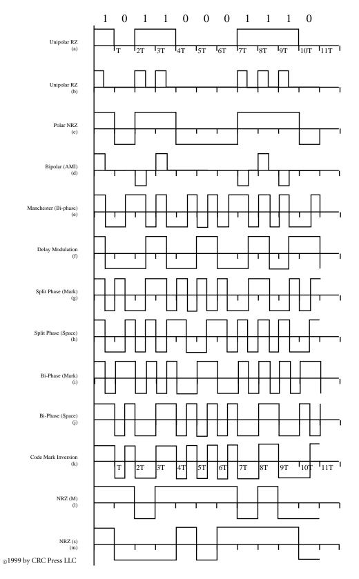
FIGURE 6.1: Waveforms for different line codes.
