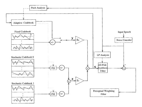
FIGURE 30.2: Basic structure of the PSI-CELP encoder.
