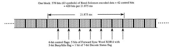
FIGURE 33.7: Cellular digital packet data forward link block structure.
