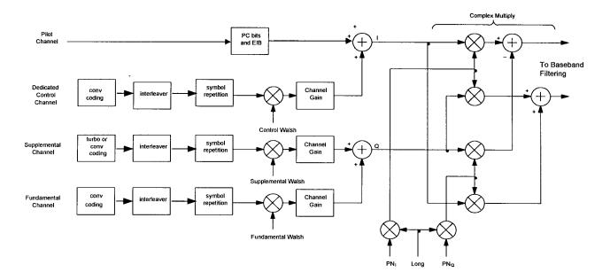
FIGURE 36.11: Reverse link channel structure in cdma2000.
