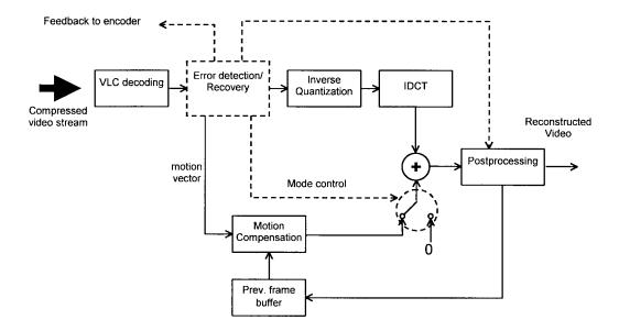
FIGURE 31.4: Error resilient video decoder.
