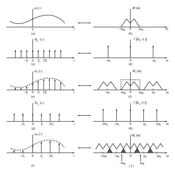
FIGURE 2.1: Illustration of instantaneous sampling and sampling theorem.
