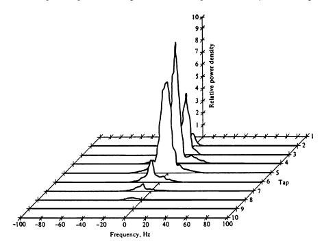
FIGURE 5.4: Scattering function of a medium-range tropospheric scatter channel.
