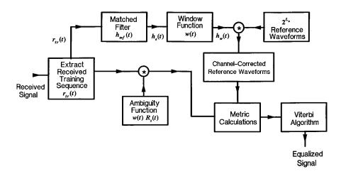
FIGURE 18.15: The Viterbi equalizer as applied to GSM.
