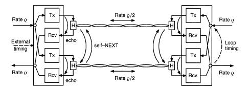
FIGURE 7.3: Model of a dual-duplex transmission system.
