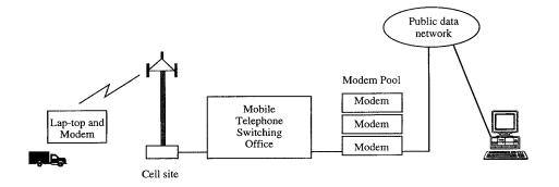
FIGURE 33.2: Cellular data service supported by modem pools in the network.
