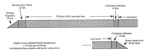
FIGURE 33.8: Cellular digital packet data reverse link block structure.
