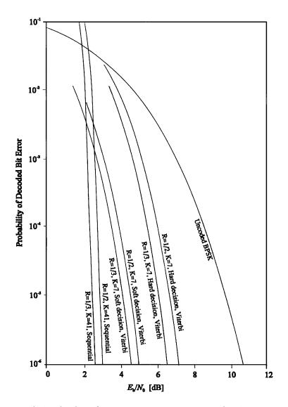
FIGURE 10.5: Convolutional code performance. *Source:* Omura, J.K. and Levitt, B.K., © 1982 IEEE, "Coded Error Probability Evaluation for Antijam Communication Systems," *IEEE Trans. Commun.*, vol. COM-30, no. 5, pp. 896–903. Reprinted by permission of IEEE.
