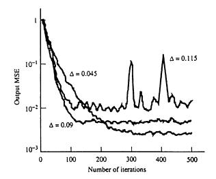
FIGURE 5.14: Initial convergence characteristics of the LMS algorithm with different step sizes.
