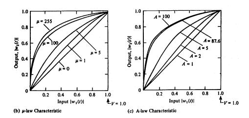
FIGURE 3.3: Compression characteristics (first quadrant shown). *Source:* Couch, L.W. II 1997. *Digital and Analog Communication Systems*, 5th ed., Prentice Hall, Upper Saddle River, NJ, p. 147. With permission.
