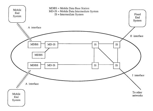
FIGURE 33.6: Cellular digital packet data network architecture.
