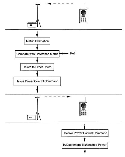
Figure 25.2a Reverse link closed-loop power control.
