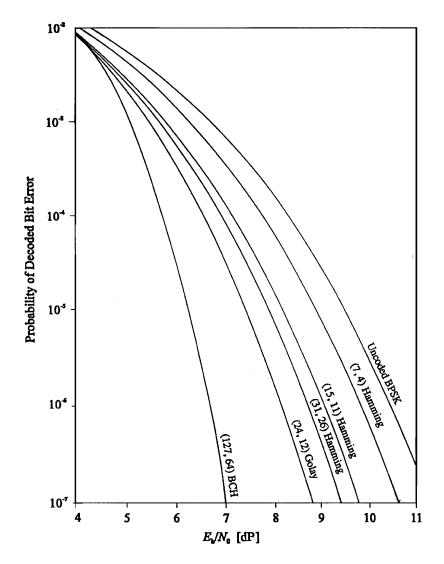
FIGURE 10.3: Block code performance. *Source:* Sklar, B., 1988, *Digital Communications: Fundamentals and Applications*, © 1988, p. 300. Reprinted by permission of Prentice-Hall, Inc., Englewood Cliffs, NJ.
