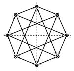
FIGURE 28.1: Constellation for  $\pi/4$  shifted QPSK modulation. *Source*: TIA, 1992. Cellular System Dual-mode Mobile Station–Base Station Compatibility Standard TIA/EIA IS-54. With permission.
