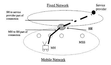
FIGURE 32.6: Proposed architecture for wireless networks.
