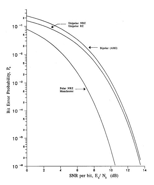
FIGURE 6.3: Bit error probability for different line codes.
