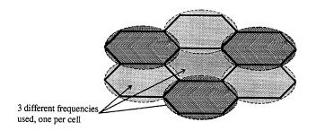
FIGURE 32.3: Cellular structure for wireless LANs (note frequency reuse).
