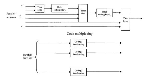
FIGURE 36.3: Time and code multiplexing principles.
