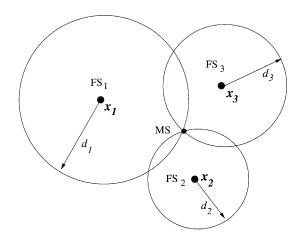
FIGURE 24.2: For signal strength and ToA based radiolocation systems the location of the MS is at the intersection of circles of radius  $d_i$ .
