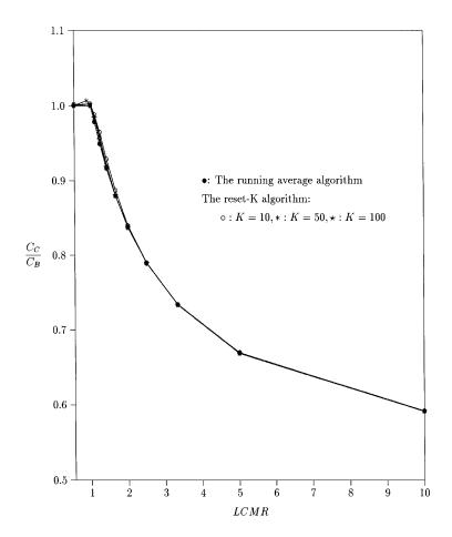
FIGURE 20.9: The location tracking costs for the running average algorithm and the reset-*K* algorithm;  $C_H = 0.5C_B$ .
