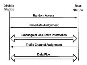
FIGURE 17.3: Mobile-originating call establishment.
