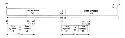
FIGURE 36.14: Burst structure.
