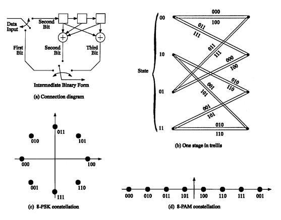
FIGURE 10.6: Rate 2/3 trellis-coded modulation.
