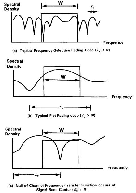
FIGURE 18.8: Relationships between the channel frequency-transfer function and a signal with bandwidth W.
