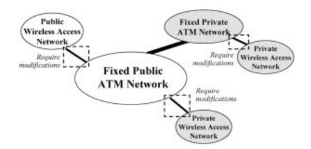
FIGURE 34.1: Wireless ATM interworking architecture.
