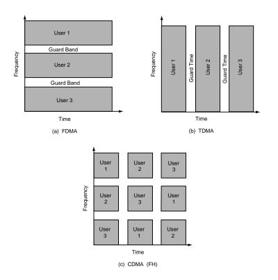
FIGURE 17.1: Multiple-access methods for wireless communication systems.
