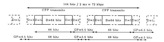
FIGURE 29.1: M1 burst and TDD frame structure.
