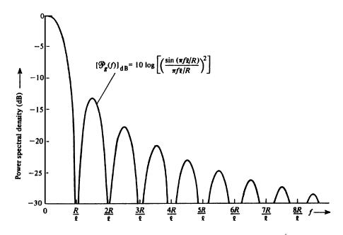
FIGURE 1.6: PSD for the complex envelope of MPSK and QAM where  $M = 2^{\ell}$  and R is bit rate (positive frequencies shown). *Source:* Couch, L.W., II. 1997. *Digital and Analog Communication Systems*, 5th ed., Prentice Hall, Upper Saddle River, NJ, p. 350. With permission.
