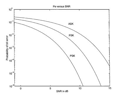
FIGURE 9.4:  $P_e$  vs. the signal to noise ratio in decibels  $[dB = 10 \log(E/N_0)]$  for amplitudeshift keying, frequency-shift keying, and phase-shift keying; note that there is a 3-dB difference in performance from ASK to FSK to PSK.
