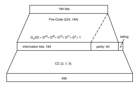
FIGURE 27.4: FEC in SACCH, FACCH, BCCH, SDCCH, PCH and AGCH, ©ETT [4].
