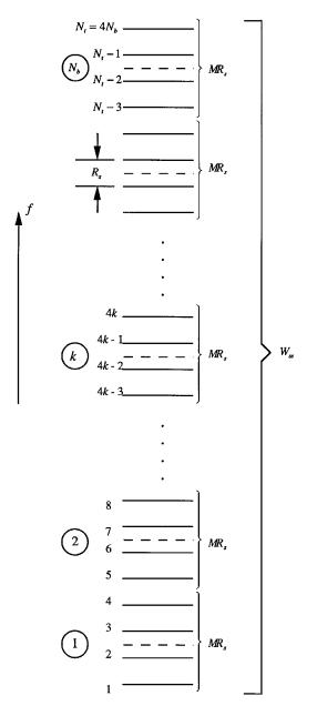
**Figure 11.3a** Frequency distribution for FH-4FSK—nonoverlapping bands. Dashed lines indicate location of hop frequencies.
