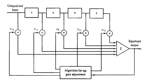
FIGURE 5.10: Linear transversal filter.
