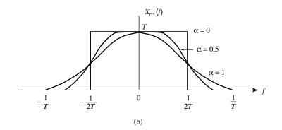
FIGURE 5.9: Pulses having a raised cosine spectrum.
