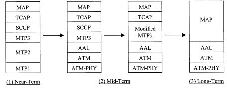
TCAP – Transaction Capabilities Application Part SCCP – Signaling Connection Control Part
