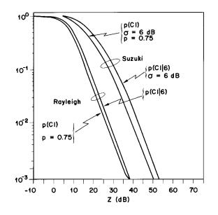
FIGURE 21.2: Conditional and unconditional outage probability for n = 6 interferes in a Rayleigh environment and in a Suzuki environment with  $\sigma = 6$  dB.
