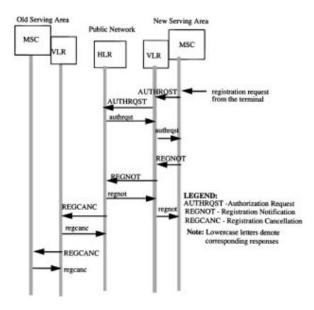
FIGURE 20.3: Signalling flow diagram for registration in IS-41.
