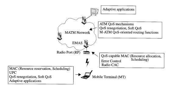
FIGURE 35.2: QoS mechanisms in wireless ATM.
