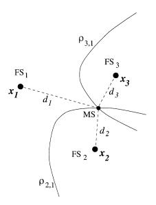
FIGURE 24.3: For TDoA based radiolocation the position of the MS is at the intersection of hyperbolas. The curves represent constant differences in distance to the MS with respect to the first FS,  $\rho_{i,1} = d_i - d_1$ .
