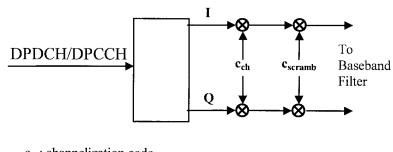
c<sub>ch</sub>: channelization code c<sub>scramb</sub>: scrambling code
