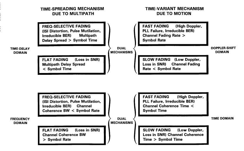
FIGURE 18.6: Small-scale fading: mechanisms, degradation categories, and effects.
