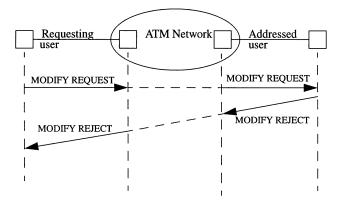
FIGURE 35.13: Addressed user rejection of modification.
