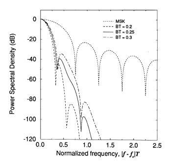
FIGURE 16.8: Power density spectrum of MSK and GMSK.
