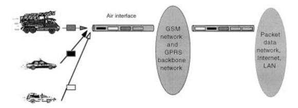
FIGURE 26.3: Simplified view of the GPRS architecture.
