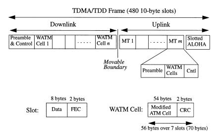
FIGURE 35.3: TDMA logical frame format.
