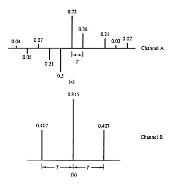
FIGURE 5.16: Two channels with ISI.
