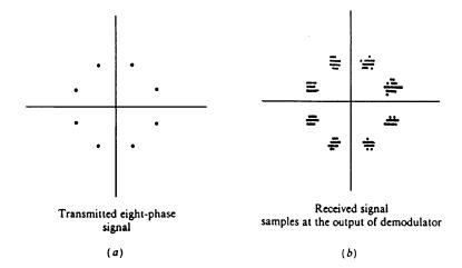
FIGURE 5.8: Two-dimensional digital eye patterns.
