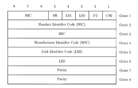
FIGURE 29.5: Fixed format packets mapped on M1, M2, and M3 during link initialization and on M1 and M2 during handshake.
