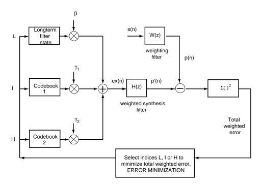
FIGURE 28.3: Black diagram of the speech encoder in VSELP. TIA. 1992. Cellular system Dual-mode Mobile Station–Base Station Compatibility Standard. TIA/EIA IS-54.
