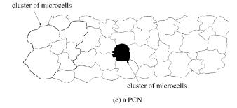
FIGURE 22.6: Microcellular clusters with oversailing macrocellular clusters. Each macrocell is associated with a particular microcellular cluster. *Source*: Steele and Williams. 1993. Third generation PCN and the intelligent multimode mobile portable. *IEE Elect. and Comm. Eng. J.*, 5(3), 147–156. With permission.
