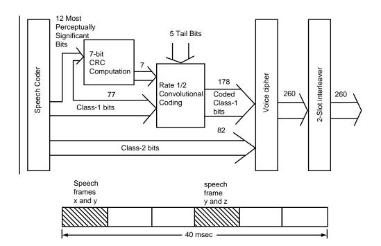
FIGURE 28.5: Error correction insertion for speech coder. Source TIA, 1992. Cellular Systems Dual-Mode Mobile Station–Base Station Compatibility Standards. TIA/EIA IS-54. With permission.
