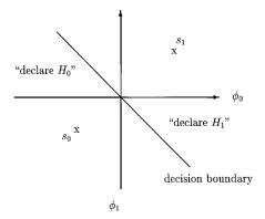
FIGURE 9.3: Signal space and decision boundary for optimal binary receiver.
