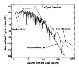
FIGURE 22.3: Signal level profiles for the two- and four-path models. Also shown are the free space and inverse fourth power laws. *Source*: Green. 1990. Radio link design for microcellular system, *British Telecom. Tech. J.*, 8(1), 85–96. With permission.
