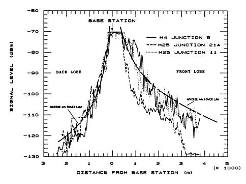
FIGURE 22.2: Overlayed received signal strength profiles of various highway cells including the inverse fourth power law curve for both the front and back antenna lobes. *Source:* Chia et al. 1987. Propagation and bit error ratio measurements for a microcellular system. *JIERE*. 57(6), 5255–5266. With permission.
