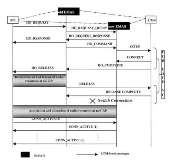
FIGURE 35.23: Backward handover control flow.
