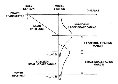
FIGURE 18.2: Link-budget considerations for a fading channel.
