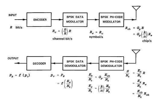
FIGURE 13.4: Direct-sequence spread-spectrum MODEM with channel coding.
