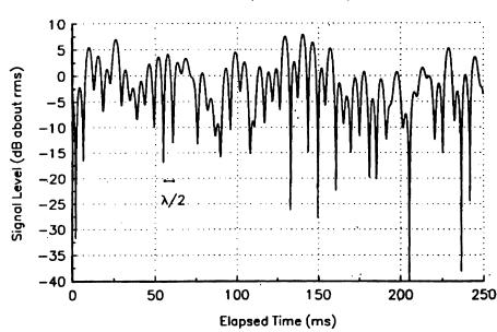
Typical simulated Rayleigh fading at the carrier Receiver speed = 1 20 km/hr
