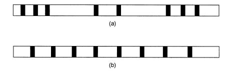
FIGURE 31.7: Position of resynchronization markers in the bitstream for (a) H.263 (Version 1) encoder with GOB headers and for (b) an MPEG-4 encoder with video packets.
