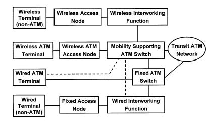
FIGURE 34.2: Wireless and wireline system integration with transit ATM Network.
