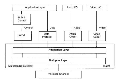
FIGURE 31.2: Configuration of a wireless multimedia terminal.
