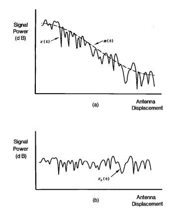
FIGURE 18.3: Large-scale fading and small-scale fading.
