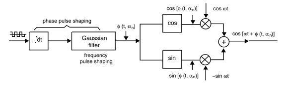
FIGURE 27.8: GMSK modulator schematic diagram, <sup>(C)</sup>ETT [4].
