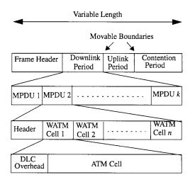
FIGURE 35.6: Magic WAND TDMA frame structure.
