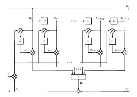
FIGURE 7.5: Block diagram of an adaptive transversal filter echo canceller.
