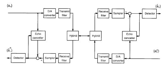
FIGURE 7.1: Model of a full-duplex PAM transmission system.
