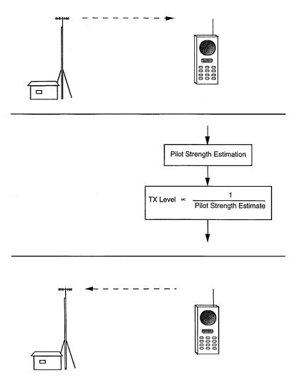
FIGURE 25.1: Reverse link open-loop power control.
