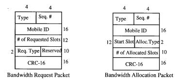
FIGURE 35.4: Bandwidth control packet formats.
