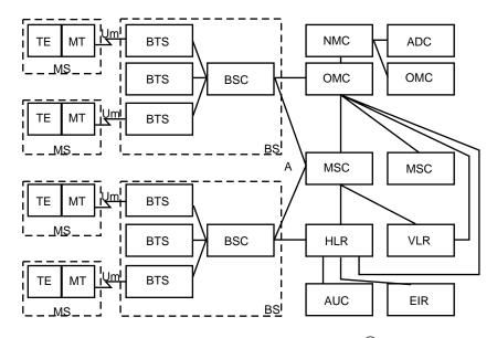
FIGURE 27.1: Simplified structure of GSM PLMN <sup>©</sup> ETT [4].
