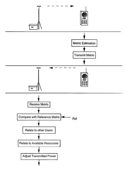
Figure 25.2b Forward link closed-loop power control.
