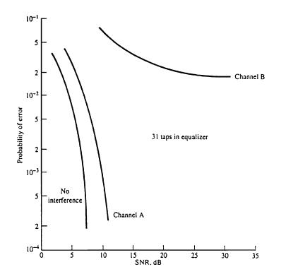
FIGURE 5.18: Error-rate performance of linear MSE equalizer.
