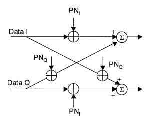
FIGURE 36.4: Complex spreading.
