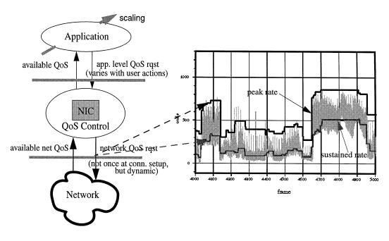
FIGURE 35.9: System and API model for QoS control with bandwidth renegotiation.
