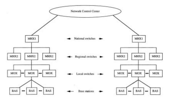
FIGURE 33.4: MOBITEX network architecture.
