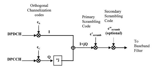
FIGURE 36.8: Reverse link spreading for the DPDCH and DPCCH.
