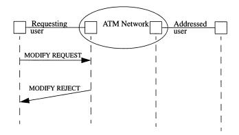
FIGURE 35.14: Network rejection of modification request.
