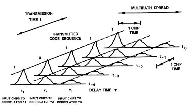
FIGURE 18.16: Example of received chips seen by a 3-finger rake receiver.
