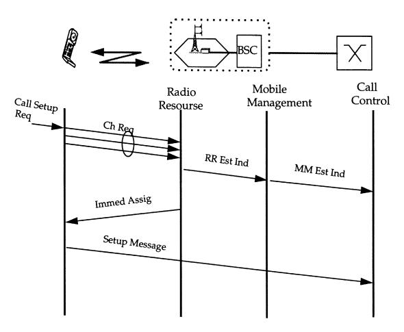
FIGURE 23.2: Radio resource assignment in GSM/DCS. *Source*: Jabbari, B., et al., Network issues for wireless personal communications. *IEEE Commun. Mag.*, 33(1), 1995.
