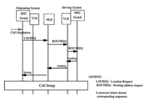
FIGURE 20.4: Signalling flow diagram for call delivery in IS-41.
