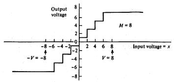
(a) Quantizer Output-Input Characteristics
