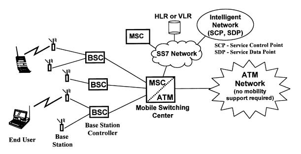
FIGURE 34.4: A near-term architecture for PCS-to-ATM interworking.
