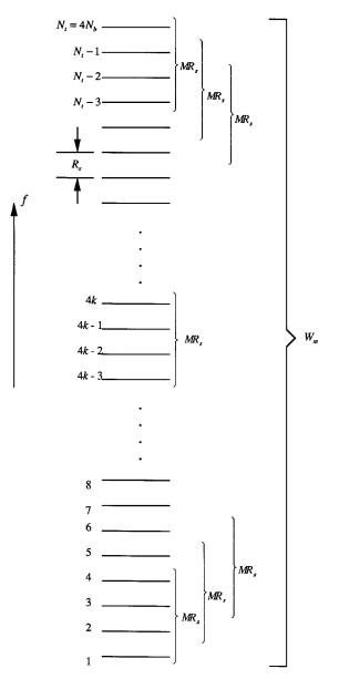
Figure 11.3b Frequency distribution for FH-4FSK—over-lapping bands.
