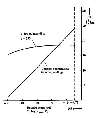
FIGURE 3.4: Output *S*/*N* of 8-b PCM systems with and without companding. *Source:* Couch, L.W. II 1997. *Digital and Analog Communication Systems*, 5th ed., Prentice Hall, Upper Saddle River, NJ, p. 149. With permission.
