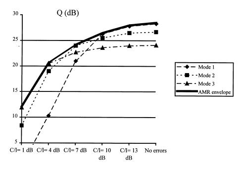
FIGURE 26.1: AMR codec quality as a function of C/I. (Typical results derived from the first AMR selection tests. Quality is given on the equivalent MNRU scale in dB).
