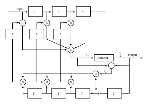
FIGURE 5.15: An adaptive zero-forcing equalizer.
