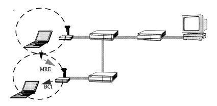
FIGURE 35.16: Handover procedure with soft-QoS in the WATMnet system.
