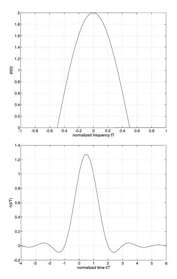
FIGURE 4.9: Duobinary frequency response and minimum bandwidth pulse.
