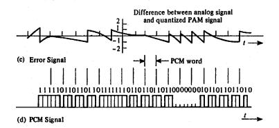
FIGURE 3.2: Illustration of waveforms in a PCM system. *Source:* Couch, L.W. II 1997. *Digital and Analog Communication Systems*, 5th ed., Prentice Hall, Upper Saddle River, NJ, p. 139. With permission.
