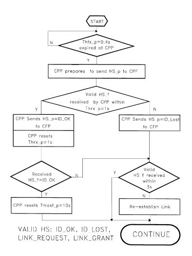
FIGURE 29.9: CT-2 handshake algorithms.
