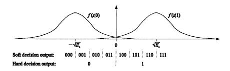
FIGURE 10.2: Hard and soft decision demodulation of a coherently demodulated BPSK signal corrupted by AWGN.  $f(z \mid 1)$  and  $f(z \mid 0)$  are the Gaussianly distributed conditional probability density functions at the threshold device.
