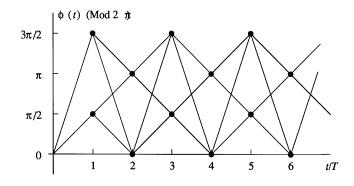
FIGURE 16.5: Phase-trellis diagram for MSK.
