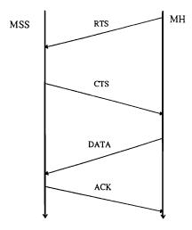
FIGURE 32.5: CSMA/CA and four-way handshaking protocol.
