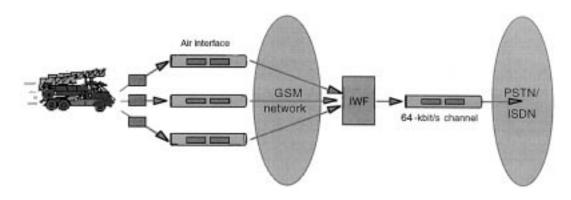
FIGURE 26.2: Simplified GSM network configuration for HSCSD.
