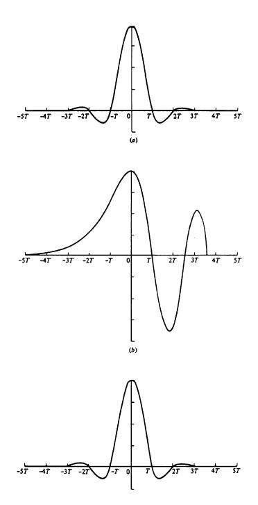
FIGURE 5.1: Effect of channel distortion: (a) channel input, (b) channel output, (c) equalizer output.
