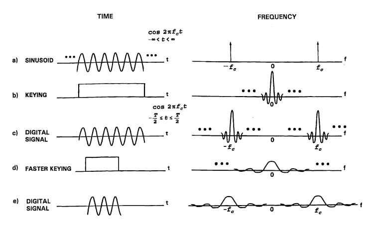
FIGURE 18.11: Analogy between spectral broadening in fading and spectral broadening in keying a digital signal.
