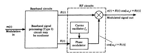
FIGURE 1.2: Generalized transmitter using the AM-PM generation technique. *Source:* Couch, L.W., II. 1997. *Digital and Analog Communication Systems*, 5th ed., Prentice Hall, Upper Saddle River, NJ, p. 278. With permission.
