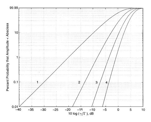
FIGURE 12.4: Probability distribution for signal envelope for maximal ratio combining.
