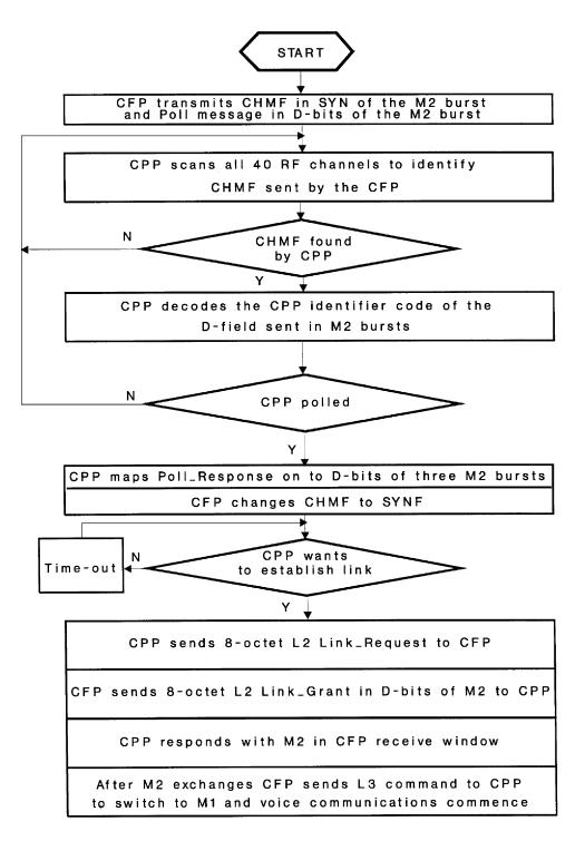
FIGURE 29.7: Flowchart of the CT-2 link initialization by the CFP.
