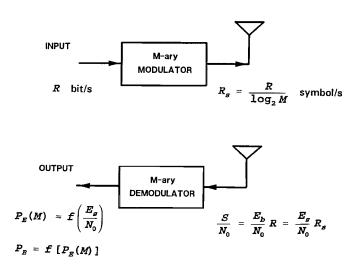
FIGURE 13.2: Basic modulator/demodulator (MODEM) without channel coding.
