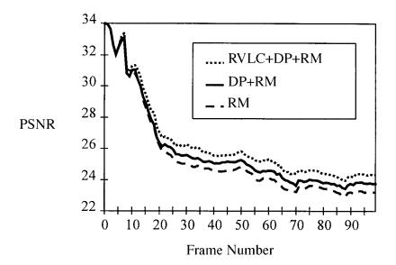
FIGURE 31.11: Performance comparison of resynchronization, data partitioning, and RVLC over a bursty channel simulated by a 2-state Gilbert model. Burst durations are 1ms long and the probability of occurrence of a burst is  $10^{-2}$ . Legend: RM—resynchronization marker; DP—data partitioning; RVLC—reversible variable length codes.
