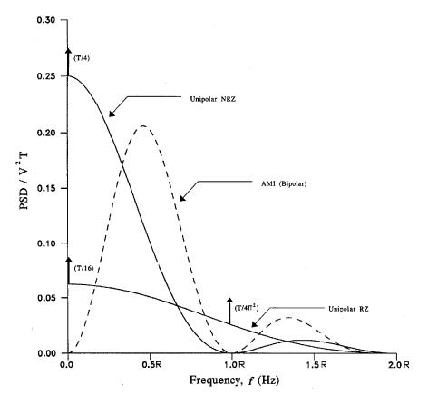
**Figure 6.2a** Power spectral density of different line codes, where R = 1/T is the bit rate.
