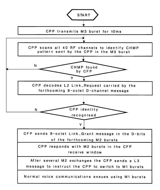
FIGURE 29.6: Flowchart of the CT-2 link initialization by the CPP.
