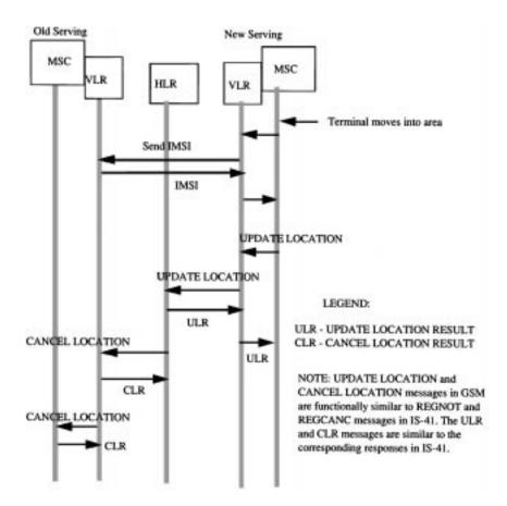
FIGURE 20.5: Flow diagram for registration in GSM.
