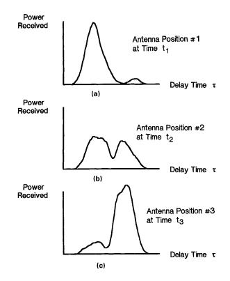
FIGURE 18.5: Response of a multipath channel to a narrow pulse vs. delay, as a function of antenna position.
