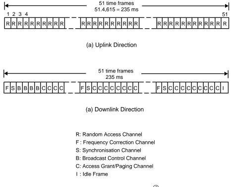
FIGURE 27.5: The control multiframe, <sup>©</sup>ETT [4].
