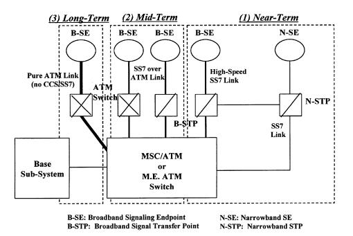
Note: A signaling endpoint is the mobility control at a mobile switch, server or database.
