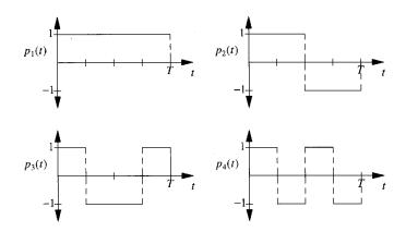
FIGURE 4.2: Four orthogonal spread-spectrum pulse shapes.
