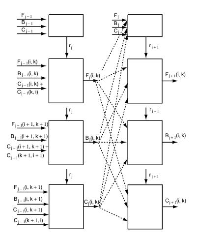
FIGURE 28.4: Block diagram for lattice covariance computations.
