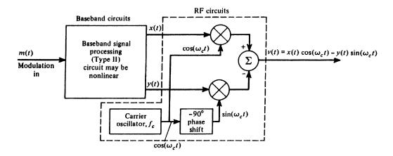
FIGURE 1.3: Generalized transmitter using the quadrature generation technique. *Source:* Couch, L.W., II. 1997. *Digital and Analog Communication Systems*, 5th ed., Prentice Hall, Upper Saddle River, NJ, p. 278. With permission.
