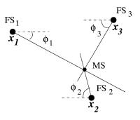
FIGURE 24.1: The measured angles,  $\phi_i$ , determine the position of the MS for a given FS geometry.
