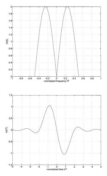
FIGURE 4.10: Modified duobinary frequency response and minimum bandwidth pulse.
