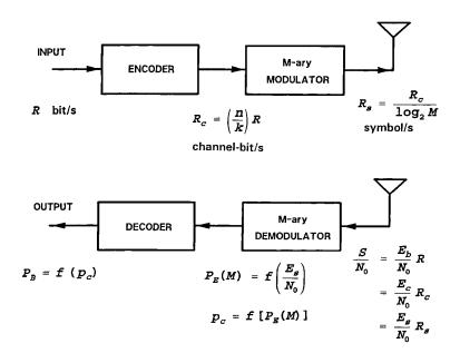
FIGURE 13.3: MODEM with channel coding.
