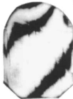
interferograms of thin aluminum mirror (both interferograms are of same mirror)
