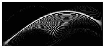
**Fig. 10.13.** An example of the presence of cross-terms in the WVD. The original signal is a chirp, first rising in frequency and then falling. High-energy coefficients appear beneath the main arc of energy in the transform plane, yet the time-domain signal contains no such tones. Higher-level interpretation routines are beset with the problem of separating such artifacts from genuine features of the signal's time evolution.
