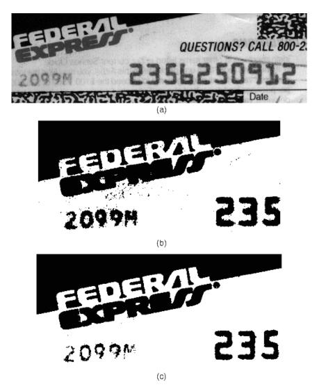
**Fig. 2.9.** Thresholding. An 8-bit, 256 gray scales image of a shipping label (a). First threshold applied (b). Here the threshold results in an image that is too dark. The company logo is only marginally readable. With a different threshold (c), the logo improves, but the shipping code beneath begins to erode. It is difficult to pick an appropriate global threshold for the image.
