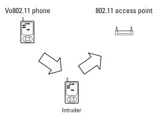
Figure 7.8 Replay attack on a network.
