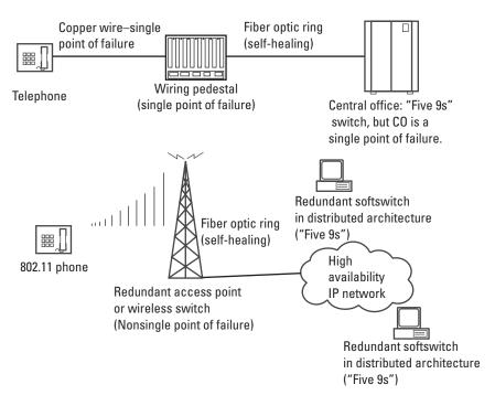
Figure 11.1 Properly engineered, wireless VoIP networks can be more reliable than the PSTN.
