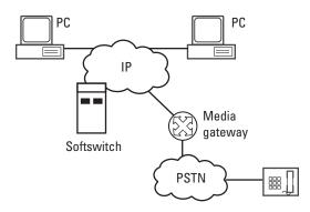
Figure 4.5 PC-to-PC and PC-to-phone applications.
