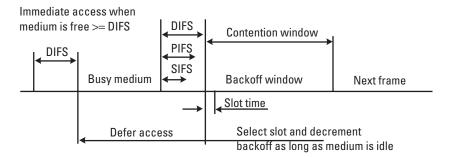
Figure 8.4 Basic access method in DCF and PCF. (*From:* [12]. © 2002 Stanford University. Reprinted with permission.)
