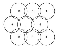
Figure 10.4 A 3-to-1 reuse pattern. (*From:* [3]. © 2002 Neeli Prasad and Anand Prasad. Reprinted with permission.)
