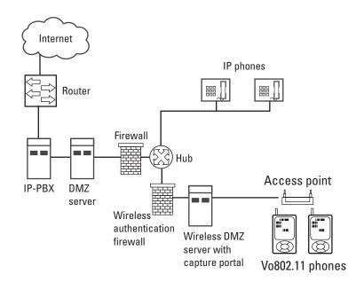
Figure 7.13 A wireless authentication firewall protects the LAN.
