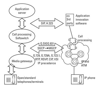
Figure 4.6 Relationship of softswitch with other components. (*From:* [7]. © 1999 Cisco Systems, Inc. Reprinted with permission.)
