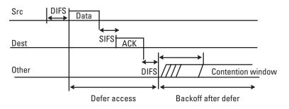
Figure 2.3 CSMA/CA back-off algorithm.
