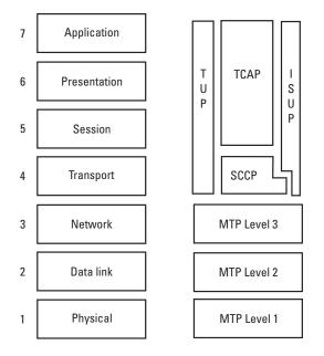
Figure 4.2 Comparison of OSI reference model and SS7 protocol stacks. (*From:* [4]. © 2003 Performance Technologies, Inc. Reprinted with permission.)
