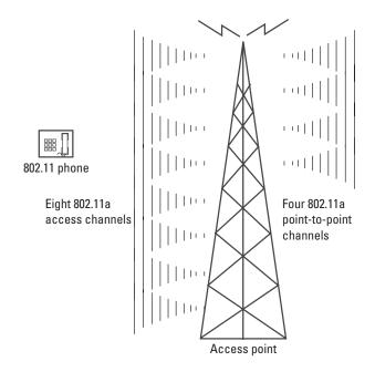
Figure 10.5 Valid 5-GHz operating channels.
