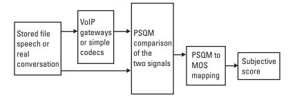
Figure 9.1 Process of PSQM. (From: [2]. © 2000 McGraw-Hill, Inc. Reprinted with permission.)
