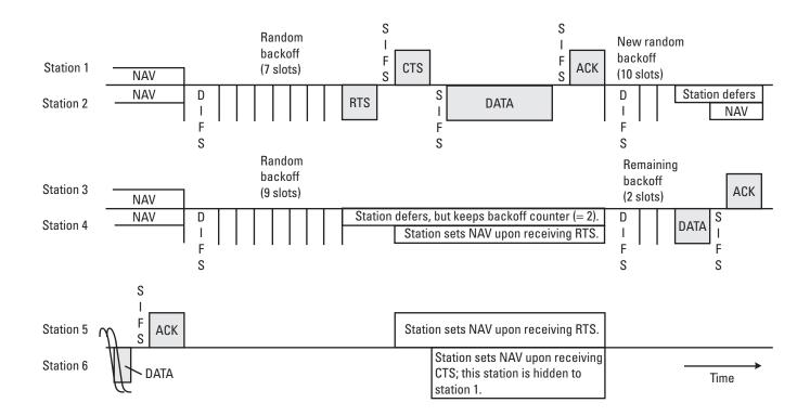
Figure 8.5 Virtual carrier sense protocol. (From: [13]. © 2002 Mustafa Ergen. Reprinted with permission.)
