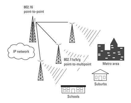
Figure 6.6 Extending the range of wireless data transmission via its architecture.
