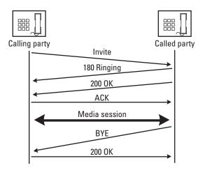
Figure 3.2 SIP UA server to UA server call. (*From:* [5]. © 2001 Artech House, Inc. Reprinted with permission.)
