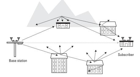
Figure 8.2 Multipath interference. (*From:* [7]. © 1999 Cisco Systems, Inc. Reprinted with permission.)
