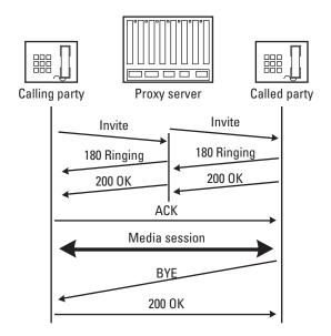
Figure 3.3 SIP call using a proxy server. (*From:* [5]. © 2001 Artech House, Inc. Reprinted with permission.)
