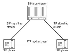
Figure 3.1 SIP is a signaling protocol and RTP transports the conversation. (*From:* [5]. © 2001 Artech House, Inc. Reprinted with permission.)
