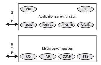
Figure 12.2 Functions of application and media servers. (*From:* [5]. © 2001 BroadSoft, Inc. Reprinted with permission.)
