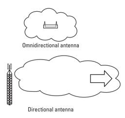
Figure 6.1 Radiated power and reach of antennas: omnidirectional and directional.
