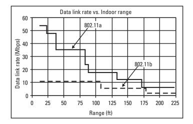
**Figure 10.2** The greater the distance from the access point, the greater the degradation in bandwidth, which limits the total number of simultaneous calls per access point. (*From:* [1]. © 2003 Trapeze Networks. Reprinted with permission.)
