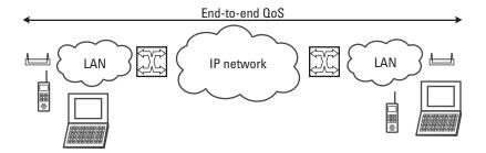
Figure 8.1 QoS is measured from endpoint to endpoint, encompassing both the wired and wireless portions of the network.
