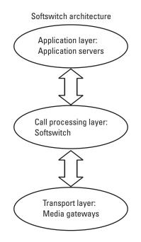
Figure 4.3 Softswitch architecture. (*From:* [4]. © 2003 Performance Technologies, Inc. Reprinted with permission.)
