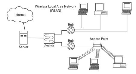
Figure 2.1 Wireless LAN on an enterprise network.
