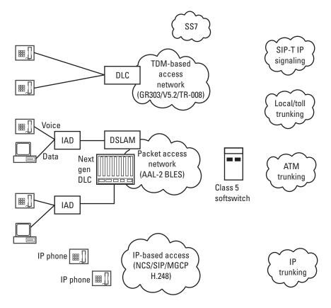
Figure 4.11 Class 5 replacement softswitch solution. (After: [14].)
