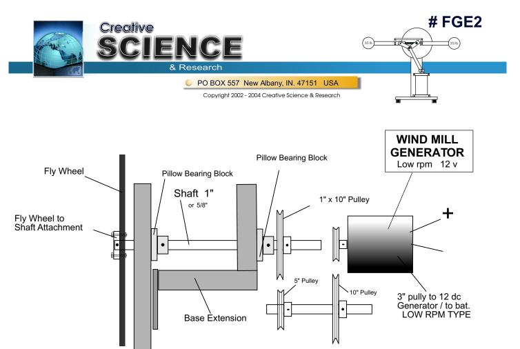
Or you can run a Low RPM Wind mill generator direct to shaft
