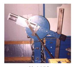
Model # 3 This was our 3rd prototype, using a machined linear slider as well as heaver weights, much higher torque!
