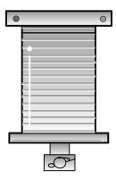
Polarity will depend on if the plunger pushes out or in. Build a small toy model first. It is best if you can build the solenoid to attract as in Figure B. Use #27 copper coated wire 66 lbs there of for larger motors and # 34 for a small toy motor, coil should weigh about 6 lbs. I do not know how many winds that is? Wind from left to right. Glue PVC bobbins with PVC glue that you can buy online or at any hardware stor. PVC sheets can be baought at any sign shop or sign supply company.
