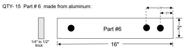
The diameter of the hole's (bore size) can be your choosing, But no less than 5/8" You can use brass bushings with bolts & nuts to separate and attach control arms.
