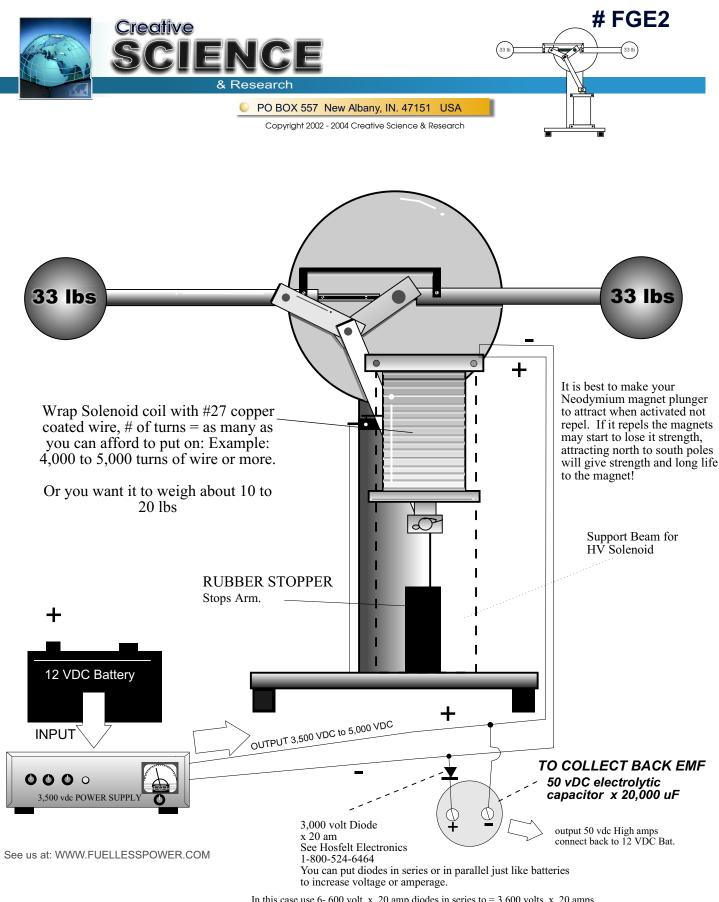
In this case use 6- 600 volt x 20 amp diodes in series to = 3,600 volts x 20 amps.
