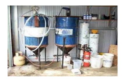
In this photo I had begun to store the 5 gallon pails in 55 gallon drums that made it easier to manage. I put a tap on the bottom so the potential bio diesel could be easily taken out.
